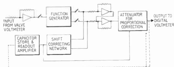
Fig. 8. Schematic diagram showing correcting circuits.
