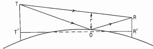
Fig. 1. The effect of a reflected wave.
