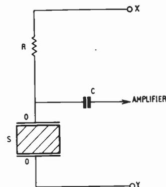
Fig. 1. Bulk conduction counter circuit. S is the semiconductor crystal, with ohmic contacts O,O. Since the counter is symmetrical the high tension collecting potential may be applied at either X or Y.
