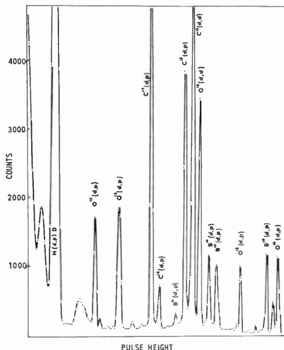
Fig. 10. A charged particle spectrum obtained in the bombardment of a thin target containing carbon, oxygen and boron with 5 MeV deuterons.
