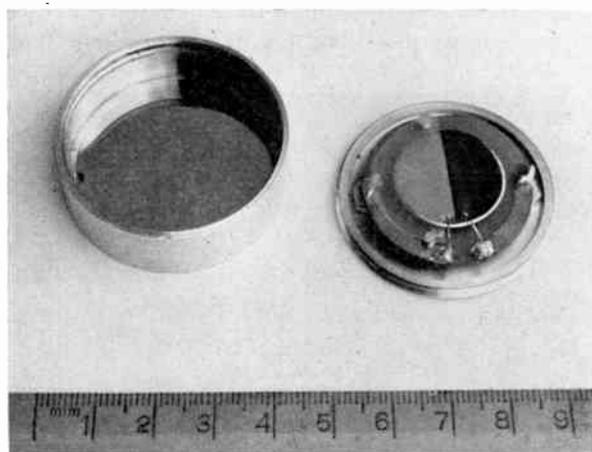
Fig. 11. Semiconductor proton-recoil fast neutron counter. Neutrons eject protons from the polyethylene which covers one of the two semi-circular counters. This counter detects the protons plus background while the other uncoated counter measures background only.
