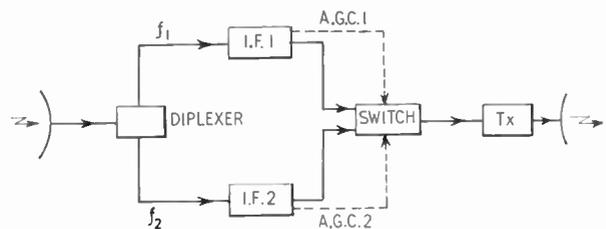
Fig. 7. Frequency diversity block schematic.
