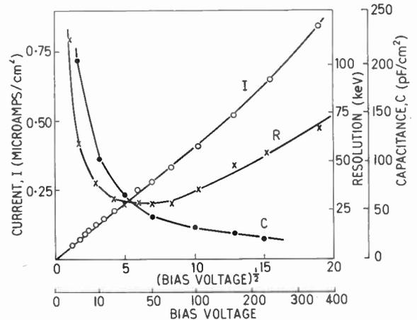
Fig. 6. Capacitance, leakage current and resolution as a function of applied bias in a typical surface-barrier detector, of area 20 mm<sup>2</sup> and of 3000 ohm cm silicon.
