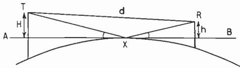
Fig. 4. Reflecting plane of interfering wave.
