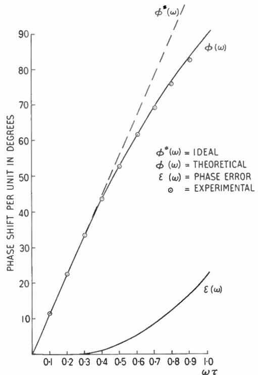
Fig. 2. Frequency phase shift characteristics.
