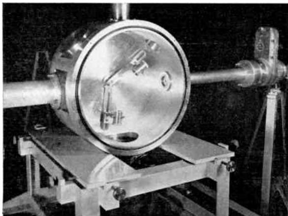
Fig. 9. A scattering chamber designed for use with semiconductor detectors. Two detectors can be set independently at any angle in a plane. The diameter of the chamber is 18 in.
