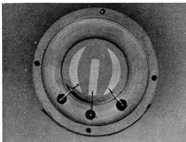
Fig. 12. A triple counter for measurements on the polarization of charged particles from nuclear reactions.
