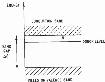
Fig. 2. Electron levels in an *n*-type semiconductor.
