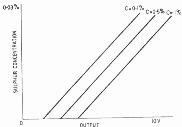
Fig. 4. Third element interference with instrument calibration.
