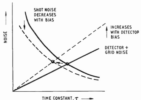
Fig. 8. Variation of noise contributions with amplifier time constants. It can be seen that the optimum time constant setting decreases with increasing detector bias.
