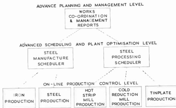
Fig. 4. Hierarchy system for integrated steel plant.
