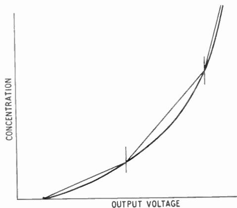
Fig. 5. Multi-segment approximation to calibration curve.
