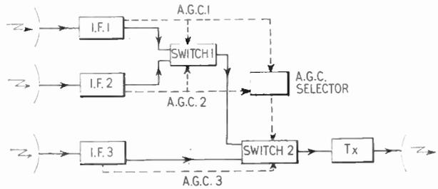
Fig. 6. Triple space diversity block schematic.
