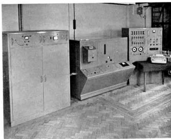
Fig. 1. The E600 direct reading spectrometer.
