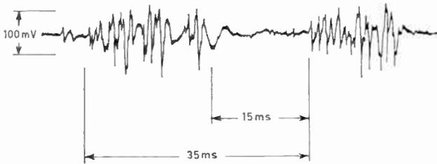
Fig. 1. Typical noise burst on a telephone circuit.
