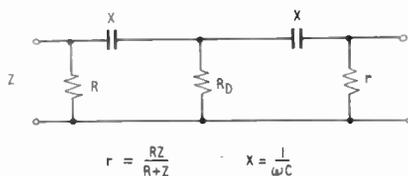
Fig. 10. Equivalent circuit non-conducting.
