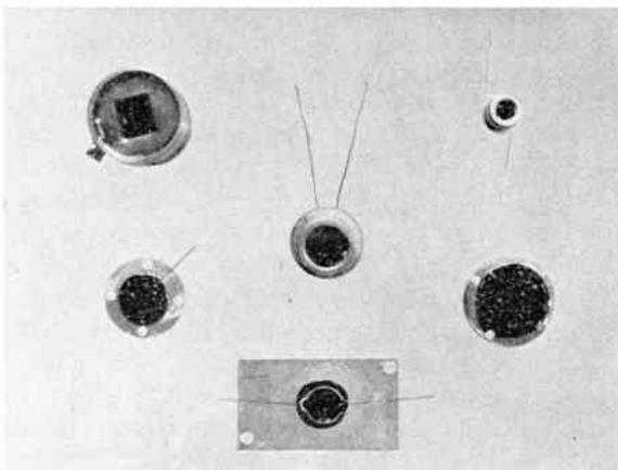
Fig. 5. Some typical semiconductor counters. Upper left—a commercial surface-barrier counter; centre and upper right—commercial diffused-junction counters, encapsulated; lower left and right—two laboratory-prepared surface-barrier counters; lower centre—a thin surface-barrier counter 0.002 in. thick for energy loss-rate measurements.
