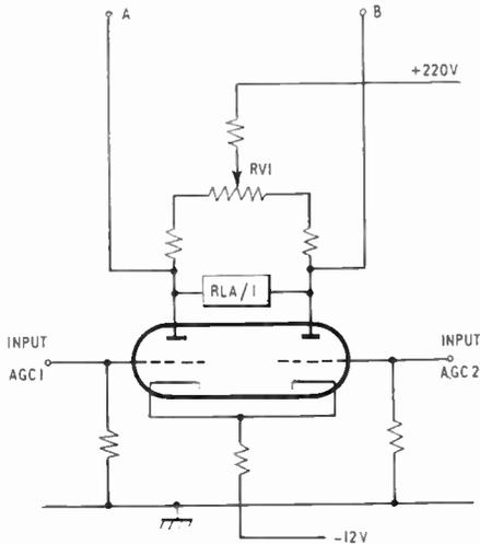
Fig. 12. Schematic of a.g.c. comparison stage.
