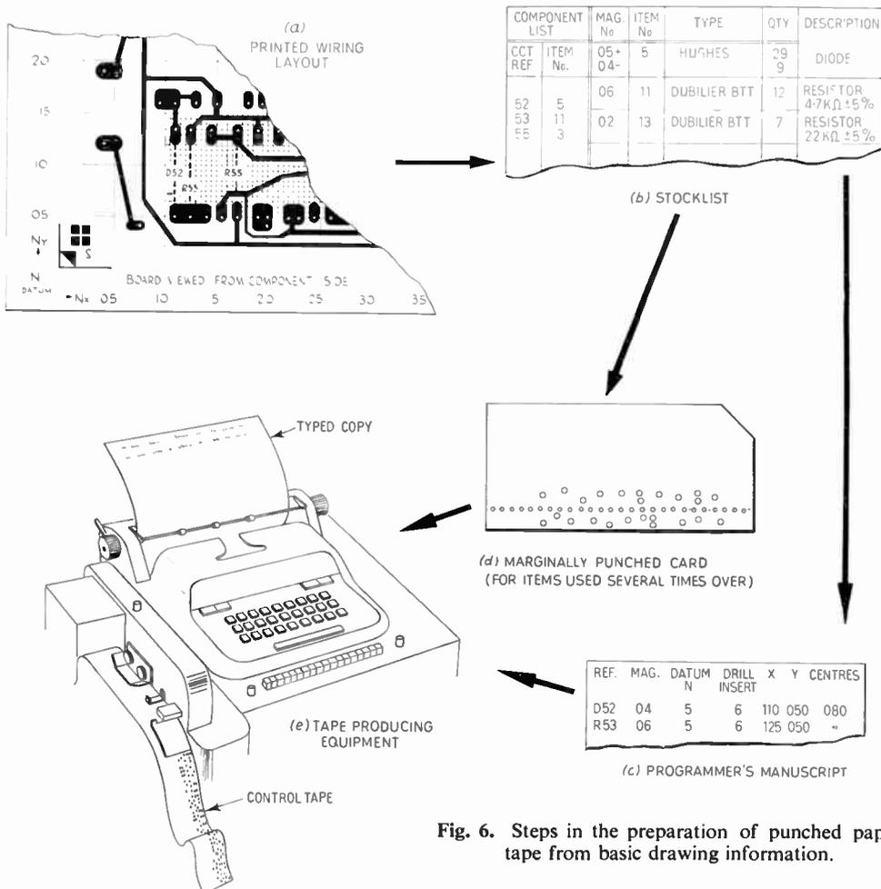
Fig. 6. Steps in the preparation of punched paper tape from basic drawing information.
