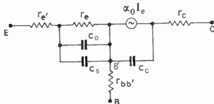
Fig. 1. Normal equivalent circuit of a p-n-p transistor in common base configuration, showing emitter diffusion capacitance, barrier-layer capacitance, the emitter diffusion-resistance, the collector barrier-layer capacitance and intrinsic base-spreading resistance  $r_{bb'}$ .
