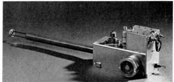
Fig. 5. Mechanical construction of the circuit of Fig. 4, showing the coaxial input, the tuned line, the variable resistor to set emitter current, the input trimmer, and the measured transistor.
