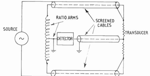
Fig. 2. Circuit to reduce ratio arm lead capacitance.
