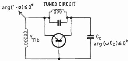
Fig. 3. Transistor in a tuned circuit with feedback to produce a negative impedance.
