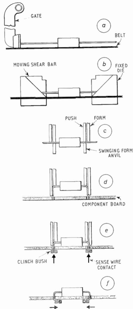
Fig. 5. Stages in component insertion.
