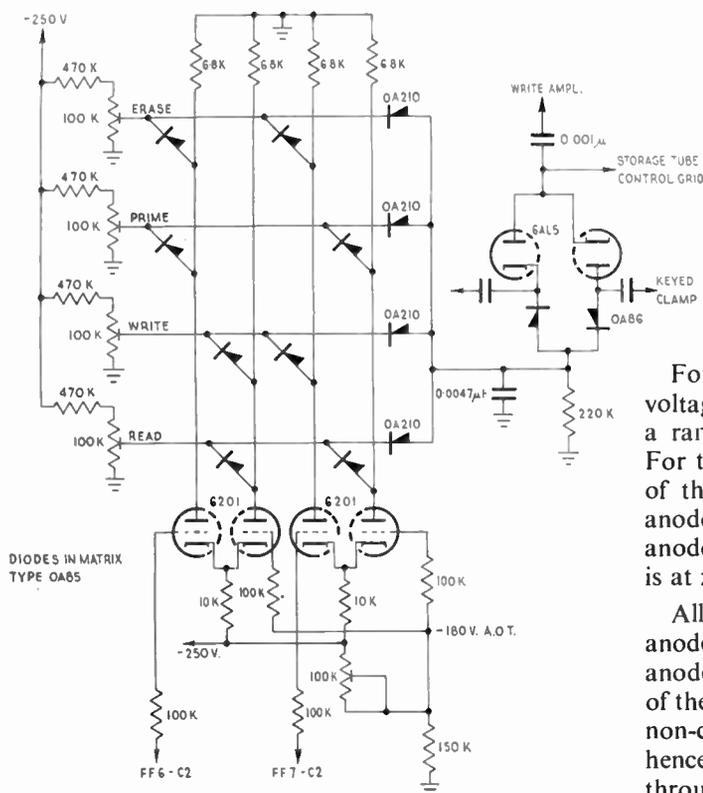
Fig. 5. Storage tube control-grid bias switching.
