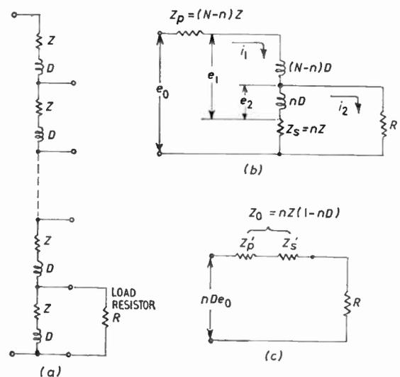
Fig. 4. Equivalent circuits for the ratio transformer.
