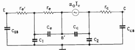
Fig. 2. Modified equivalent transistor circuit neglecting the influence of both input frequency behaviour and the intrinsic base-spreading resistance.
