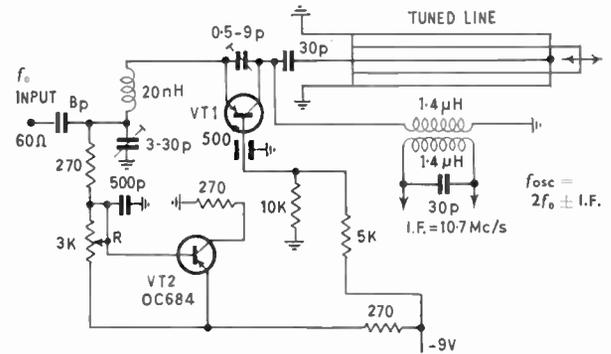
Fig. 4. Circuit of a relatively simple mixer producing high gain at low noise figures. VT1 is the transistor given in Table 1.
