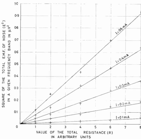
Fig. 2. Relation between noise and total resistance.
