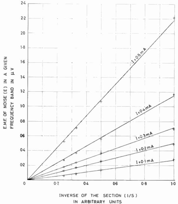
Fig. 3. Relation between noise and cross-section.
