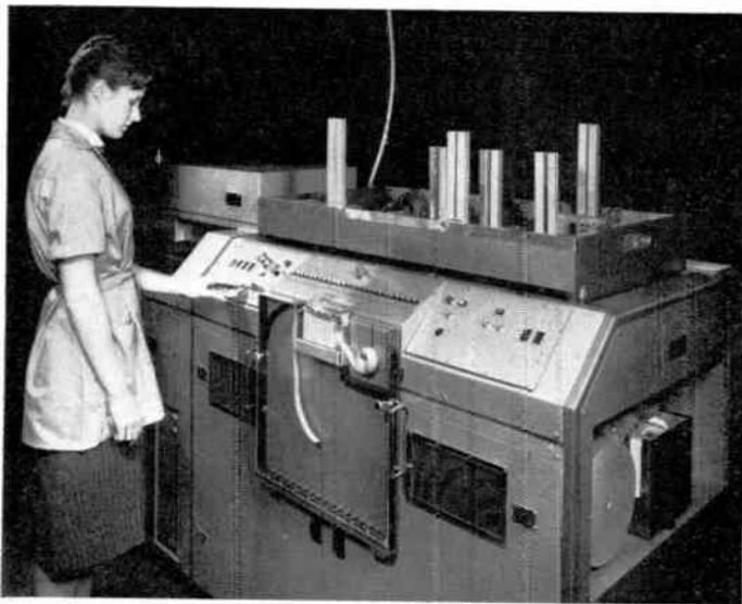
◀ The operator is here depressing the start key on her control panel. The component magazines are jacked into the store frame which can be lifted off and quickly replaced by another. The output tape reperfector is housed in a recess at the end of the machine.
