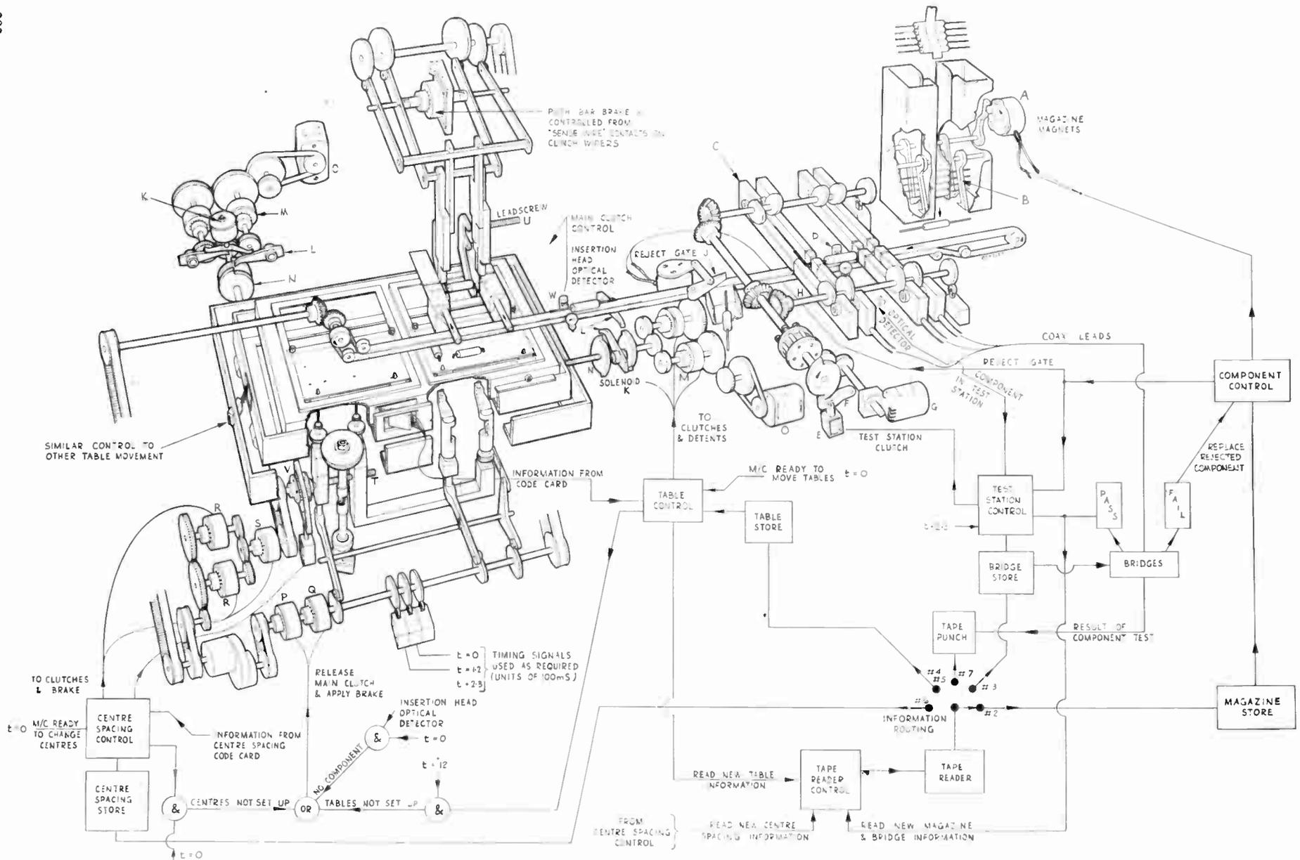
Fig. 4. Schematic diagram showing the machine elements and their connections to the control circuits.
