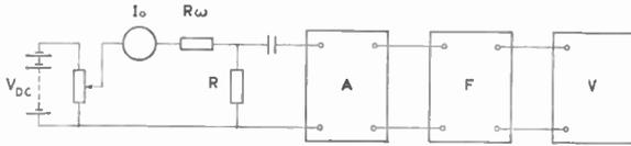
Fig. 1. Experimental arrangement for measuring current noise.
