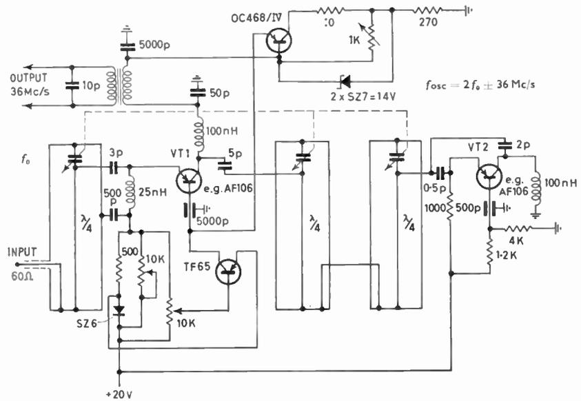
currents. Figure 8 shows the circuit of the experimental low-noise head amplifier suitable for frequencies between 400 Mc/s and 5000 Mc/s and employing normal and epitaxial transistors. Use is made of the voltage dependence of the transistor capacitance  $C_c$ . To ensure satisfactory operation of this current tuned condition and the maintenance of a sufficiently steady
