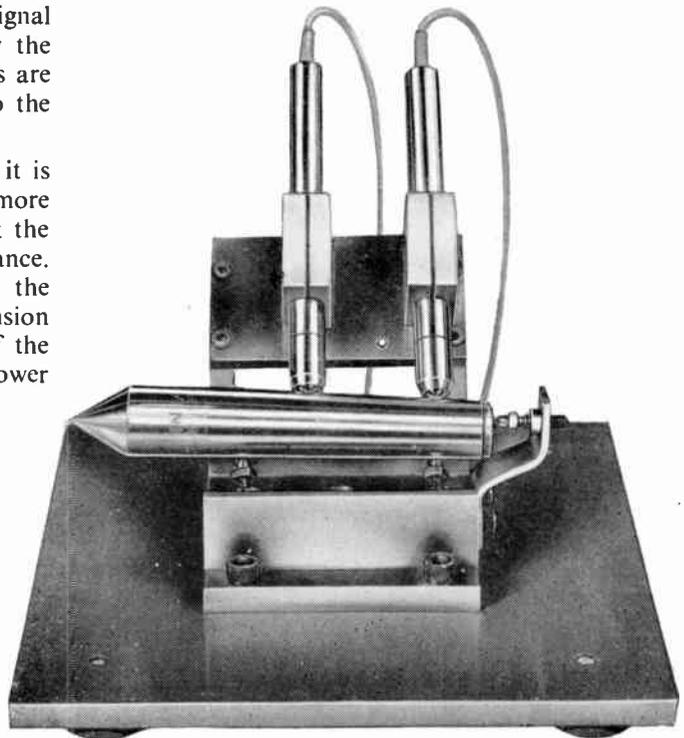
Fig. 5. Interdependent inspection example: differential gauge measuring two points on a taper roller simultaneously with interdependent logic giving taper-angle directly on scale of instrument (not shown).
