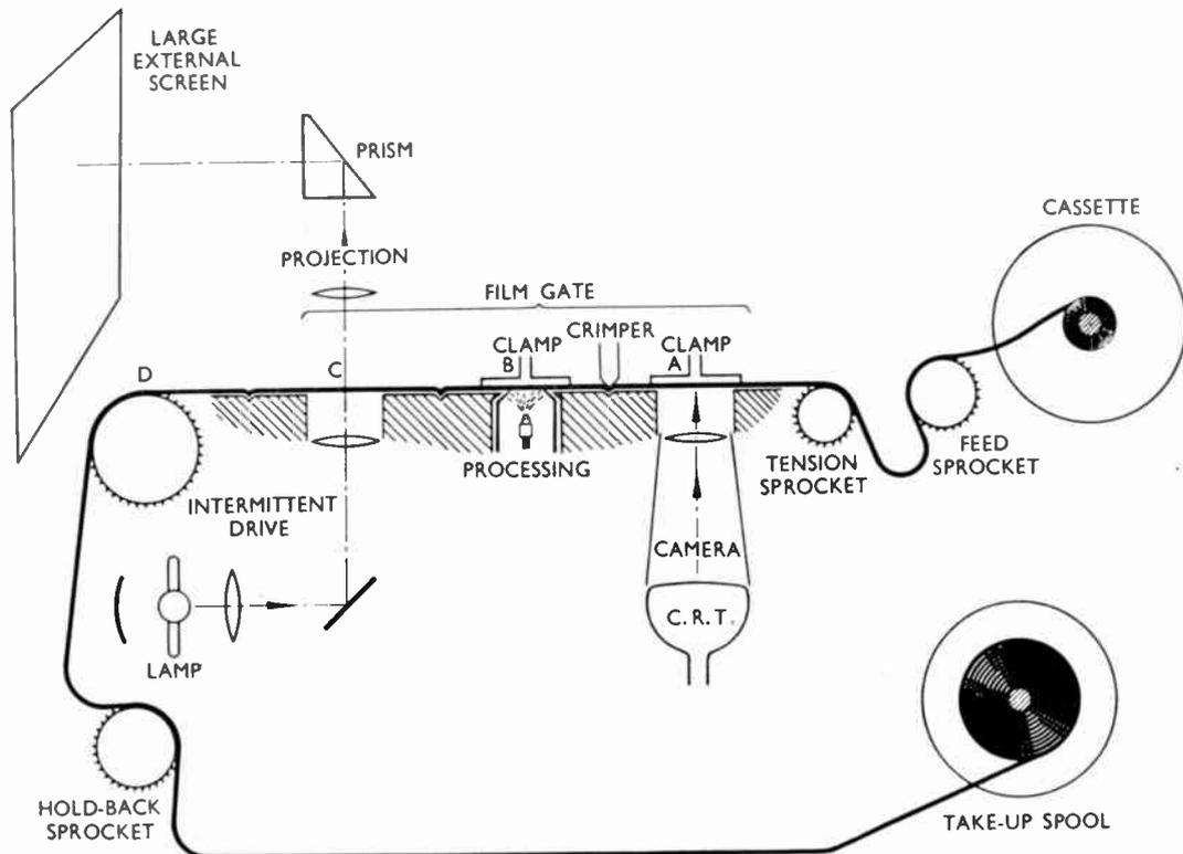
Fig. 1. Schematic representation of the 35 mm rapid photographic processor and projector.
