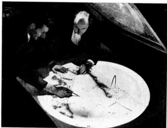
Fig. 10. A bright radar display of the Thames Estuary at Southend showing chart comparison.
