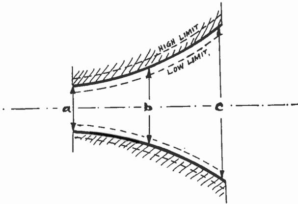
Fig. 6. Interdependent inspection example: measurements on a nozzle curvature.
