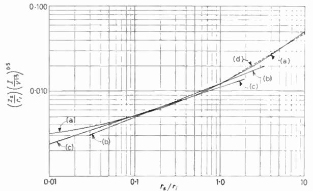
Fig. 1. The beam parameter, normalized screen distance  $\times \sqrt{\text{perveance}}$ , shown as a function of the normalized spot radius. (a) From exact solutions of the space-charge equations (1) and (2). (b) Equation (3). This is the preferred form for beam design. (c) Equation (4). (d) Equation (3) with  $r_s$  and  $r_i$  interchanged. (Equation (5).)
