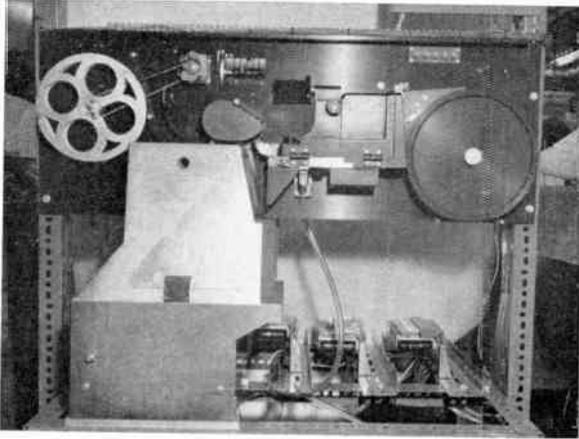
Fig. 6. The 16 mm rapid photographic processor and projector.
