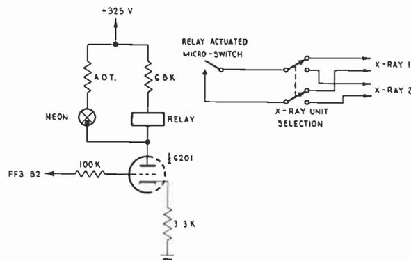
Fig. 8. X-ray unit control.
