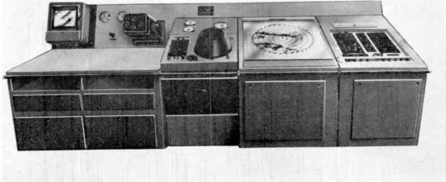
Fig. 8. The navigational console on the P & O-Orient liner S.S. *Canberra*.
