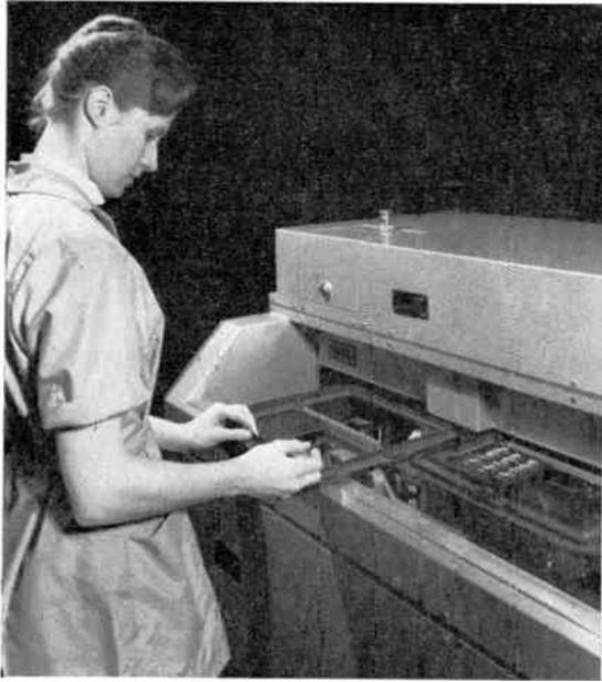
◀ The printed circuit boards are held in adjustable pallet frames. The operator is shown removing a drilled board. An assembled board can be seen in the right hand pallet.
