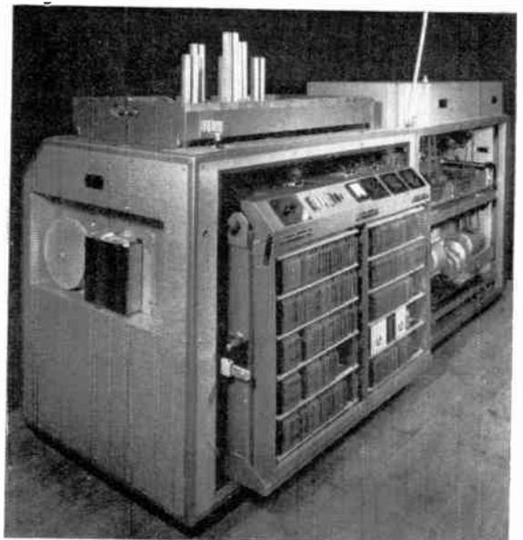
Fig. 8. The Automatic Component Assembly Machine.
