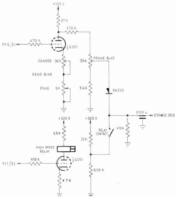
Fig. 6. Storage-grid bias switching.
