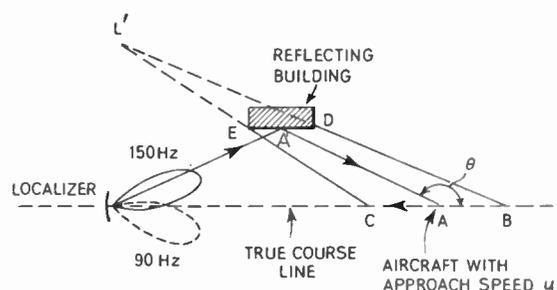
Fig. 5. Geometry of building reflection.
