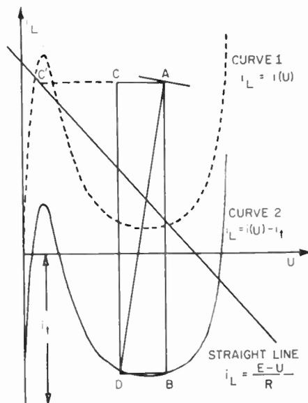
Fig. 6. Method of determining the direction of the normal to the trajectory of the operating point at any arbitrary point.
