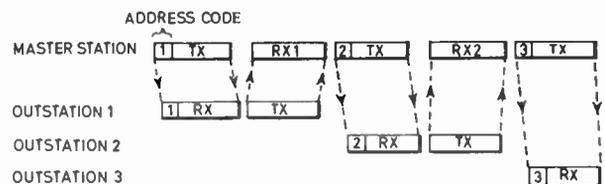
Fig. 4. Transmit/receive sequences for simplex working.
