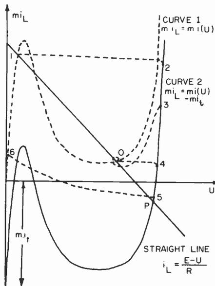
Fig. 7. Construction of the trajectory of the operating point in the (i<sub>L</sub>, U) plane.
