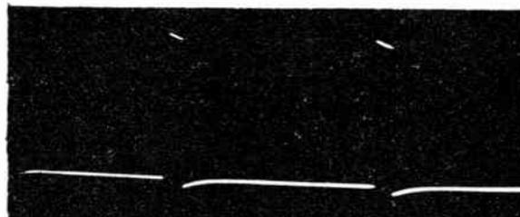
(b) Output pulse when the inductance in the circuit is a minimum.
