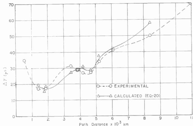
Fig. 3. Diurnal time delay  $\Delta T$  as a function of path distance.
