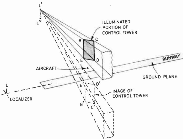
Fig. 12. Illumination restricted to upper part of control tower.
