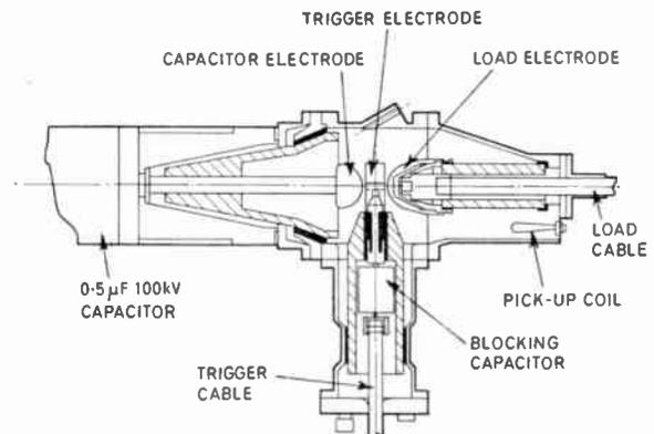
Fig. 1. Section of *Tarantula* spark-gap switch.
