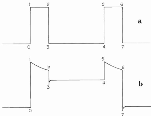
Fig. 8. (a) A pair of input rectangular positive current pulses. (b) Shape of the output pulse.
