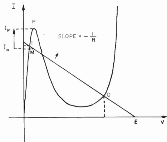
Fig. 2. Volt-ampere characteristic of the tunnel diode.
