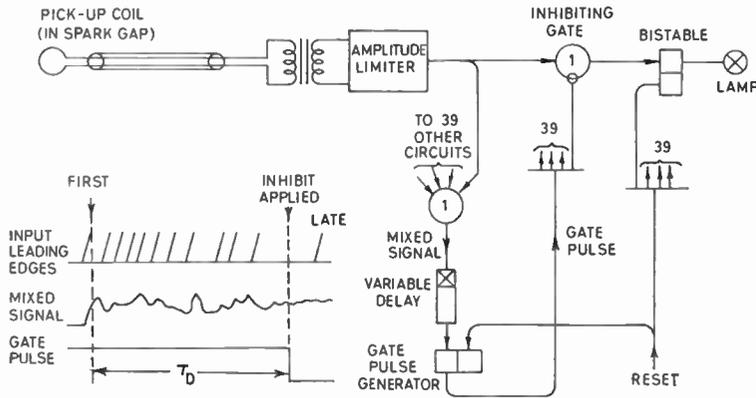
Fig. 2. Block diagram of monitor, with timing sequence.
