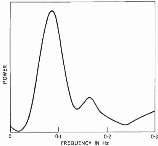
Fig. 2. Power spectrum of error current observed at mast. Overflying aircraft ground speed 130 knots, at height of 1000 ft on a course at 2° to runway.
