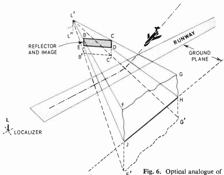
Fig. 6. Optical analogue of building reflection.
