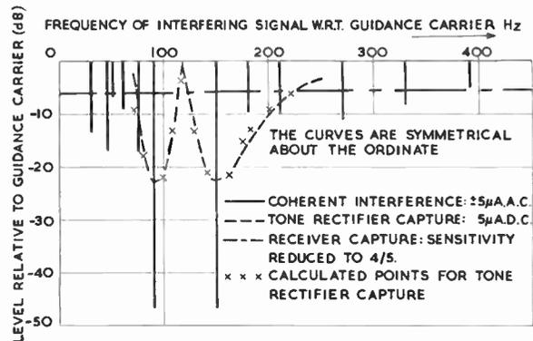
Fig. 6. V.H.F. localizer receiver interference thresholds.
