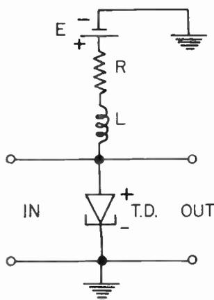
Fig. 1. Binary circuit using one tunnel diode.
