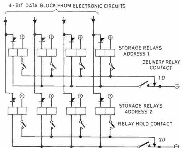
Fig. 10. Typical relay storage circuit for system having 2 addresses and 4 bits per block.
