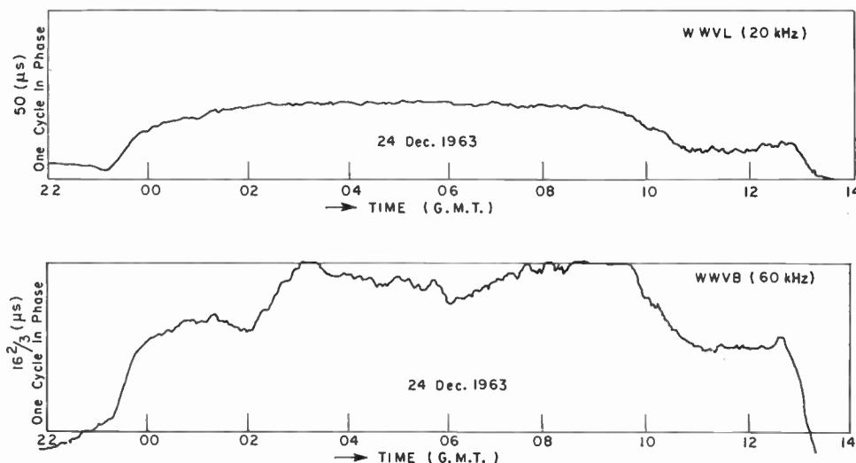
Fig. 1. Typical phase recordings of 20 and 60 kHz signals.
