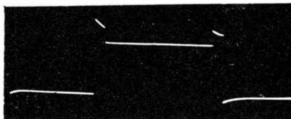
(d) Output pulse when the inductance in the circuit is a maximum.
