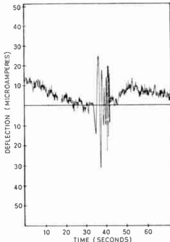
Fig. 5. Interference from overflying aircraft.
