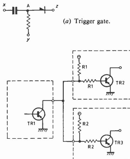
Fig. 11. Logic circuits.
