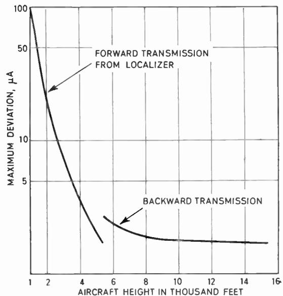
Fig. 3. Maximum deviation against height of overflying aircraft.
