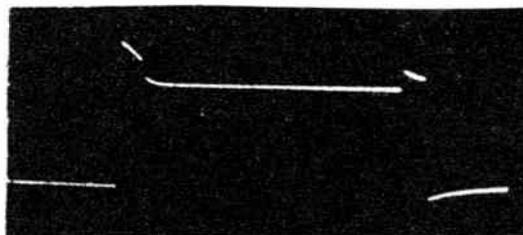
(c) Output pulse when the inductance in the circuit is of intermediate value.
