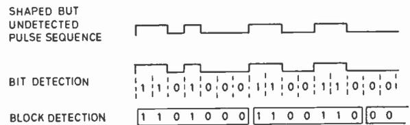
Fig. 7. Bit and block detection.
