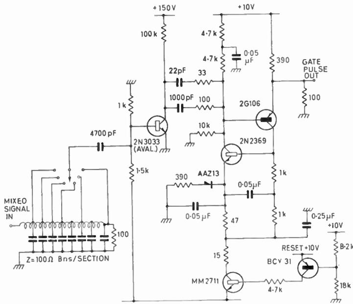
Fig. 5. Circuit of gate-pulse generator.
