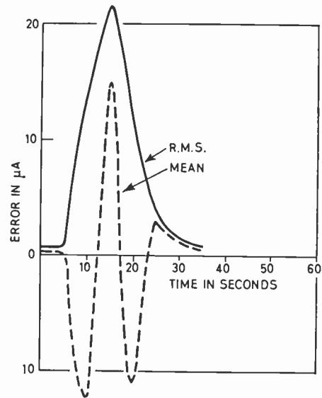
Fig. 1. Mean and r.m.s. error currents observed at mast. Overflying aircraft ground speed 130 knots, at height of 1000 ft on a course at 2° to runway.
