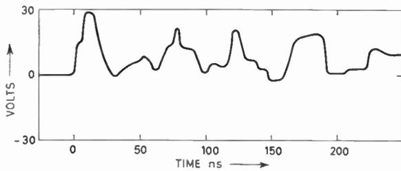
Fig. 3. Typical signal waveform from pick-up coil.
