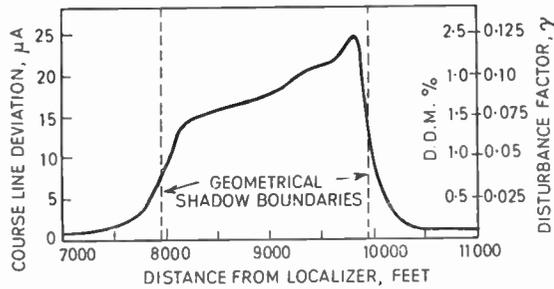
Fig. 8. Theoretical disturbance from B.E.A. Engineering Base.
