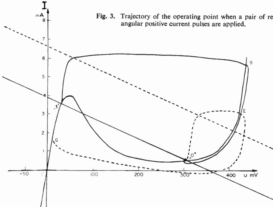
Fig. 3. Trajectory of the operating point when a pair of rectangular positive current pulses are applied.
