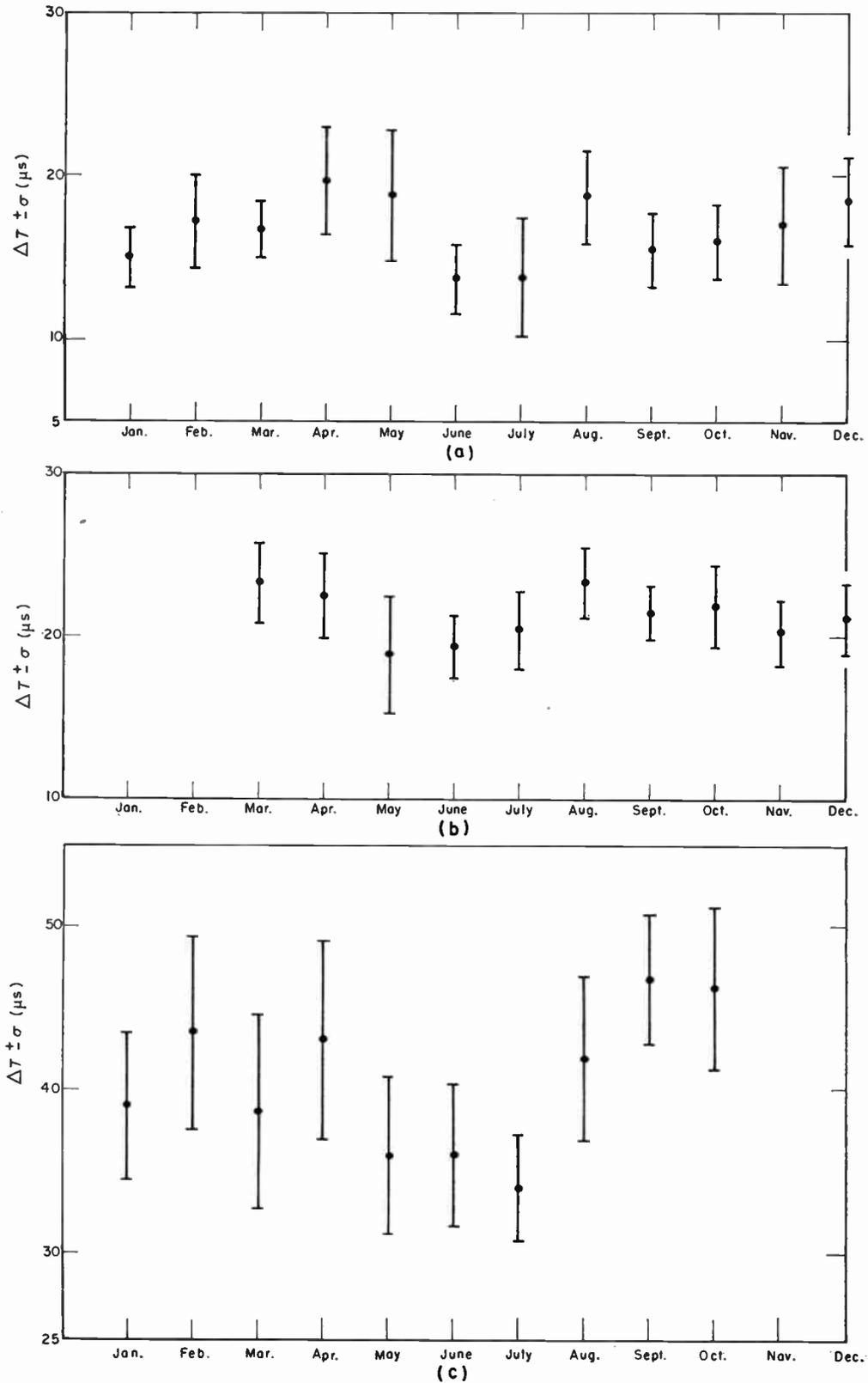
Fig. 5. Monthly variation of mean  $\Delta T$  for the paths (a) Boulder-Columbus, (b) Balboa-Columbus and (c) Rugby-Columbus.
