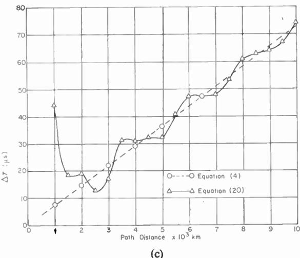
Fig. 2. Diurnal time delay  $\Delta T$  as a function of path distance for (a) 16 kHz, (b) 18 kHz and (c) 20 kHz transmissions.
