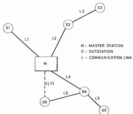
Fig. 1. Typical telemetry and telecontrol system.
