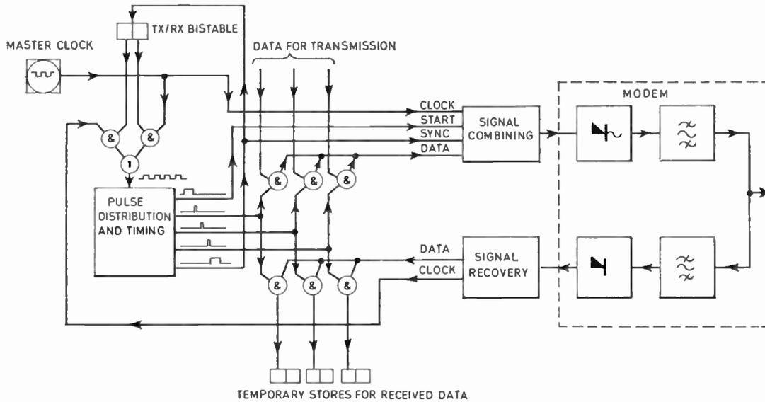
Fig. 9. Simplified operation of t.d.m. communication unit, for a 3-bit block, double-frequency-simplex master station.
