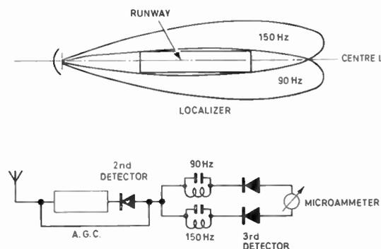
Fig. 1. Principle of I.L.S. localizer.
