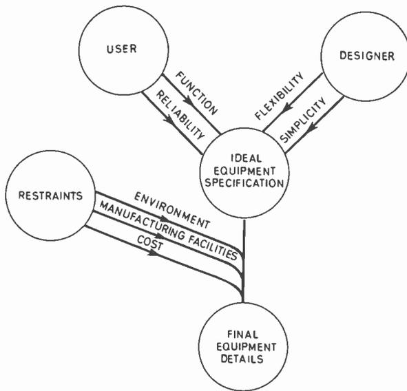
Fig. 2. Equipment design process.
