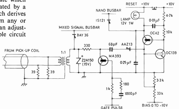
Fig. 4. Circuit of one channel.
