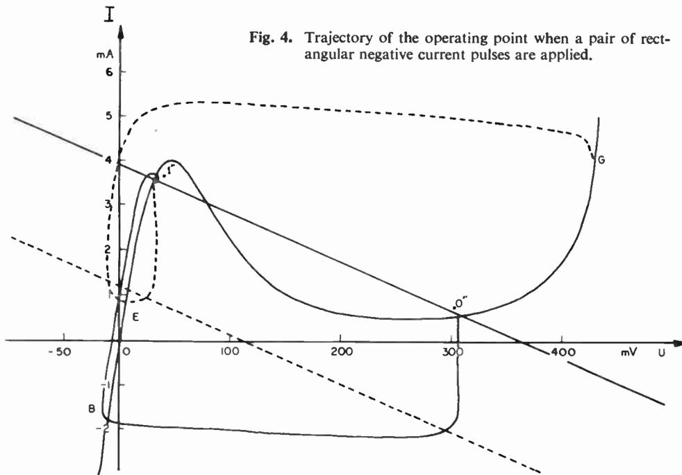
Fig. 4. Trajectory of the operating point when a pair of rectangular negative current pulses are applied.
