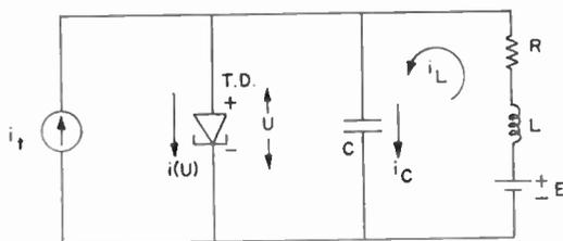
Fig. 5. Equivalent circuit of the binary counter.
