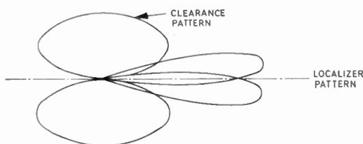
Fig. 2. Localizer and clearance arrays.
