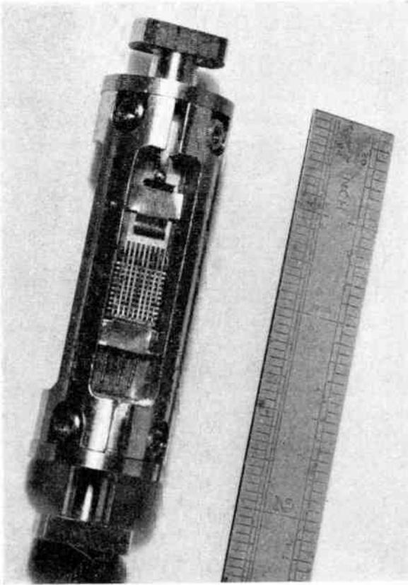
Fig. 3. Cartridge containing a module stack.
