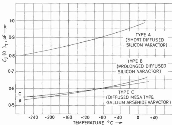
Fig. 2. Curves for zero bias capacitance against temperature.
