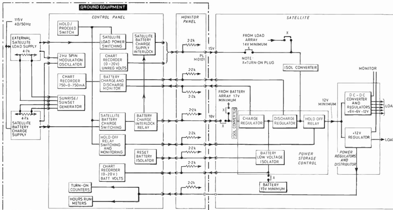
Fig. 5. Block schematic of the external power supply to satellite.
