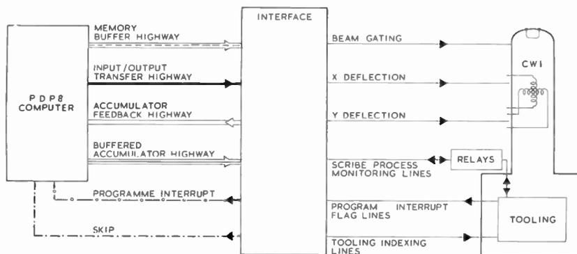
Fig. 9. Block diagram of the system.
