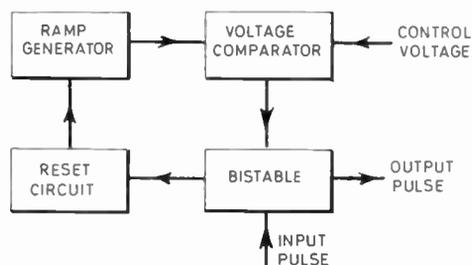
Fig. 1. Block diagram of time delay circuit.
