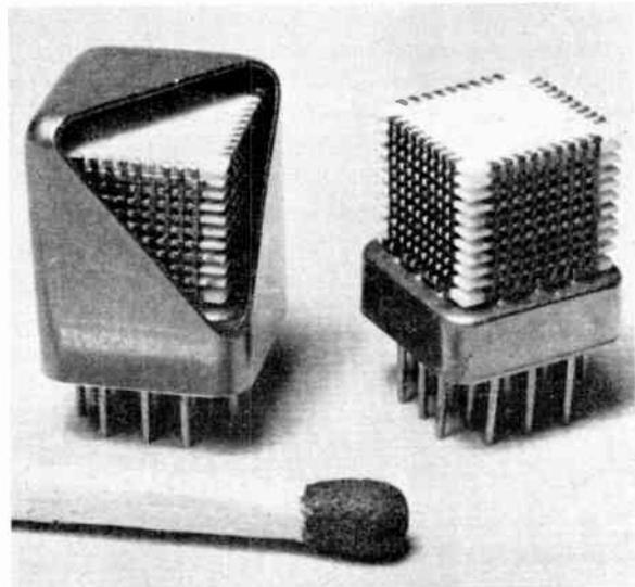
Fig. 1. The microelectronic module.
