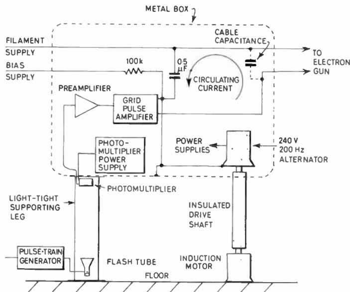
Fig. 11. Grid pulsing equipment.
