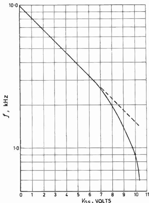
Fig. 8. Frequency versus control voltage plot for the circuit of Fig. 7.
