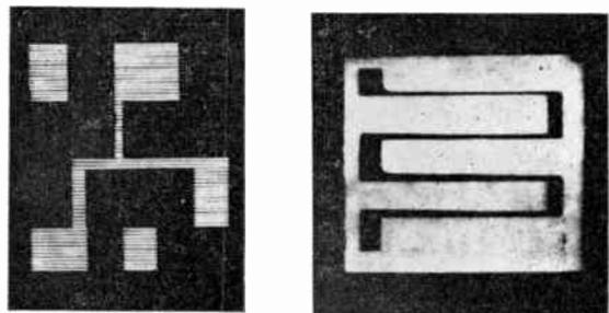
Fig. 12. Initial machining of  $750 \text{ \AA}$  tantalum film on Pyrex glass. Patterns were machined in a 1 mm square by a  $3 \mu\text{m}$  spot with  $2 \mu\text{A}$  at 20 kV swept at 80 mm/s.
