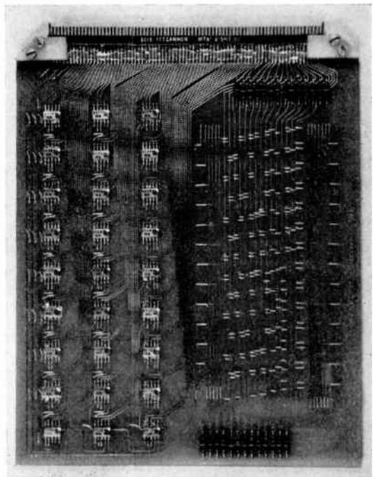
(b) Clock integrated circuit board.
