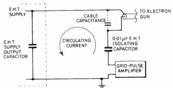
Fig. 10. Circulating current loop.
