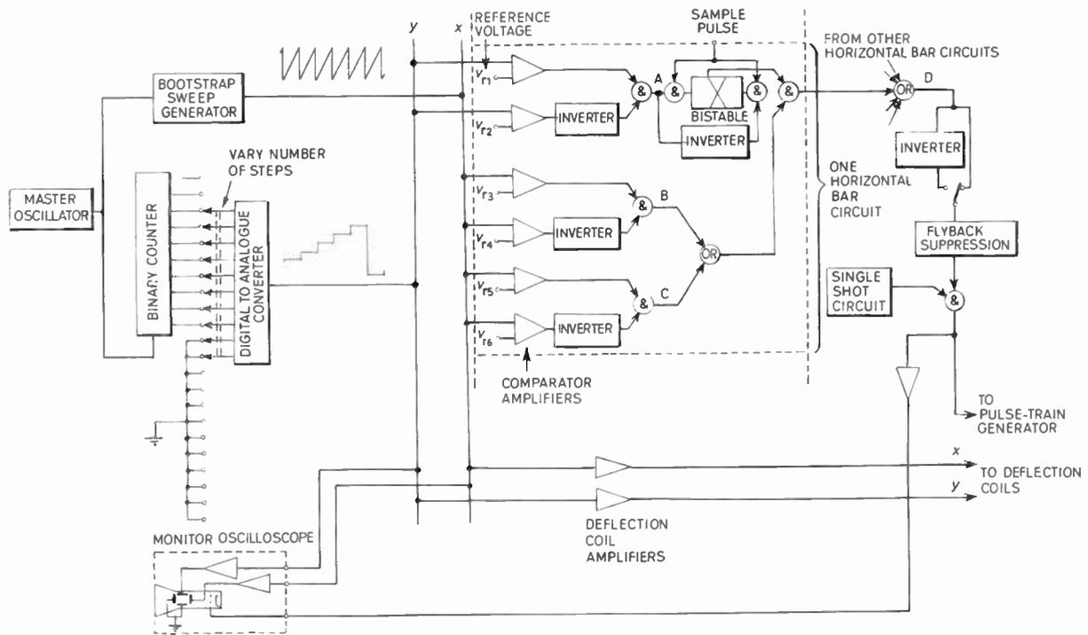
Fig. 9. Block diagram of the pattern generator.
