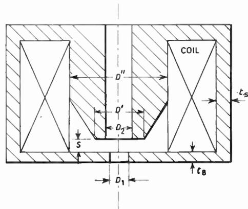
Fig. 16. Magnetic lens construction.
