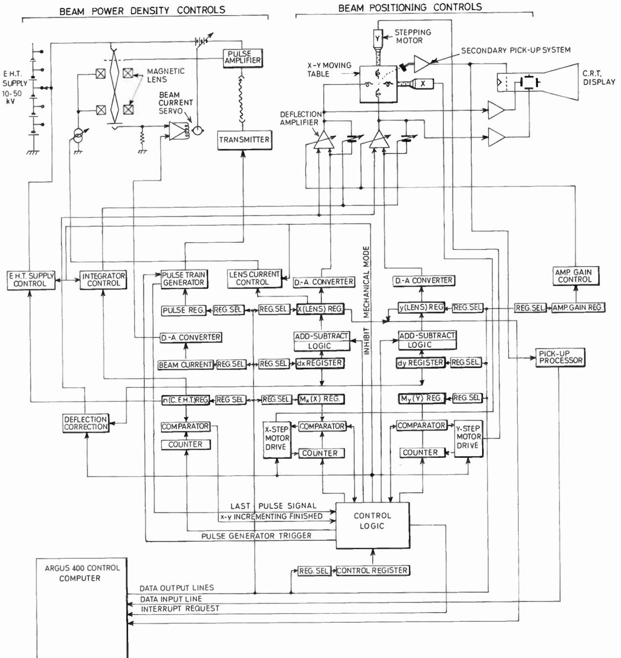
Fig. 13. Proposed control system for the electron beam machine.
