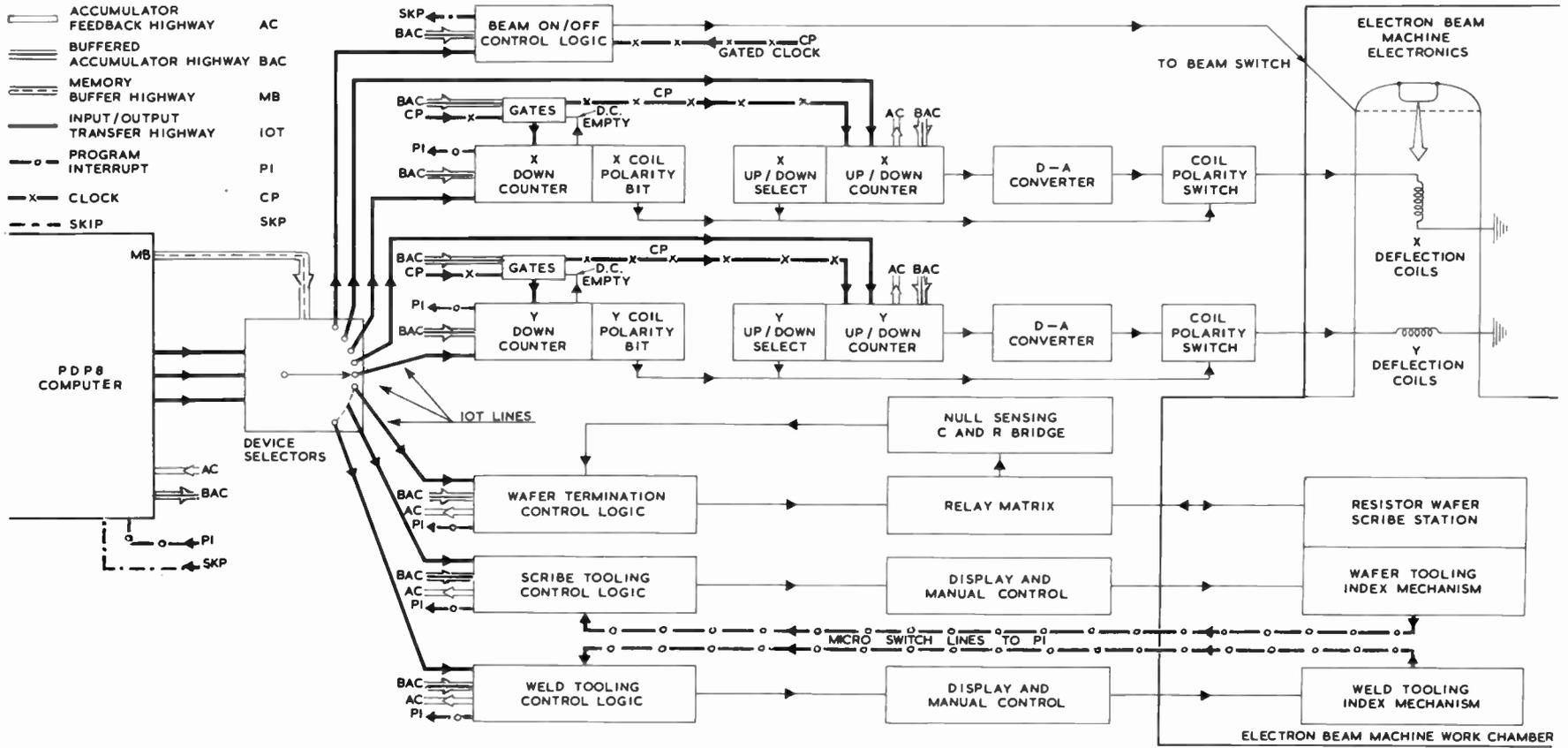
Fig. 10. Block diagram of the interface.
