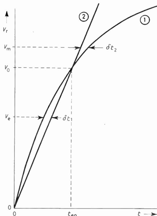
Fig. 8. Ramp linearity.
