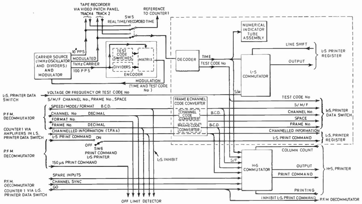
Fig. 11. Block schematic of digital clocks.
