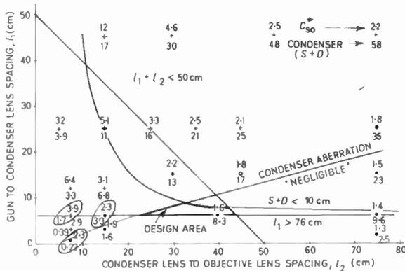
Fig. 3. Design graph for lens spacings: + condenser-lens aberration is dominant; O objective-lens aberration is dominant; ● condenser-lens aberration is negligible.
