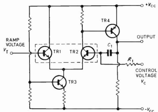
Fig. 5. Simplified voltage comparator circuit.
