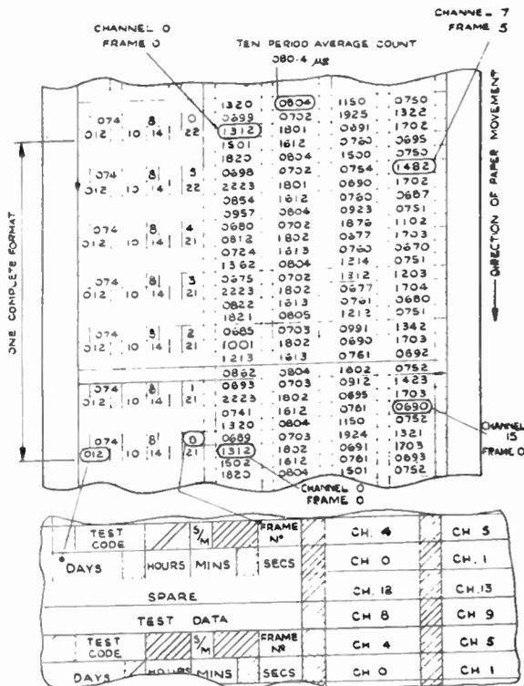
Fig. 10. Typical high-speed print-out.
