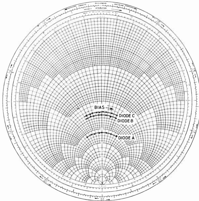
Fig. 7. Loci of spreading resistance ( $R_s$ ) normalized to  $R_s$  at 77°K, for bias 0–3V.
