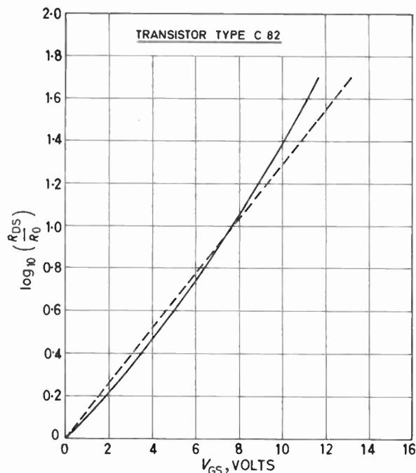
Fig. 1. Resistance versus control voltage characteristic for a 'remote pinch-off' f.e.t.
