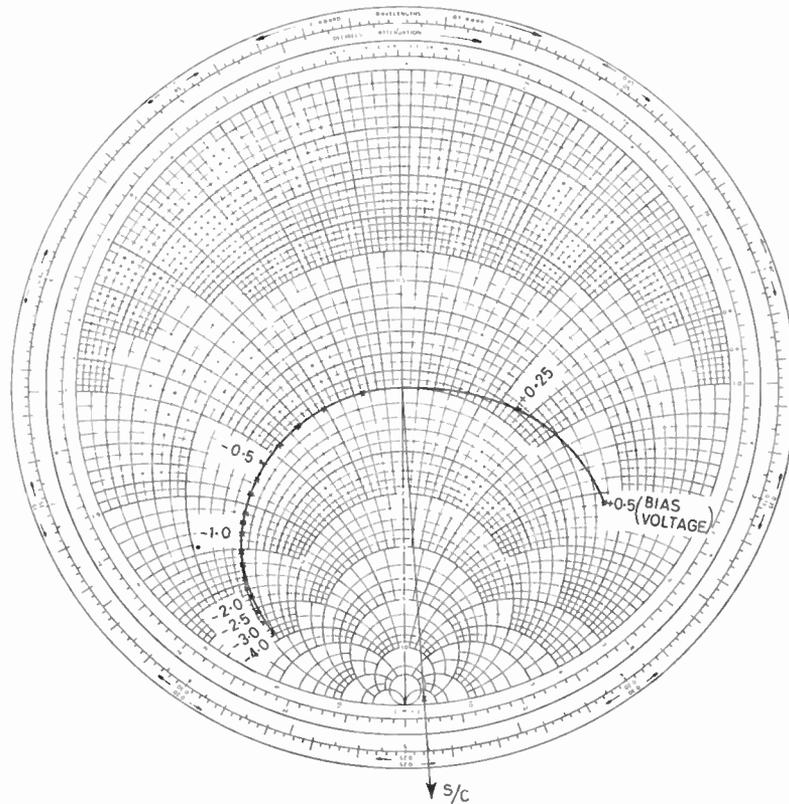
Fig. 4. Diode impedance plot derived by Harrison's method (gallium arsenide varactor).
