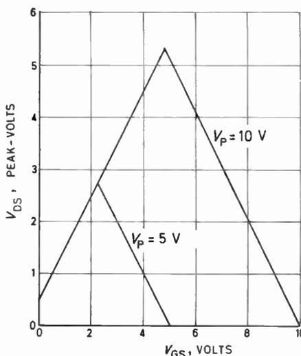
Fig. 2. Permitted operating regions for ohmic behaviour. The device behaves as an ohmic variable resistor provided that the peak drain voltage is such that the working point is within the triangle appropriate to the pinch-off voltage of the device in use.
