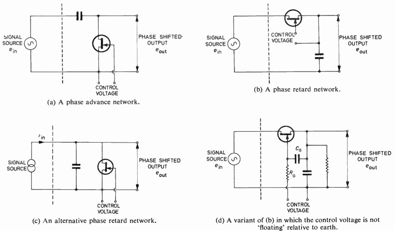
Fig. 3. Simple phase-shift networks using f.e.t.'s.
