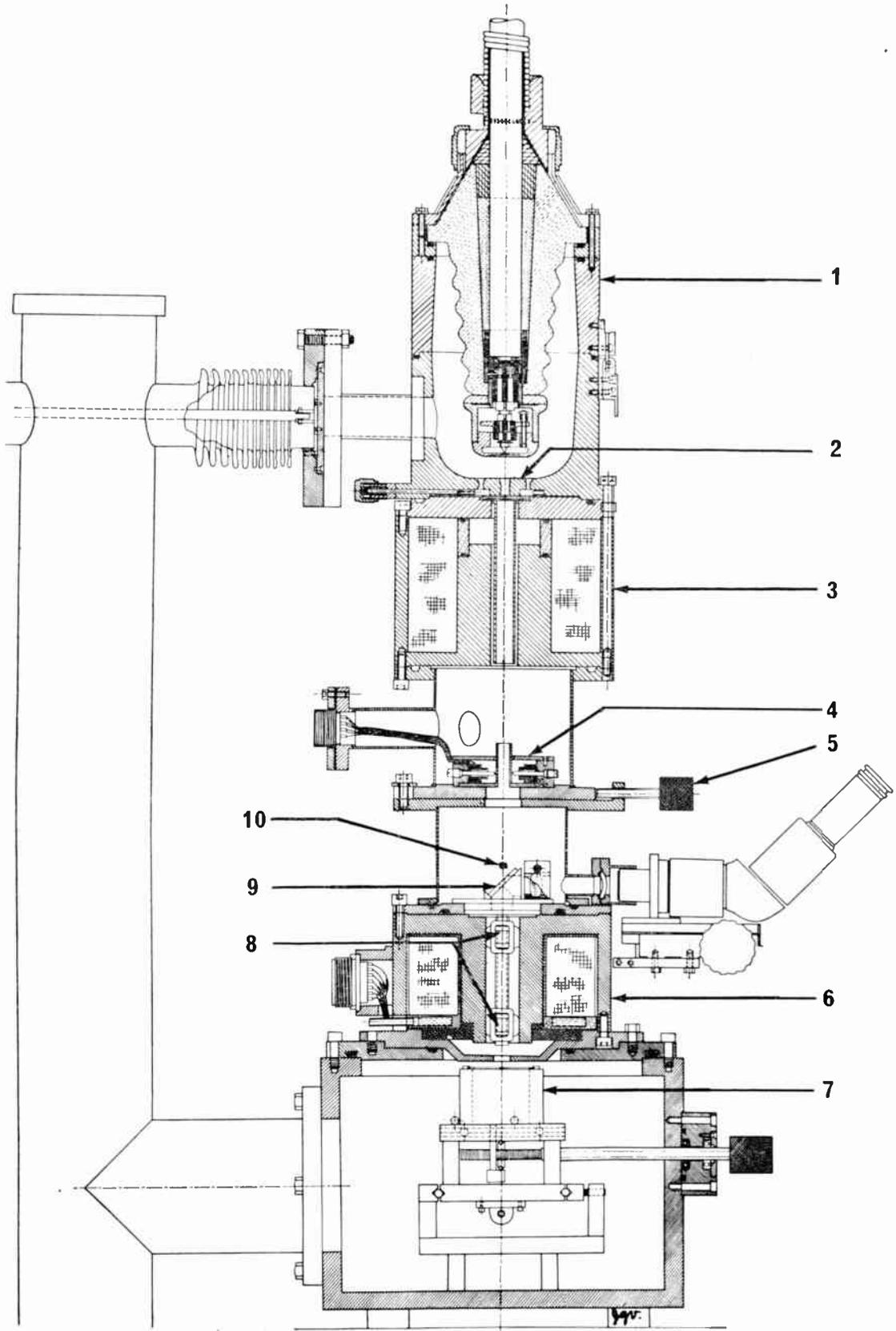
Fig. 4. Cross-section of the electron beam machine.
