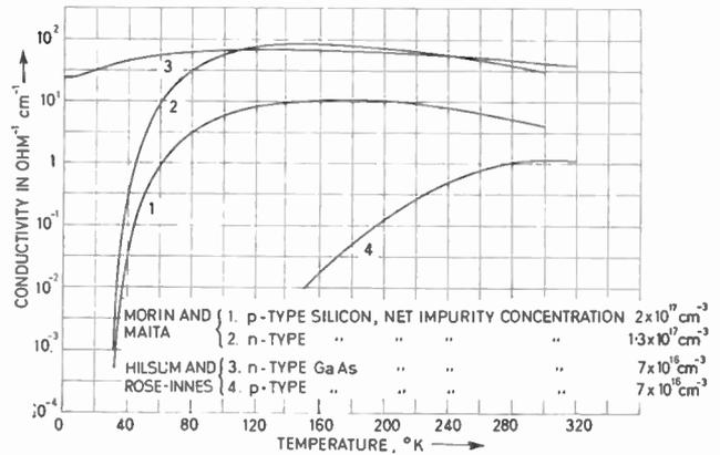
Fig. 3. Curves showing the variation of conductivity with temperature.
