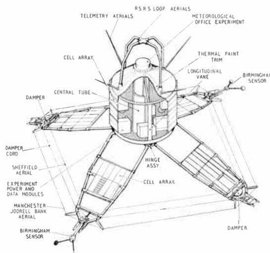
Fig. 1. UK-3 satellite with experiment sensors.
