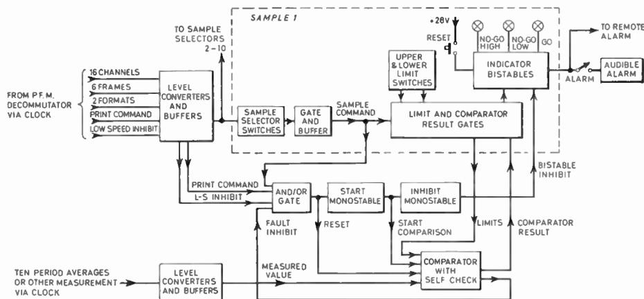
Fig. 13. Block schematic of the off-limit detector.
