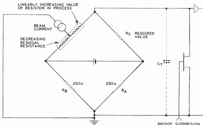
Fig. 11. The bridge circuit configuration.
