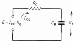
Fig. 4. Circuit for determination of ramp linearity.
