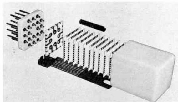
Fig. 2. Module piece parts.
