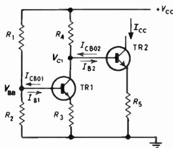
Fig. 9. Compensated constant current generator.
