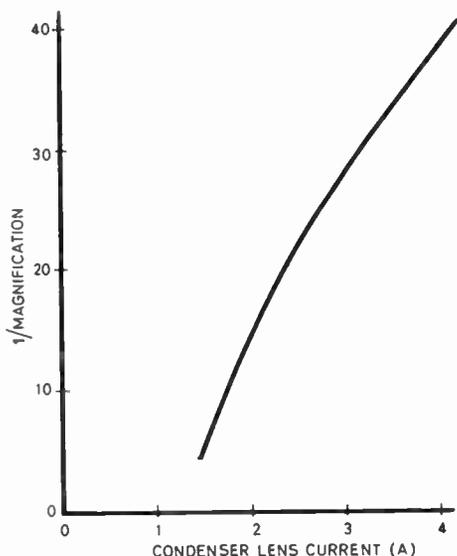
Fig. 5. Variation of column magnification with condenser-lens current. (Lens coil is tapped to give 335, 473 and 749 turns at 10 kV, 20 kV and 50 kV respectively.)
