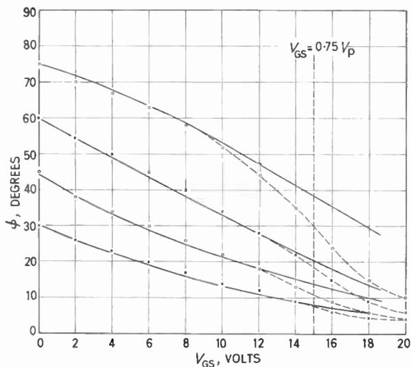
Fig. 4. Characteristics obtained with the network of Fig. 3(a). Points and broken line: experimental results. Full line: values predicted by eqn. (4).
