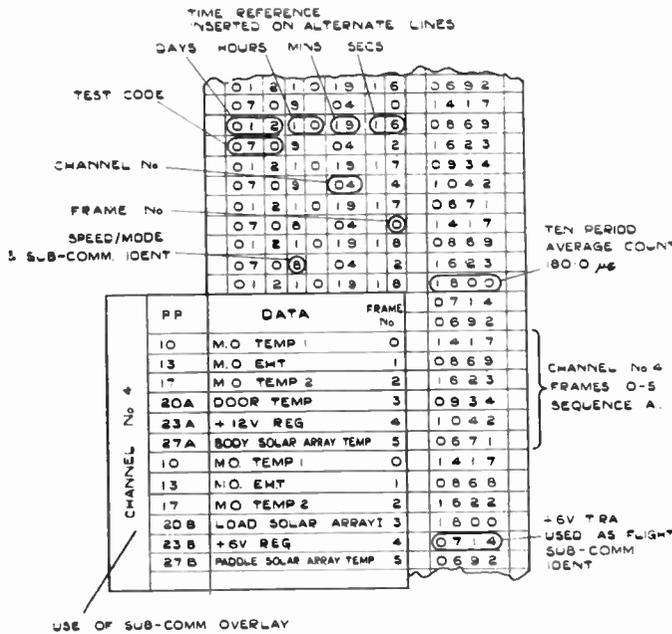
Fig. 7. Typical low-speed print-out.
