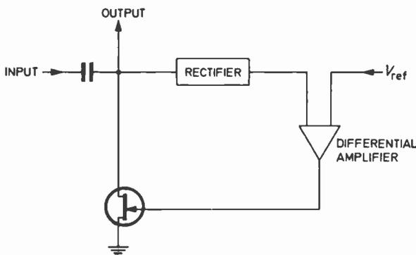
Fig. 9. A system which produces constant phase shift of a sinusoid.
