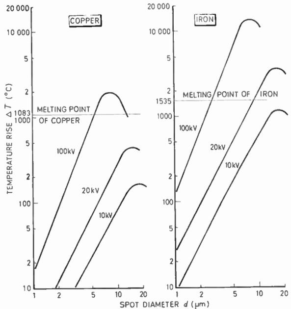
Fig. 2. Theoretical heating of copper and iron targets by the electron beam,  $C_s = 3$  cm,  $\rho_c = 2$  A/cm<sup>2</sup>.
