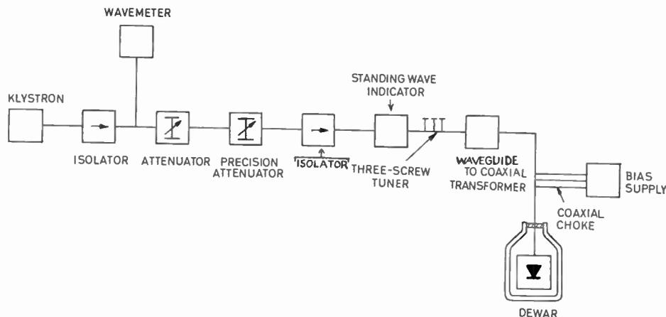
Fig. 6. Block diagram of measuring apparatus.
