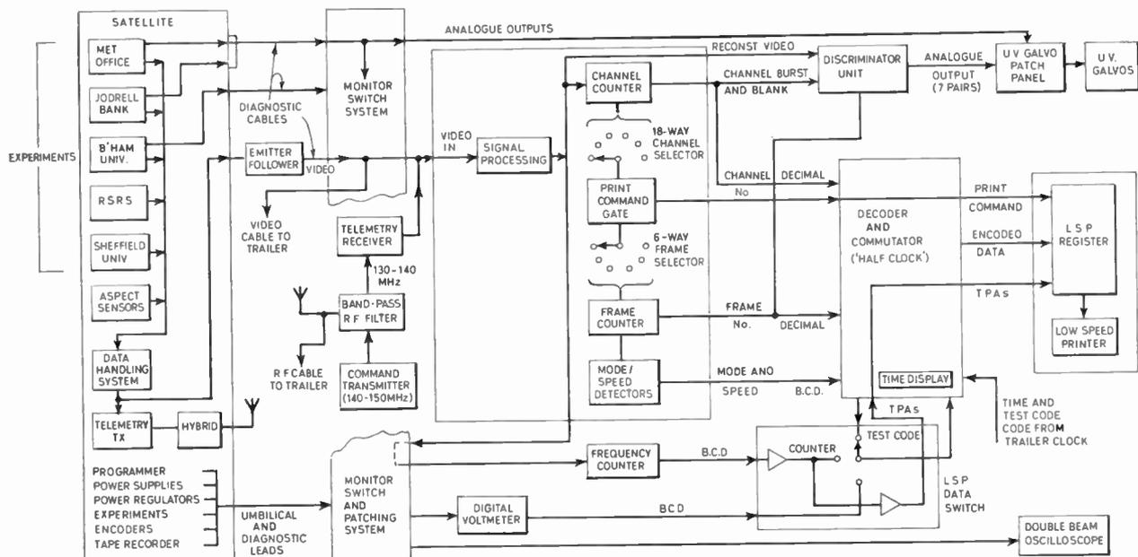
Fig. 6. Block schematic of the data extraction in mobile check-out equipment.
