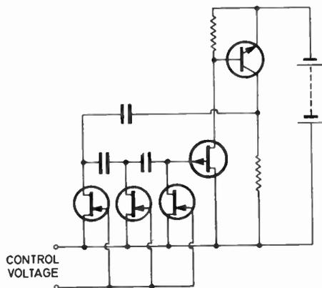
Fig. 7. A voltage-controlled variable frequency oscillator.
