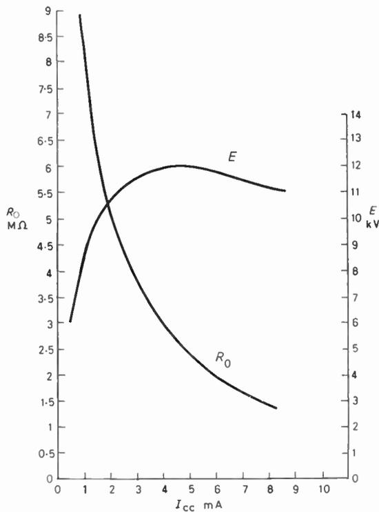
Fig. 6. Collector output resistance  $R_o$ , and aiming voltage  $E$ , where  $E = I_{cc}R_o$ . Transistor (half) 2N2060. Measured under large signal conditions with  $R_b = R_o = 10\text{ k}\Omega$ .
