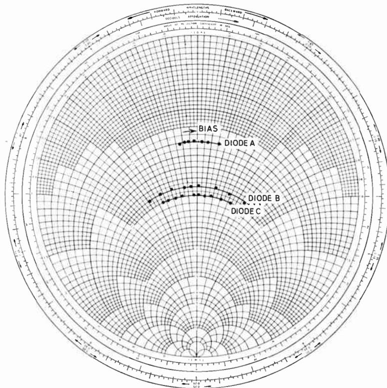
Fig. 8. Loci of spreading resistance ( $R_s$ ) normalized to  $R_s$  at 4°K, for bias range 0–3V.
