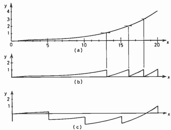
Fig. 14. Non-linear deflection correction.
