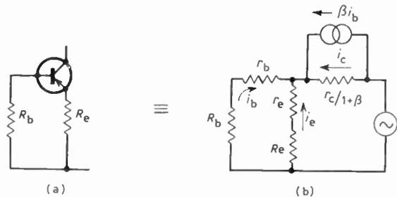
Fig. 3. Circuits for determination of output resistance.
