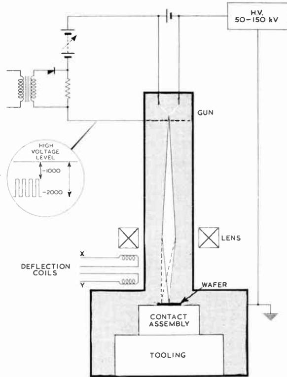
Fig. 8. Block diagram of a CW-1 and the electron optical system.
