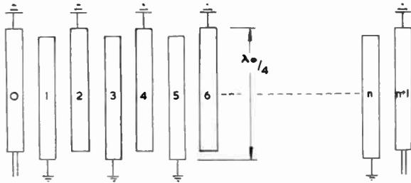
Fig. 1. Narrow-band interdigital structure.
