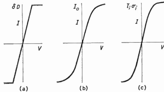
Fig. 2. Three different forms of amplitude limiter.
