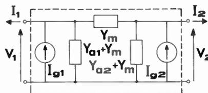
Fig. 3. A two-port antenna with equivalent circuit.
