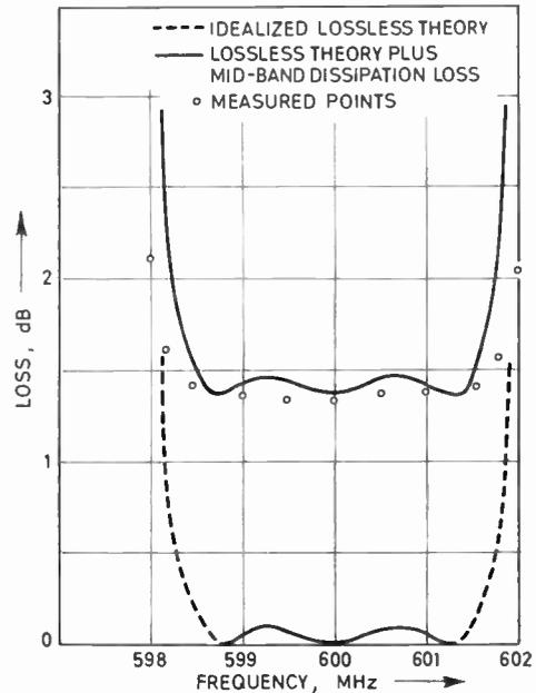
Fig. 15. Comb-line filter response.
