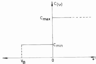
Fig. 2. Idealized capacitance vs. voltage.
