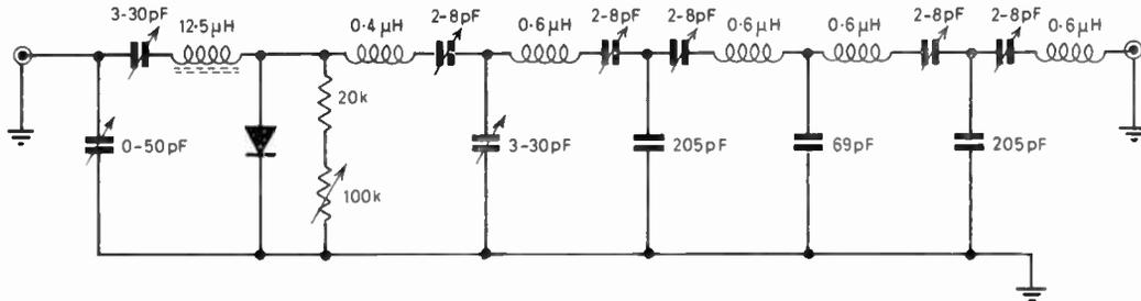
Fig. 10. Circuit diagram of the complete multiplier.
