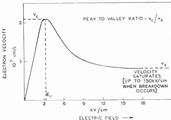
Fig. 1. Velocity-field characteristic (after Butcher and Fawcett<sup>6</sup>).
