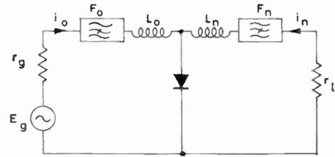
Fig. 4. Schematic diagram of multiplier.
