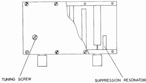
Fig. 16. Interdigital filter with band-stop elements.
