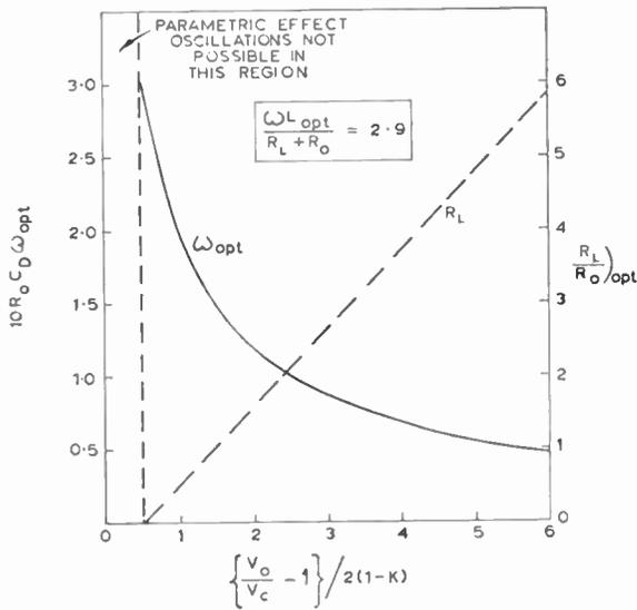
Fig. 9. Variation of frequency for optimum power output with applied bias.
