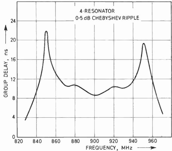
Fig. 10. Typical group-delay characteristic.
