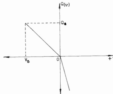
Fig. 3. Idealized charge vs. voltage.
