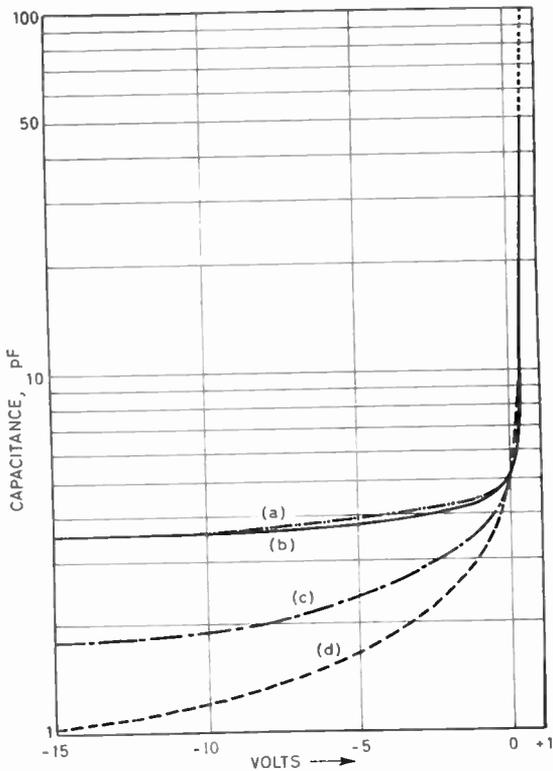
Fig. 1. Variation of capacitance with applied voltage for a step-recovery diode.
