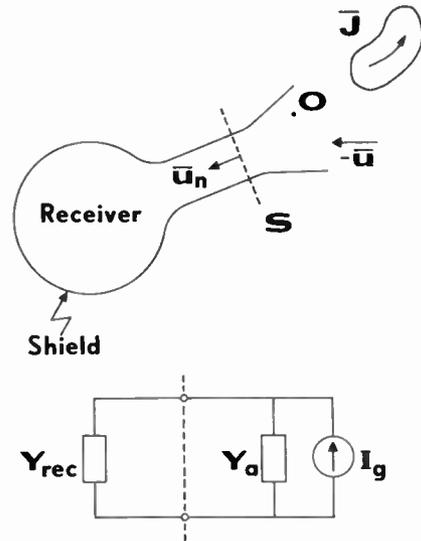
Fig. 2. A one-port antenna with equivalent circuit.
