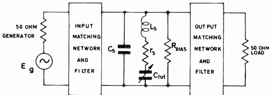
Fig. 6. Schematic diagram of a practical multiplier.
