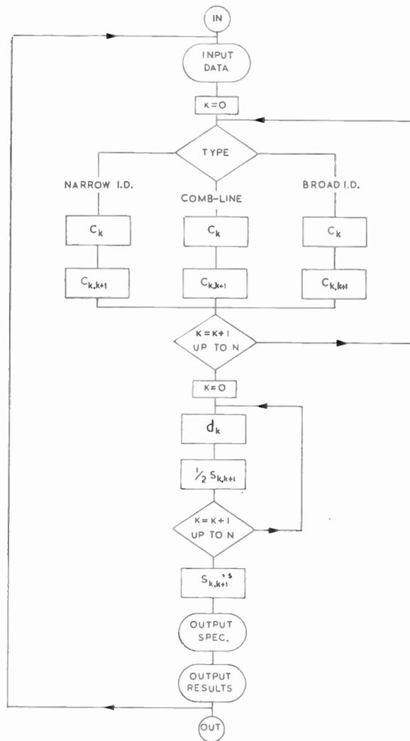
Fig. 18. Flow-chart for interdigital and comb-line filter program.
