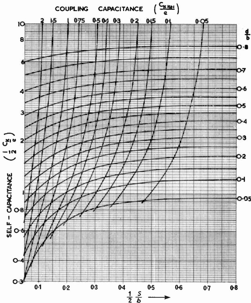
Fig. 7. Graph of rod diameters and spacings (after Cristal<sup>4</sup>).
