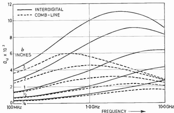
Fig. 14. Unloaded- $Q$  of slab-line resonator.
