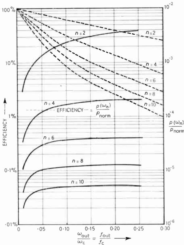
Fig. 7. Variation of efficiency and normalized output power as a function of  $f_{out}/f_c$ .
