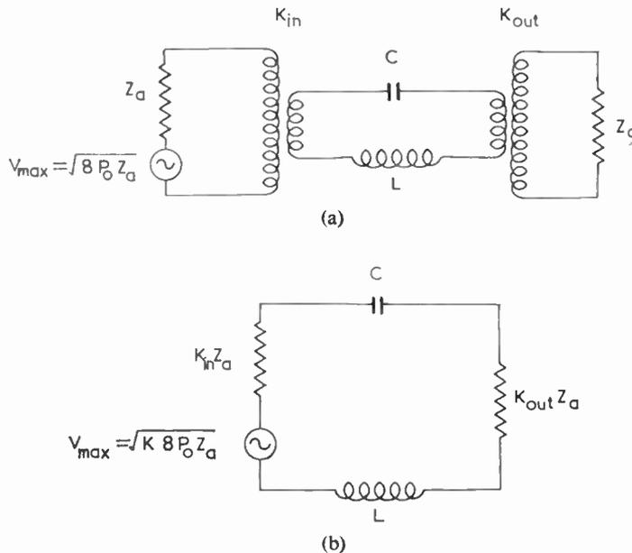
Fig. 17. Equivalent circuits of a lossless resonator.
