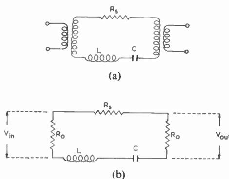
Fig. 11. Resonator equivalent circuits.
