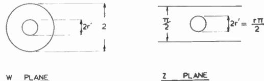
Fig. 13. Conformal mapping  $w = \tan z$ .
