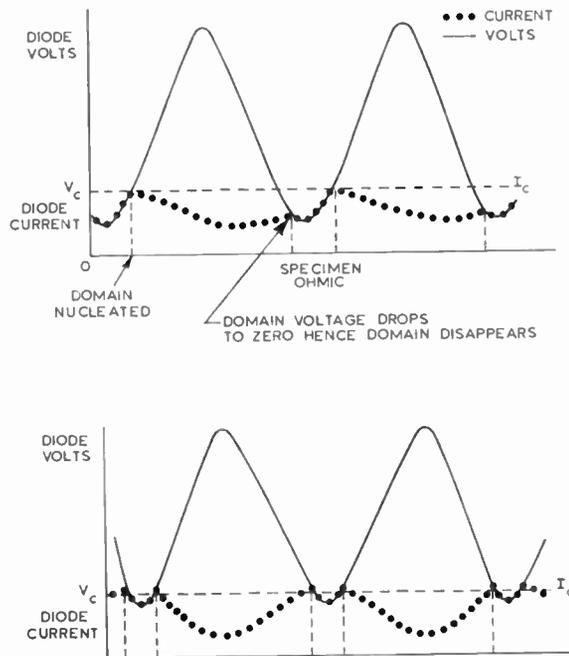
Fig. 7. Negative resistance modes (quenched domain modes or l.s.a. mode).
