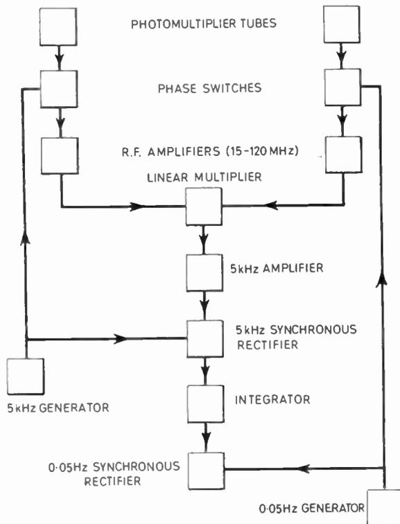
Fig. 1. Block diagram of the correlator.
