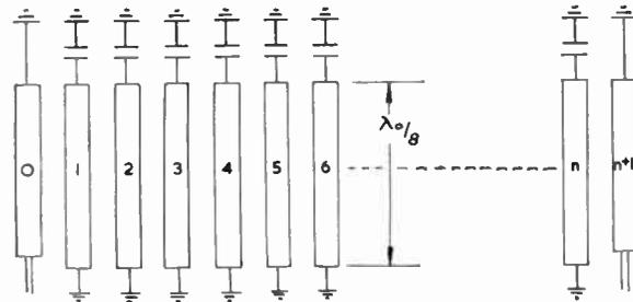
Fig. 3. Narrow-band comb-line structure.
