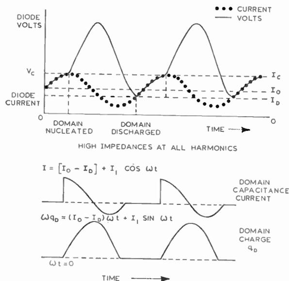
Fig. 8. Idealized parametric mode.
