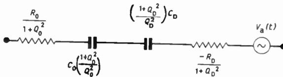
(b) Equivalent series form at frequency  $\omega$ .
