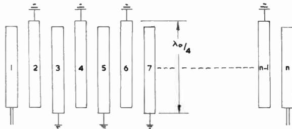
Fig. 2. Broad-band interdigital structure.
