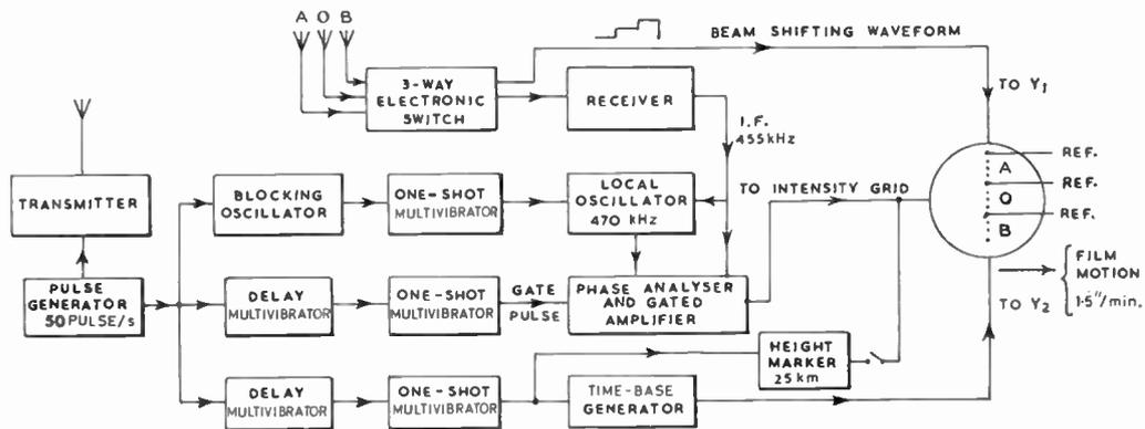
Fig. 3. Block diagram of the spaced aerial phase path recording equipment.
