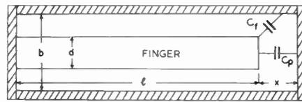
Fig. 8. Capacitances at open-circuit end of interdigital element.
