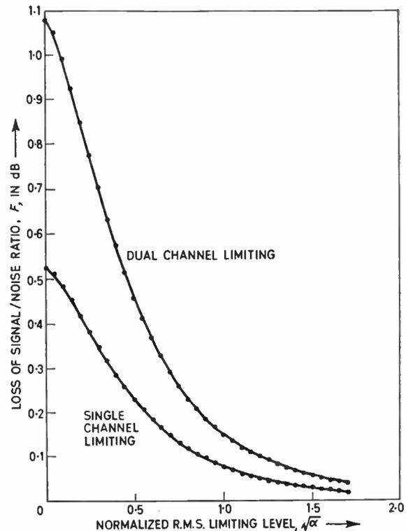
Fig. 3. Loss of signal/noise ratio as a function of limiting level.
