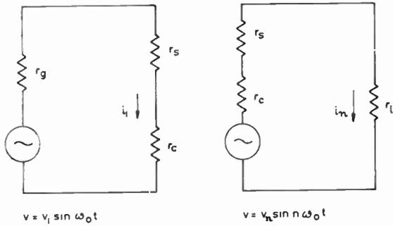
Fig. 11. Equivalent circuits of the diode at input and output frequencies for tuned operation.
