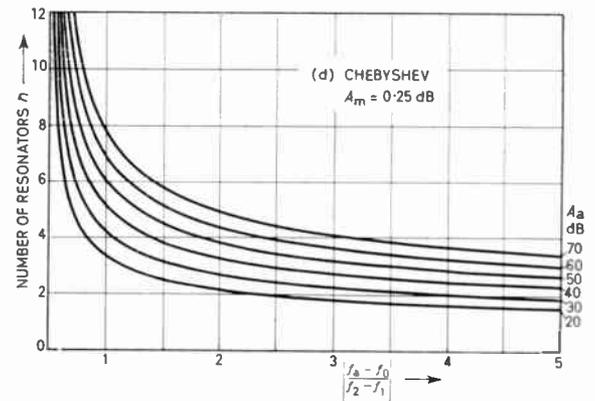
Fig. 4. Number of resonators,  $n$ , against frequency parameter for various degrees of attenuation.
