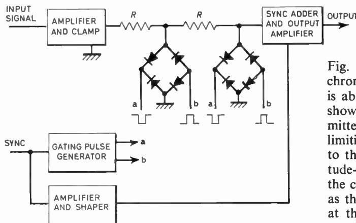
Fig. 6. Stabilizing amplifier.
