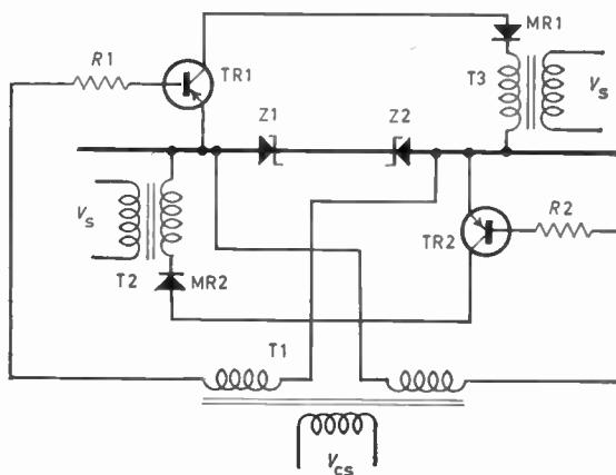
Fig. 21. Common-collector circuit using additional a.c. supply.
