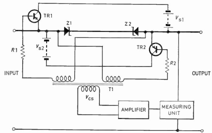
Fig. 16. Transformerless class-B common-collector circuit.
