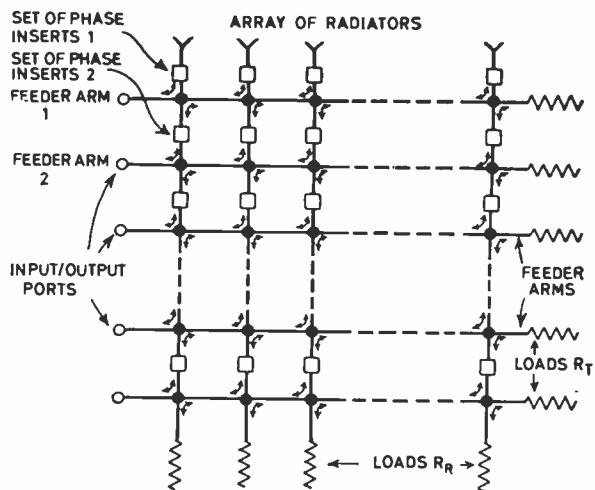
Fig. A. Schematic of Maxson multi-beam antenna.
