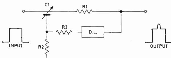
(a) Circuit for the production of a voltage spike, superimposed on a biasing pulse. DL = delay line.
