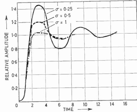
Fig. 9.  $N = 6$  In-line pole step response.
