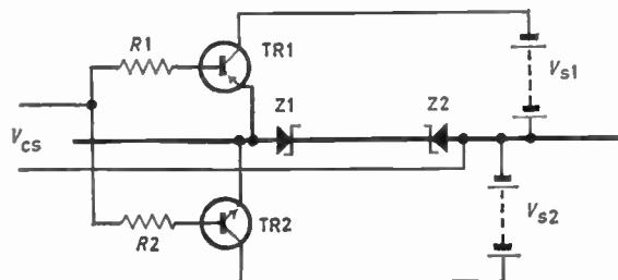
Fig. 19. Common-collector circuit using complementary transistors.
