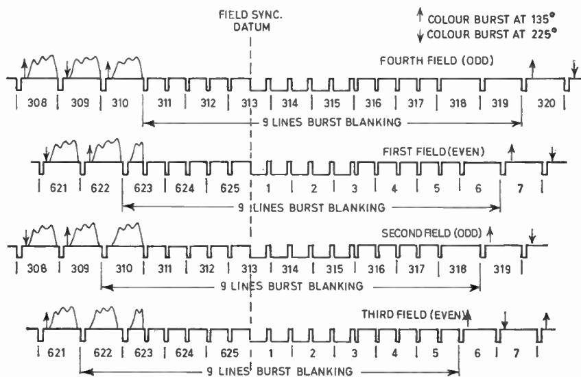
Fig. 2. Burst blanking.
