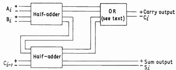
Fig. 3. Schematic arrangement of a full-adder.
