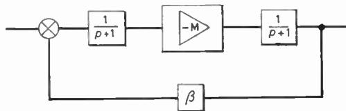
(a) Basic configuration of a system for generating conjugate pole-pairs (the pole-forming networks have been normalized).
