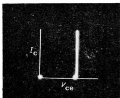
(a) No control voltage  $V_{ru} = 0.1 \text{ V}$
