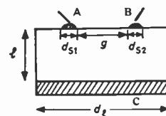
Fig. 3. A Gunn-effect comparator (triode).
