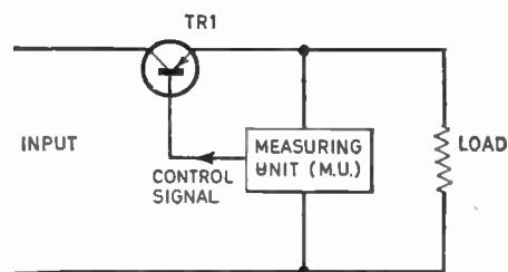
Fig. 1. Basic stabilizer circuit.
