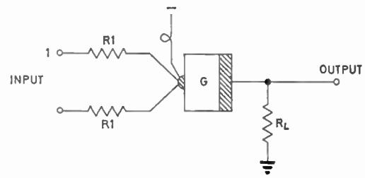
Fig. 9. A Gunn-effect AND circuit.
