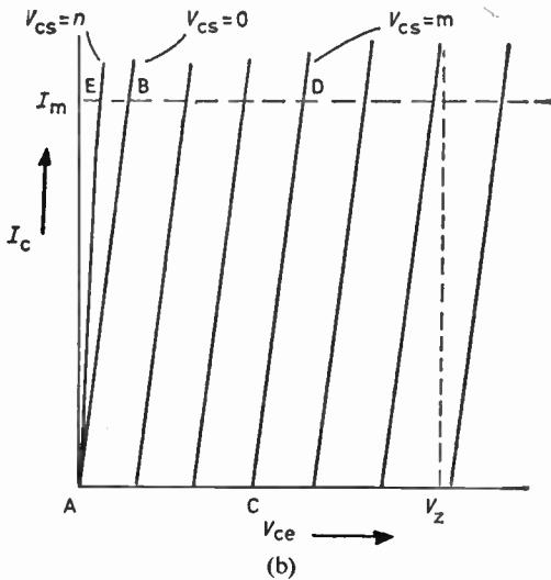
Fig. 8. (a) Common-collector circuit; (b) common-collector characteristics.
