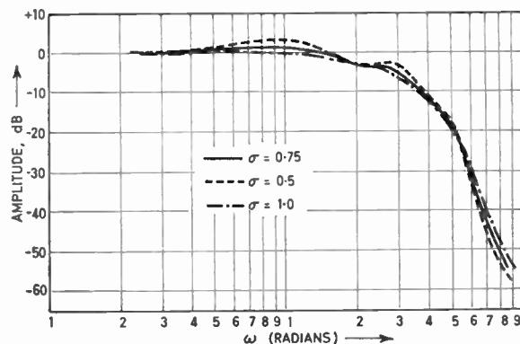
Fig. 3.  $N = 6$  In-line pole amplitude response.
