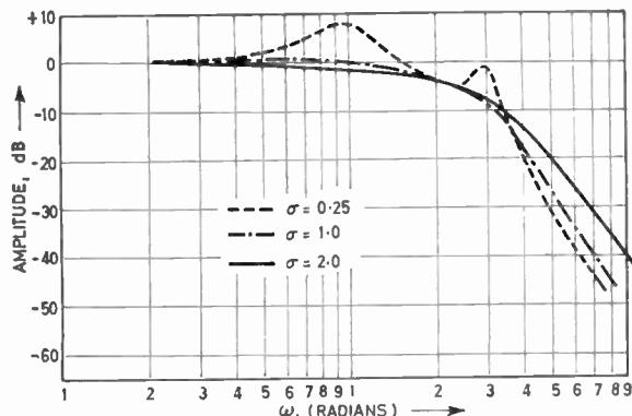
Fig. 6.  $N = 4$  In-line pole amplitude response.
