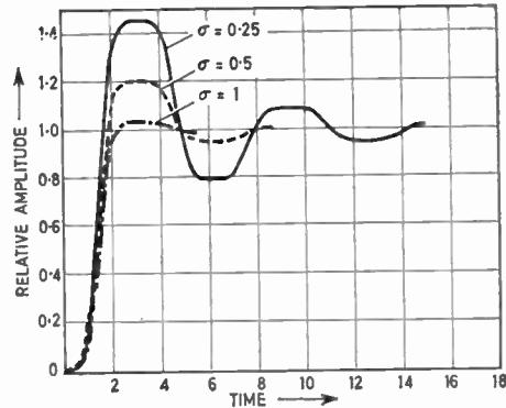
Fig. 8.  $N = 4$  In-line pole step response.
