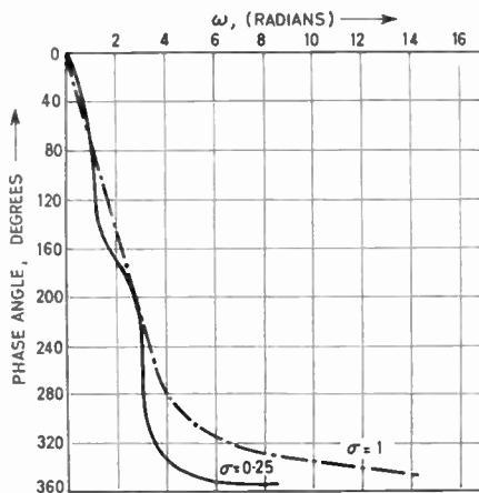
Fig. 4.  $N = 4$  In-line pole phase response.
