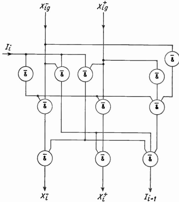
The schematic arrangement resulting from these equations is shown in Fig. 2. Many alternatives are possible depending on the availability of logic operators supplied by any given manufacturer. It is interesting to note that the same circuit will generate the cyclic code from the natural form.
