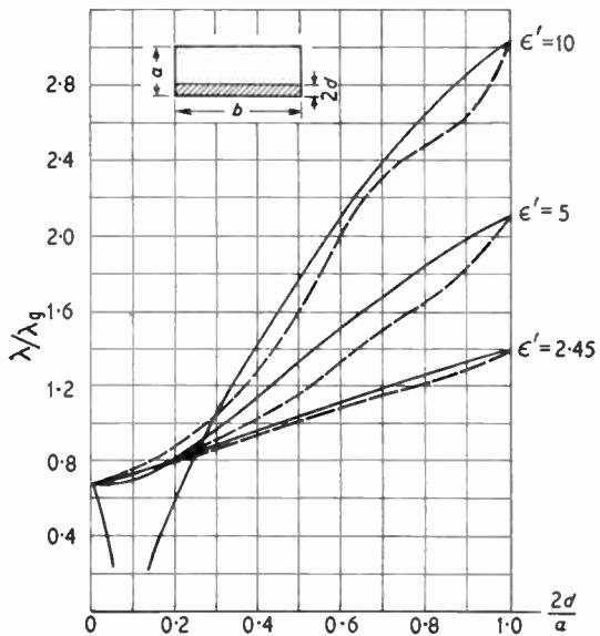
Fig. 1. Comparison of the approximate and exact solutions for the wavelength of the quasi- $TE_{01}$  mode in a rectangular waveguide with a dielectric slab.
