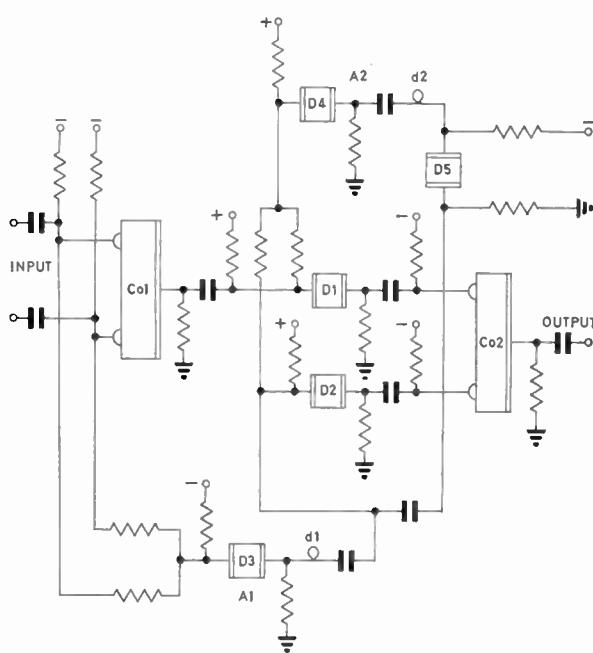
Fig. 10. Binary sequential adder.
