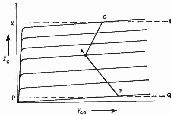
Fig. 13. Operating line for class-A common-emitter circuit showing serious distortion.
