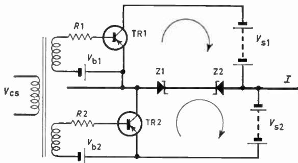
Fig. 14. Transformerless class-B common-emitter circuit.
