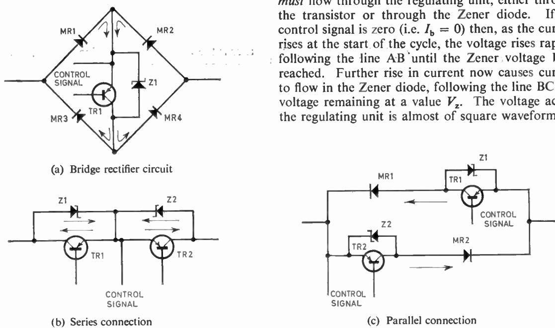
Fig. 6. Methods of connecting transistors in a.c. regulating units.
