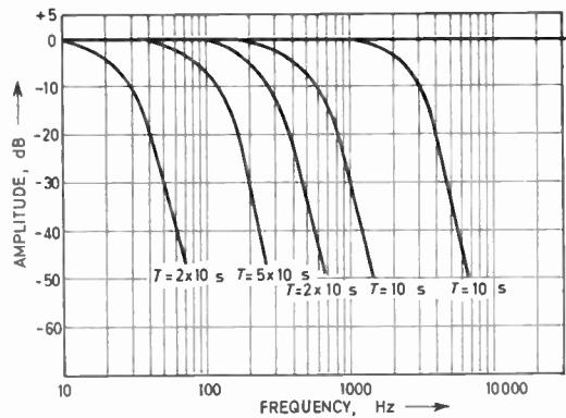
Fig. 14. Curves of  $N = 6$ ,  $\delta = 1$  in-line pole filter.
