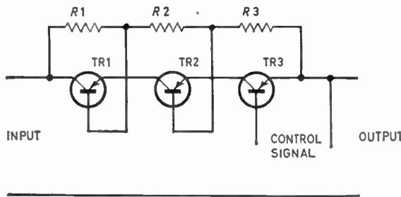
Fig. 2. Use of transistors in series.
