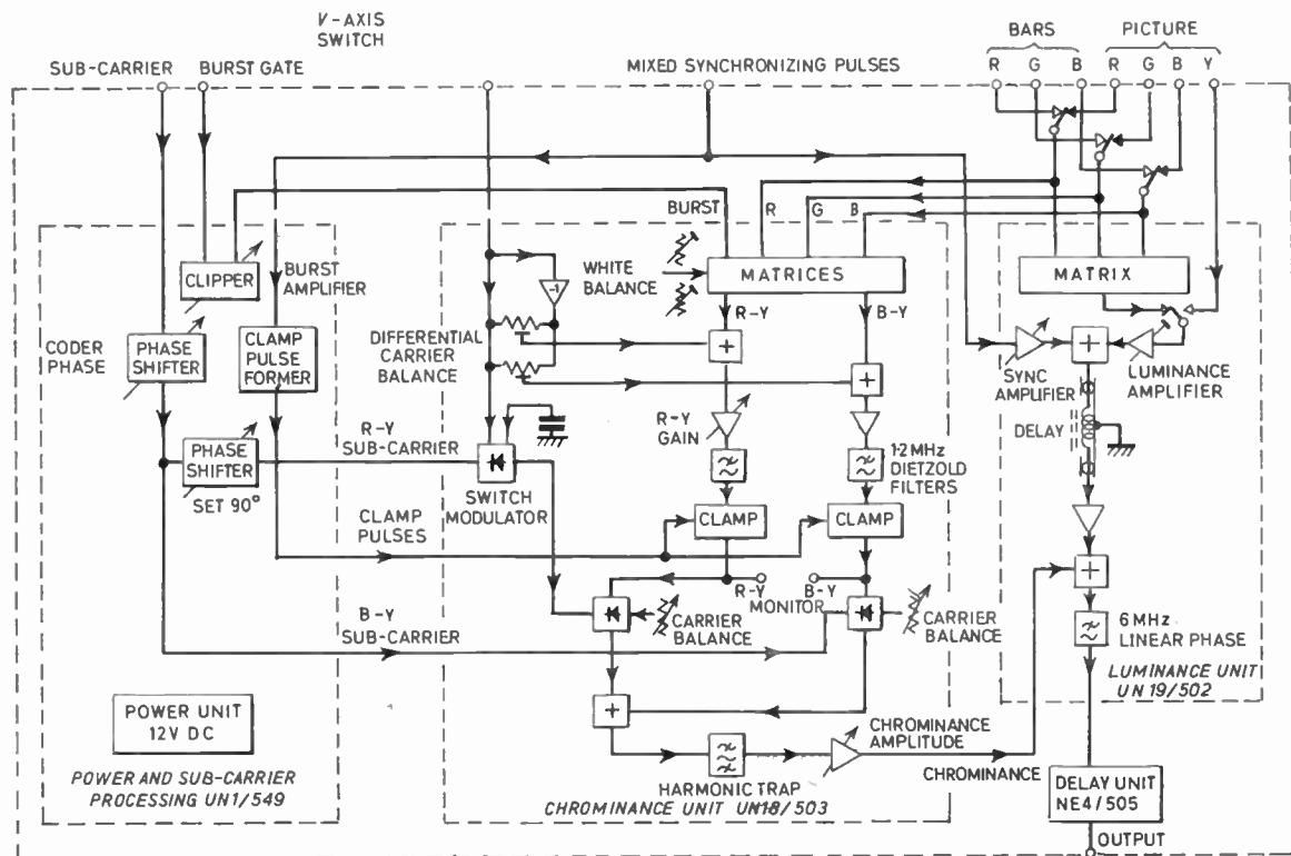
Fig. 4. PAL colour coder (B.B.C. type GE1M/526).
