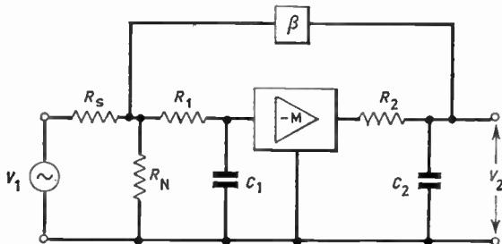
(b) Schematic diagram giving the de-normalized arrangement for generating conjugate pole-pairs.
