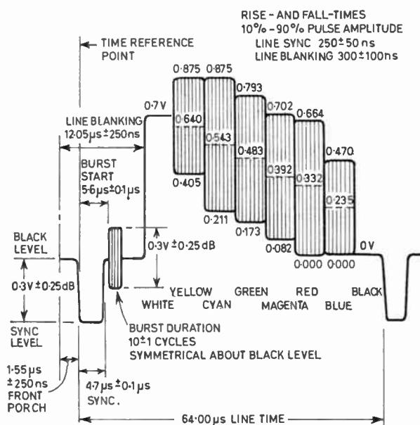
Fig. 7. 95% colour bars—line waveform.
