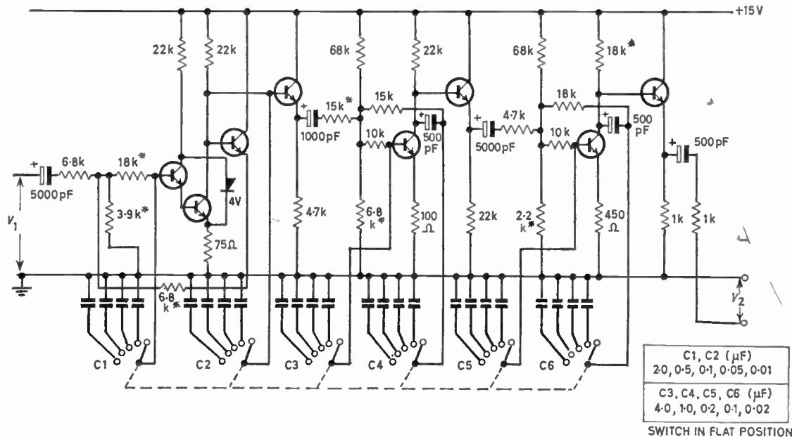
Fig. 12. Circuit diagram of the  $N = 6$  in-line pole filter.
