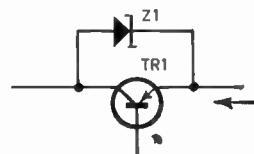
Fig. 5. Use of Zener diode to limit the voltage across the regulating unit.
