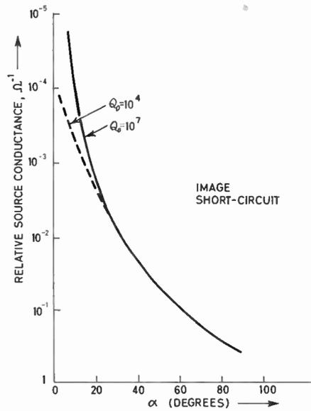
Fig. 9. Source conductance for narrow-band mixer using asymmetric diode.
