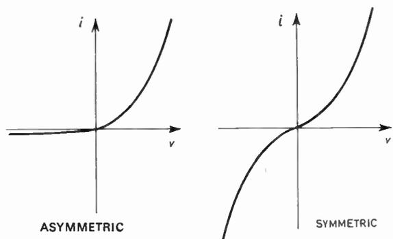
Fig. 2. Diode characteristics.
