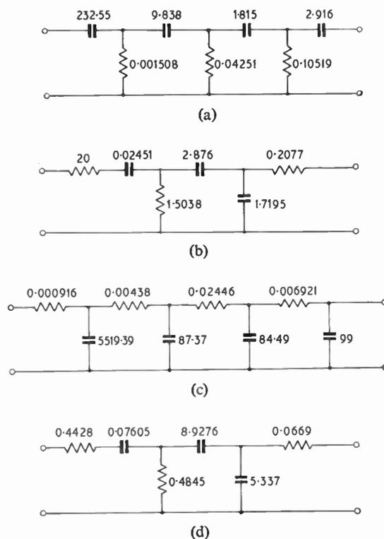
Fig. 1. Parallel ladders of a fourth-order network.
