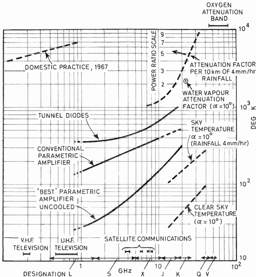
Fig. 1. Frequency band allocation, 'state of the art', and natural limitations based on Refs. 2, 3, 4.
