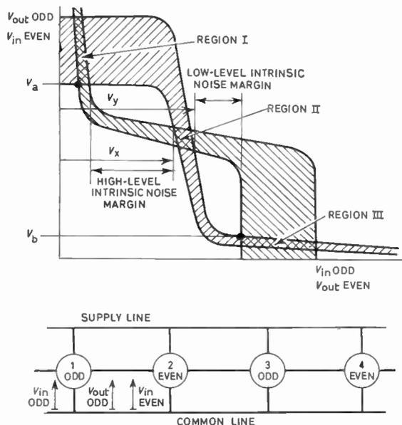
Fig. 9. Logical compatibility diagram and cascade of gates.
