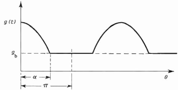
Fig. 7. Asymmetrical diode conductance.
