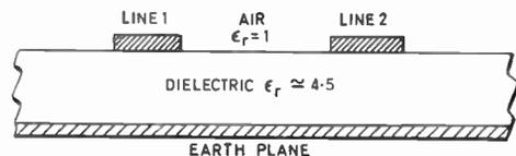
Fig. 2. Typical microstrip transmission system.
