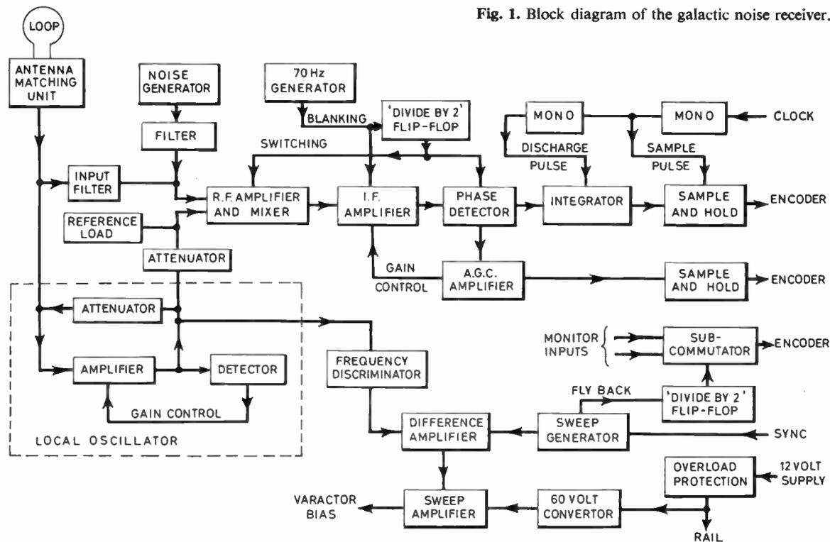
Fig. 1. Block diagram of the galactic noise receiver.
