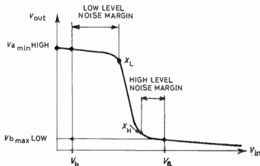
Fig. 11. Nominal transfer characteristic with input and output level limits.
