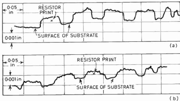
Fig. 4. (a) Profiles of dried but unfired prints from a ruthenium oxide ink.
