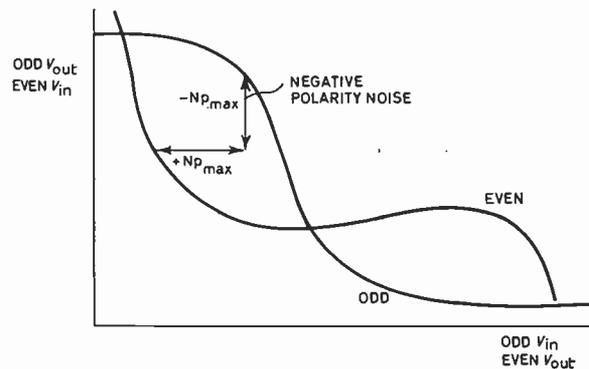
Fig. 12. Definition of d.c. noise margin based on logical compatibility diagram.
