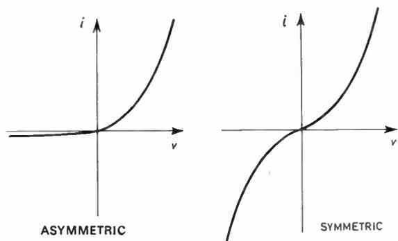
Fig. 2. Diode characteristics.
