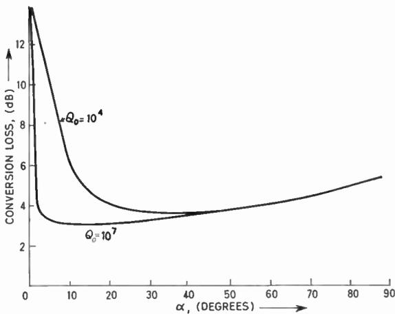
Fig. 10. Conversion loss of broad-band mixer using asymmetrical diode.
