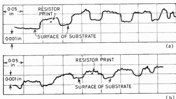
Fig. 4. (a) Profiles of dried but unfired prints from a ruthenium oxide ink.
