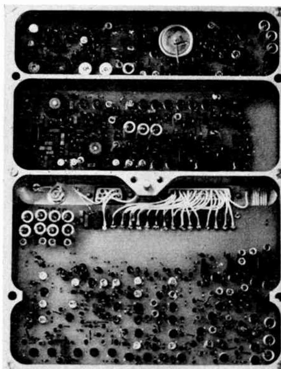
Fig. 3. View of the receiver, before foam encapsulation, showing (top to bottom) the low-frequency and data handling section, the r.f. and i.f. section and the frequency-sweep and converter section.
