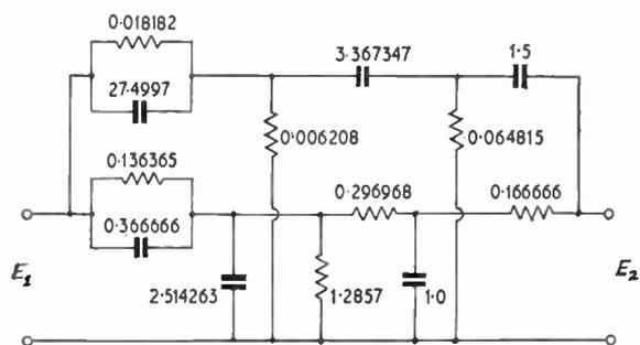
Fig. 2. Third-order rational transfer function network.
