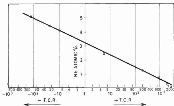
Fig. 2. Dependence of temperature coefficient of resistance (t.c.r.) on dopant level in host oxide.
