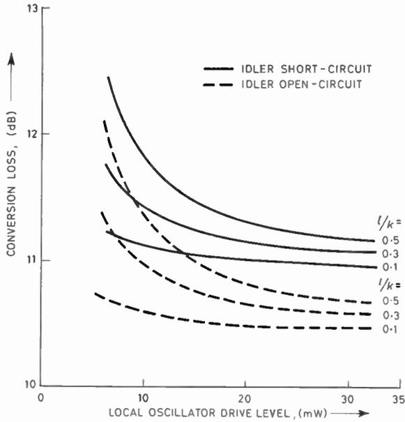
Fig. 6. Influence of shunt linear conductance on loss.
