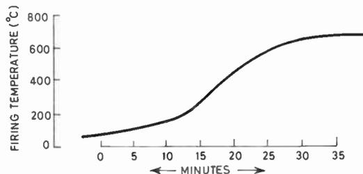
Fig. 3. Typical firing profile for ruthenium resistor glazes.
