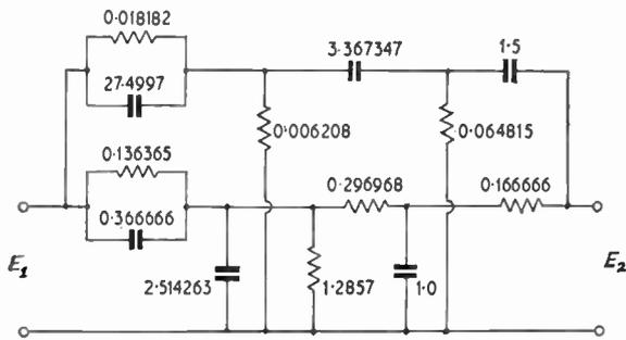
Fig. 2. Third-order rational transfer function network.
