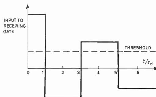
Fig. 5. Oscillations at input of receiving gate.
