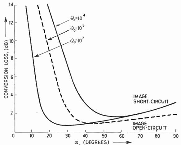
Fig. 11. Conversion loss for narrow-band mixer, using asymmetric diode and additional idler circuit at angular frequencies of  $p+q, 3p-q$  rad/s.
