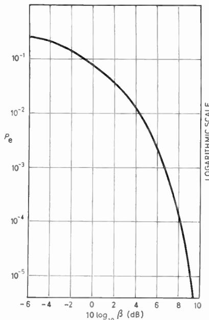
Fig. 2. Error probability in coherent p.s.k. system.
