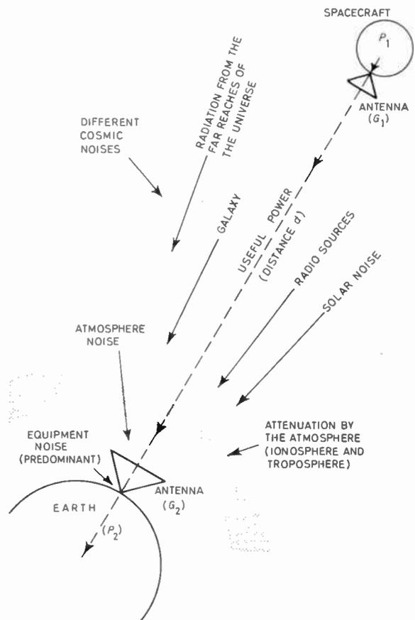
Fig. 1. Diagram of a radio frequency link between Earth and satellite.
