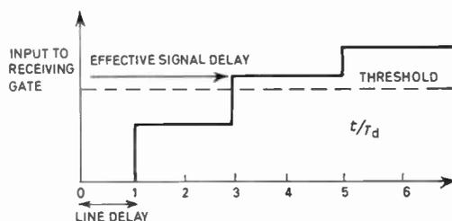
Fig. 4. Increase in signal delay time due to reflections.
