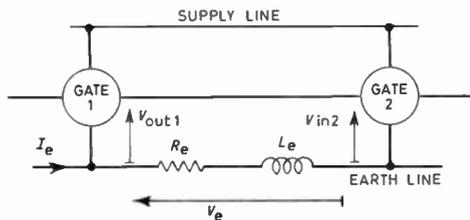
Fig. 6. Cause and effect of earth noise.
