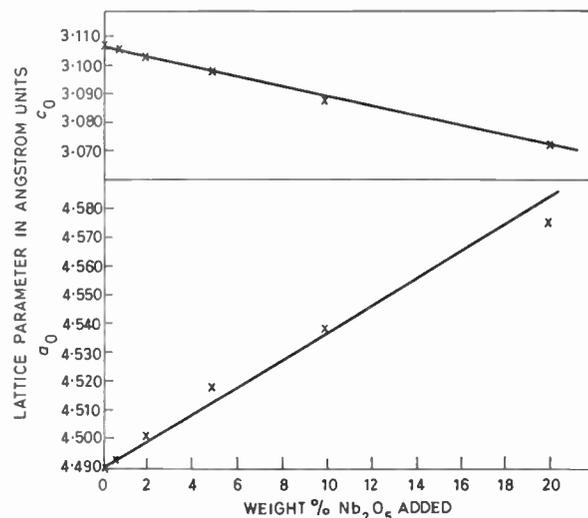
Fig. 1. Effect of additions of  $\text{Nb}_2\text{O}_5$  on the lattice parameters of  $\text{RuO}_2$  showing conformity to Vegard's law.
