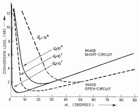
Fig. 8. Conversion loss for narrow-band mixer using asymmetric diode.
