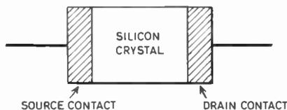
Fig. 1. Structure of s.c.l. diodes.
