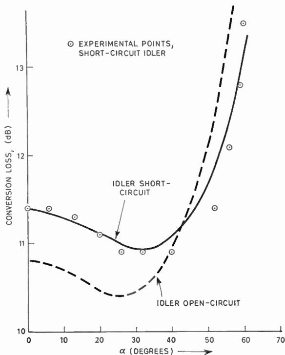
Fig. 5. Symmetrical diode—zero linear conductance.
