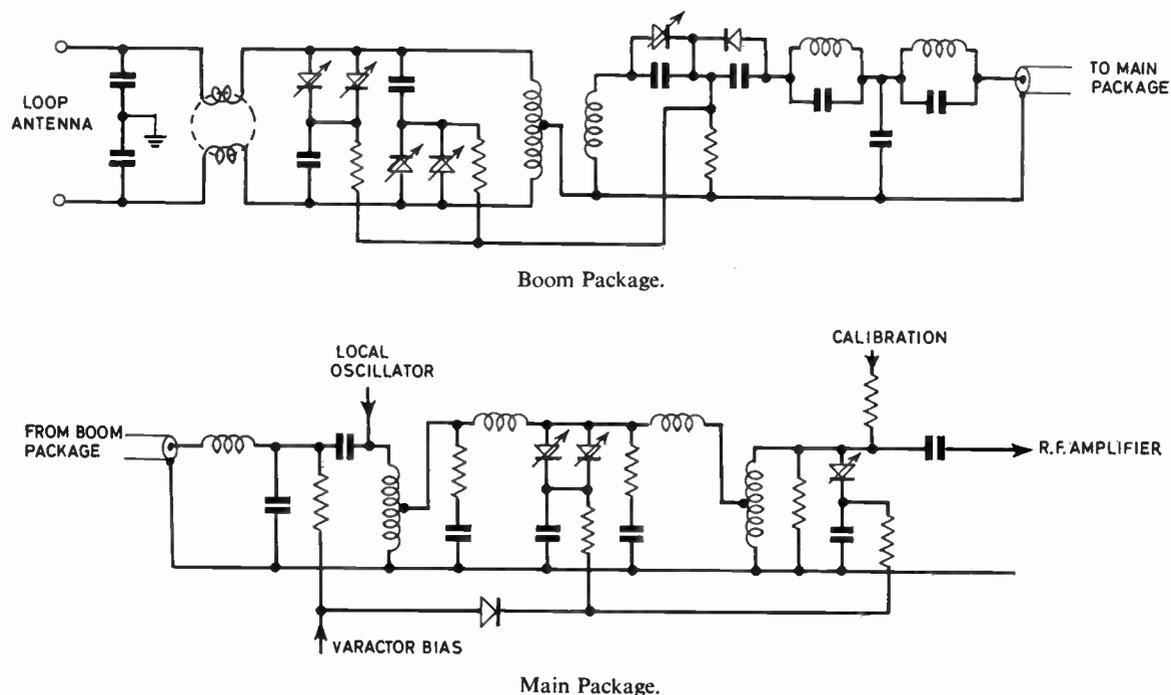
Fig. 2. Circuit diagram of the front end, showing connections between the antenna, the boom unit and the main package.
