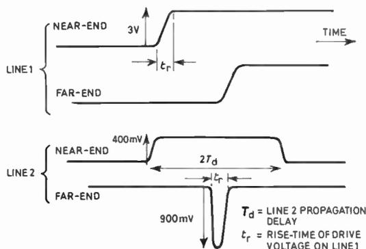
Fig. 3. Typical waveforms for system of Fig. 2, with matched lines.
