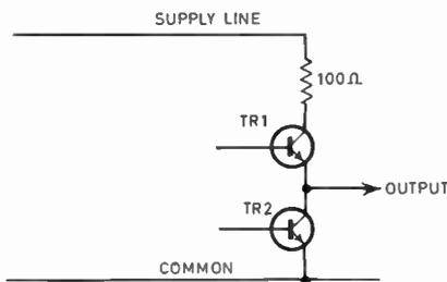
Fig. 7. 'Totem pole' output stage.
