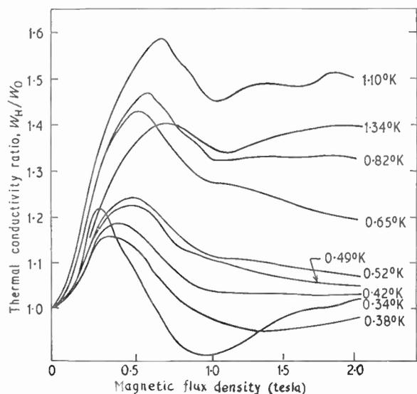
Fig. 3. Variation of thermal conductivity with magnetic field at different temperatures.
