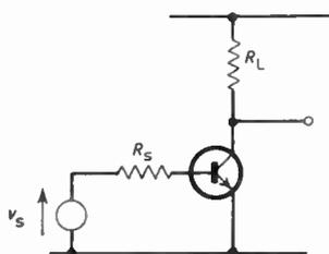
Fig. 3. The common-emitter amplifier.
