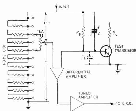
Fig. 4. Bridge circuit for measuring transistor input impedance.
