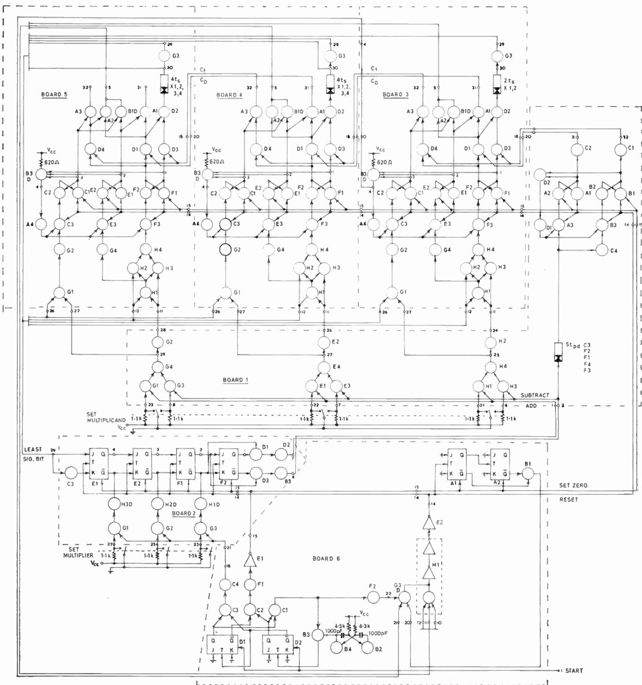
Fig. 3. Experimental asynchronous multiplier.
