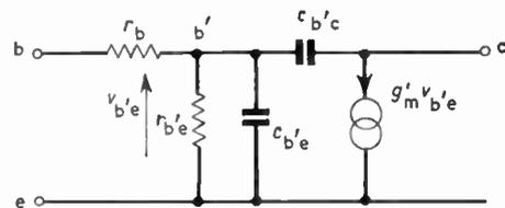
Fig. 2. The hybrid  $\pi$  equivalent circuit of a silicon planar transistor.
