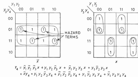
static hazards exist when an input change dictates a transition between internal states in different groupings on the Karnaugh map. For example, the optimum equations for  $Y_3$  are, from Table 4:
