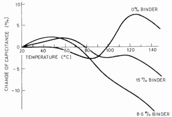
Fig. 5. Variation of capacitance with temperature.
