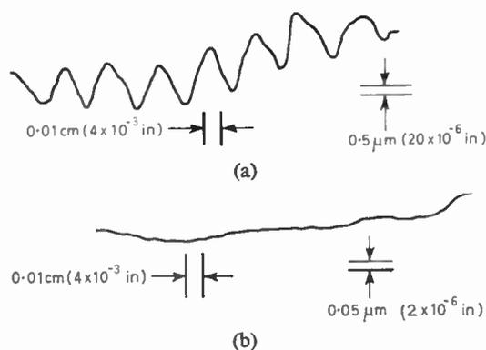
Fig. 6. Typical surface finish of (a) first glaze, (b) second glaze.
