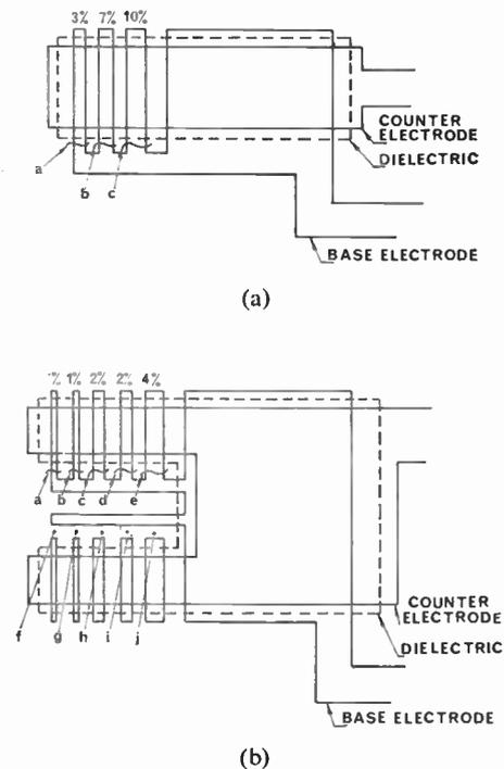
Fig. 3. Adjustable printed glaze capacitors. (Two approaches are shown.)
