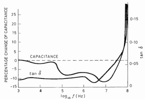
Fig. 7. Variation of capacitance and  $\tan \delta$  with frequency.
