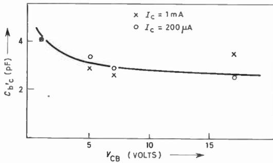
Fig. 7. The variation of collector-base capacitance,  $c_{b'c}$ , with collector-base voltage,  $V_{CB}$ , for a single 2N3707 transistor.
