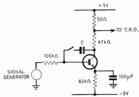
Fig. 1. Test rig for measuring the collector-base capacitance of a transistor.
