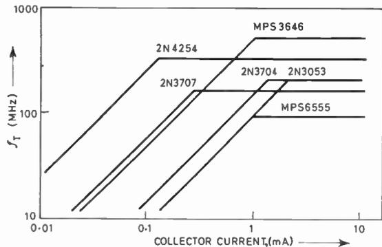
Fig. 9. The variation of transition frequency,  $f_T$ , with collector current for the six transistors of Table 1 (straight line approximation, drawn with logarithmic axes).
