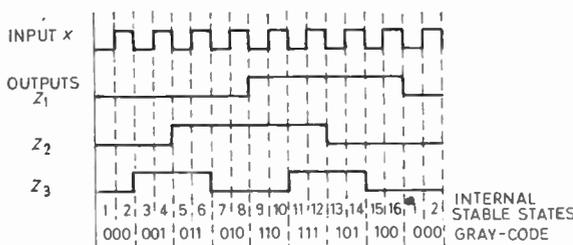
Fig. 2. Timing diagram for Gray-code counter.
