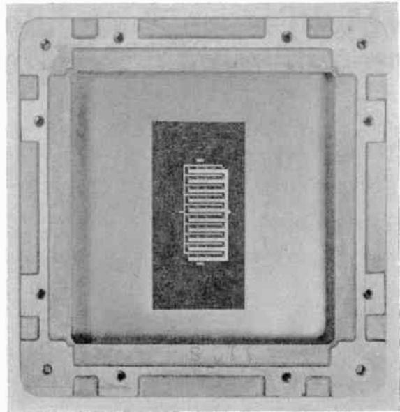
Fig. 2. Etched metal stencil screen.
