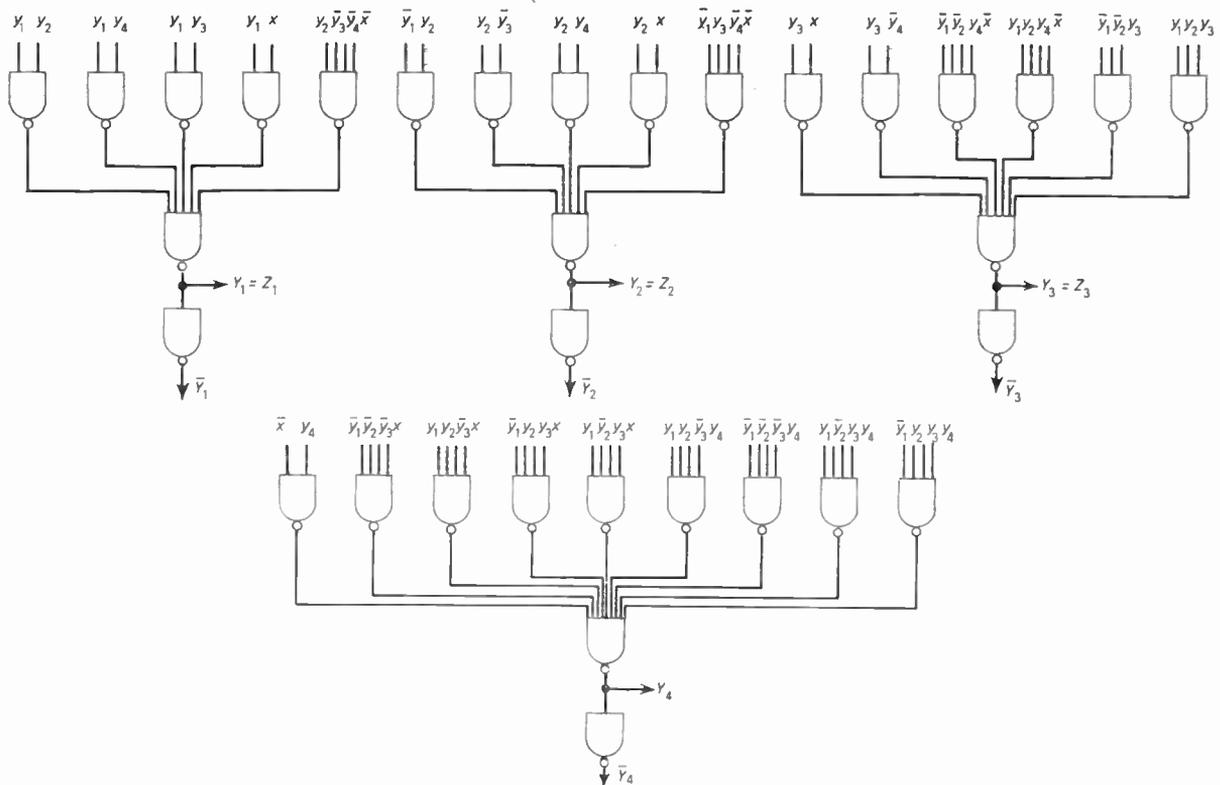
Fig. 3. Implementation of excitation equations for Gray-code counter.
