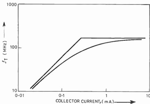
Fig. 8. The variation of transition frequency,  $f_T$ , with collector current  $I_C$  for a typical 2N3707 transistor. The curve is calculated from eqn. (5), and the straight line approximation from its asymptotes.
