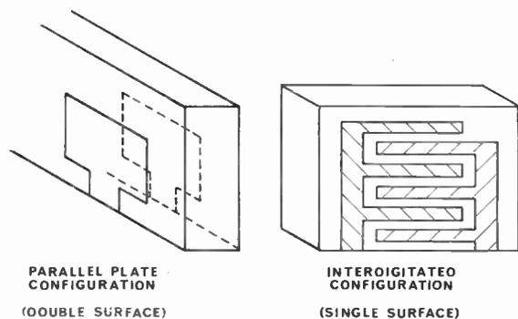
Fig. 1. Electrode configurations on dielectric substrates.
