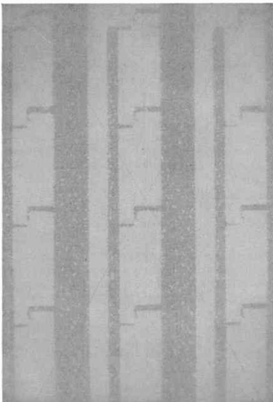
(a) Discontinuous screened gold deposit (magnification  $\times 10$ ).
