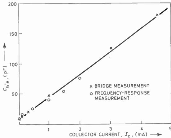
Fig. 5. The variation of base-emitter capacitance,  $c_{b'e}$  with collector current for a single 2N3707 transistor.  $V_{CB} = 5\text{ V}$ .
