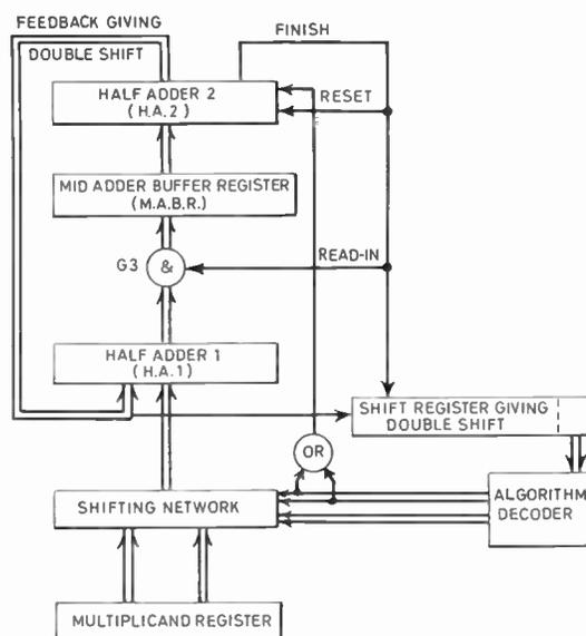
Fig. 2. Multiplier using quaternary algorithm.
