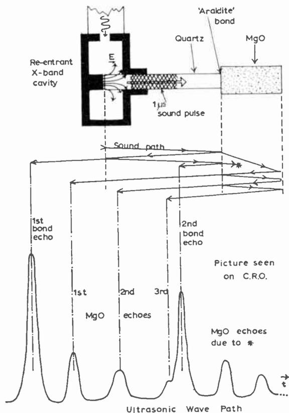
Fig. 1. Re-entrant x-band cavity arrangement.
