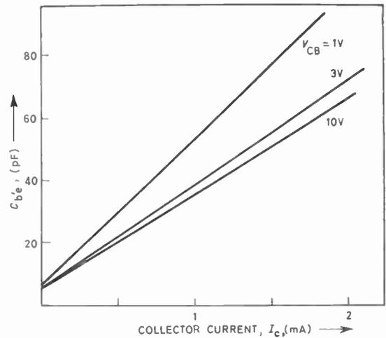
Fig. 6. The variation of  $c_{b'e}$  with  $I_C$  at three values of collector-base voltage. Same 2N3707 transistor as in Fig. 5.
