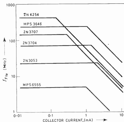
Fig. 10. The variation of  $f_y$ , the corner frequency of  $y_{re}$ , with collector current for the six transistors of Table 1 (straight line approximation, drawn with logarithmic axes).
