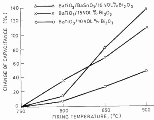
Fig. 4. Variation of capacitance with dielectric firing temperature.
