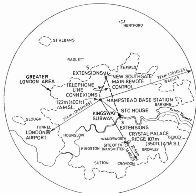
Fig. 8. Coverage map for u.h.f. mobile system with 12.5 kHz channel spacing.
