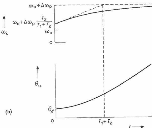
Fig. 10. Frequency and phase drift during field sync.
