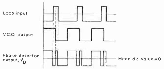
Fig. 3. Phase detector operation.
