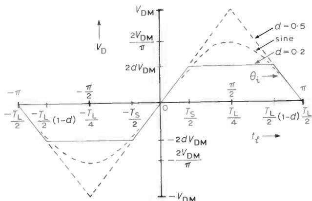
Fig. 5. Phase detector sensitivity.
