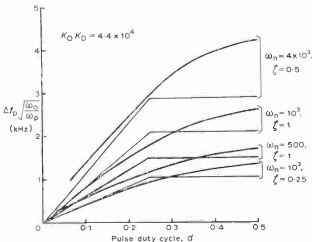
Fig. 15. Experimental data compared with pull-in approximation. As a reasonable design equation we then use, for
