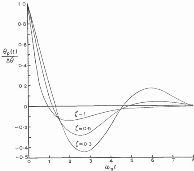
(a) Phase error  $\theta_p(t)$  due to a step in phase  $\Delta\theta$ .
