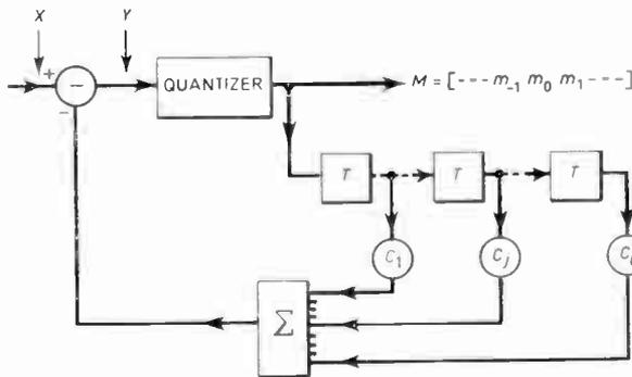
Fig. 5. Quantized-feedback correction.
