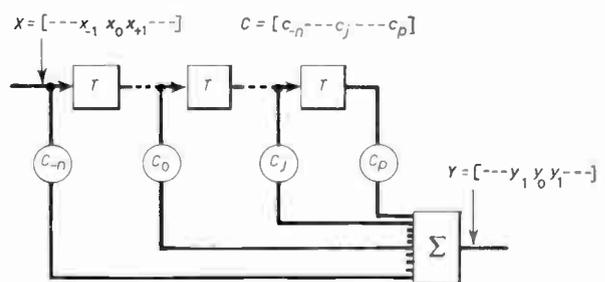
Fig. 4. Linear non-recursive transversal network.
