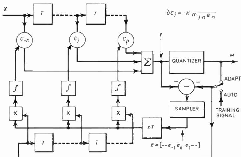
Fig. 6. Zero-forcing adaptive equalization.
