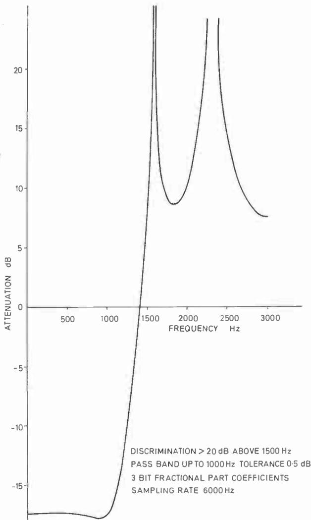
Fig. 4. Frequency response of a low-pass filter.
