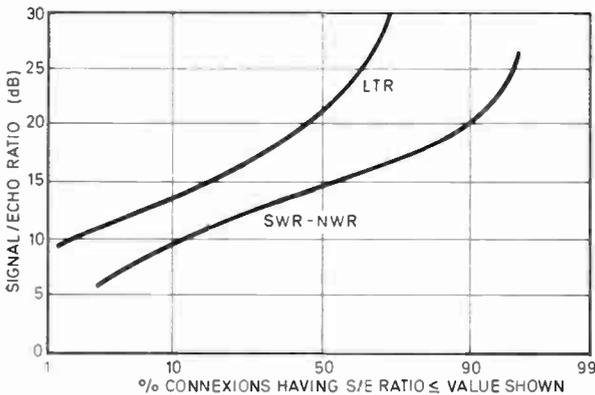
Fig. 3. Cumulative distribution of signal/echo ratio.
