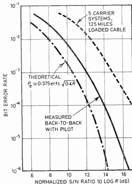
Fig. 11. Noise performance of modem.
