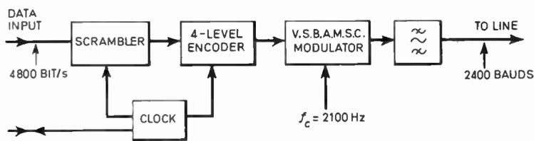
Fig. 9. An experimental adaptively equalized modem.
