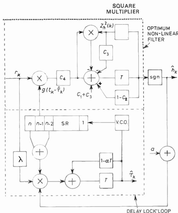
Fig. 1. Signal-flow diagram based on eqns. (12), (17).
