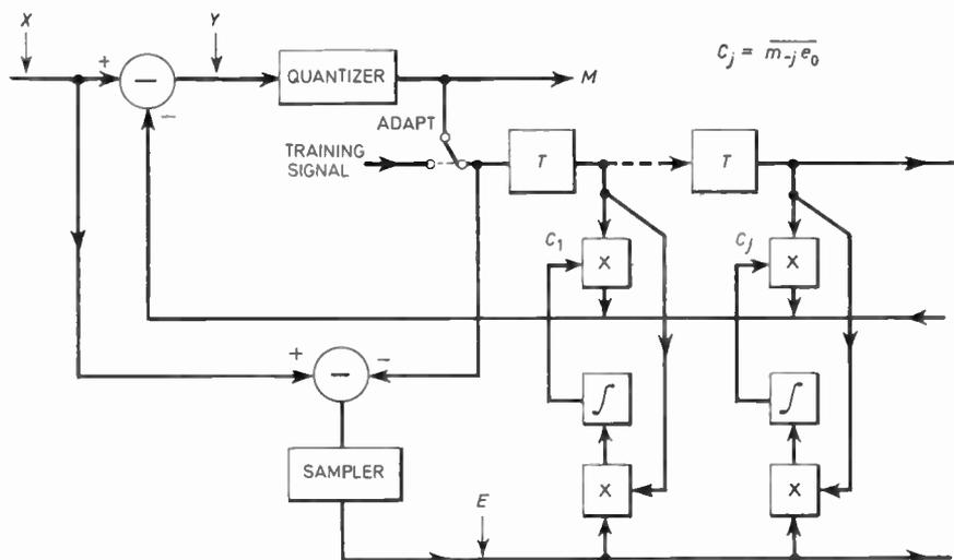
Fig. 8. Quantized-feedback coefficient.
