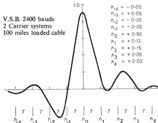
Fig. 2. Measured pulse response.
