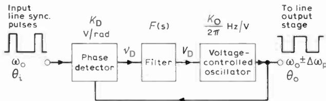
Fig. 1. The phase-locked loop system.
