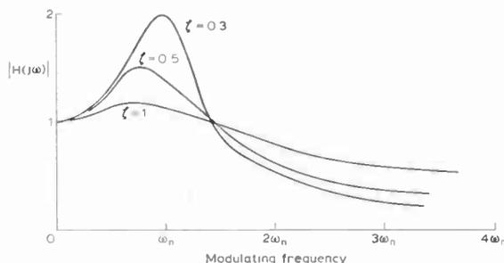
Fig. 6. Loop frequency response.
