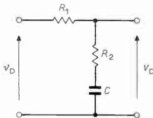
Fig. 2. The loop filter.
