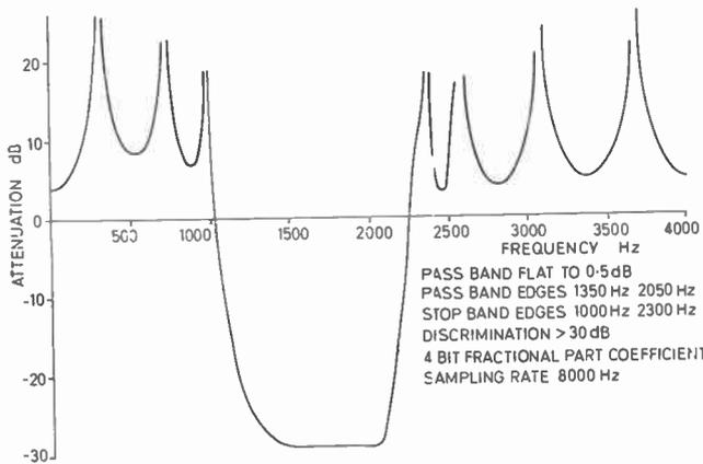
Fig. 6. A band-pass characteristic.
