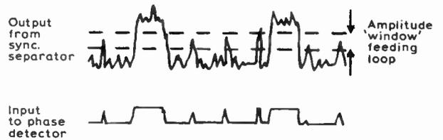
Fig. 9. Noise limiting at the loop input.
