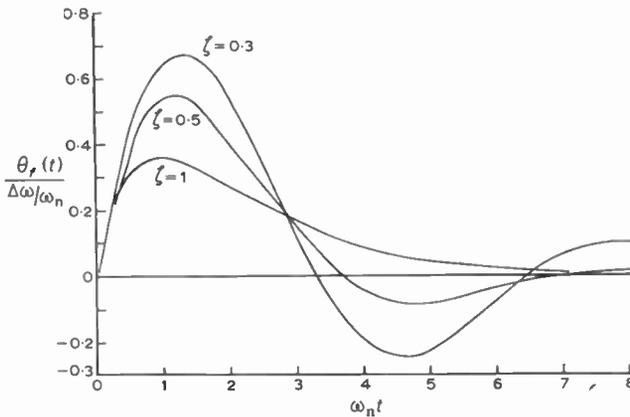
(b) Phase error  $\theta_f(t)$  due to a step in frequency  $\Delta\omega$ .
