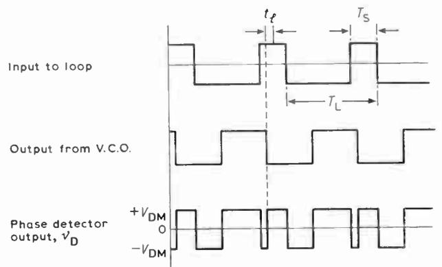
Fig. 4. Phase detector operation with a timing error,  $t_l$
