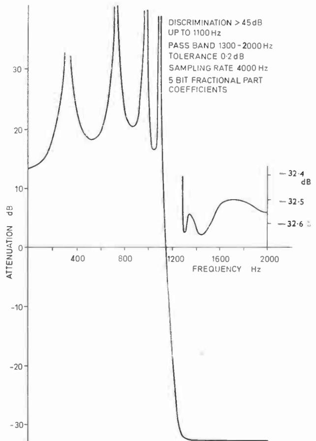
Fig. 5. Frequency response of a high-pass filter.
