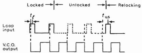
Fig. 11. V.C.O. frequency drift during field sync.
