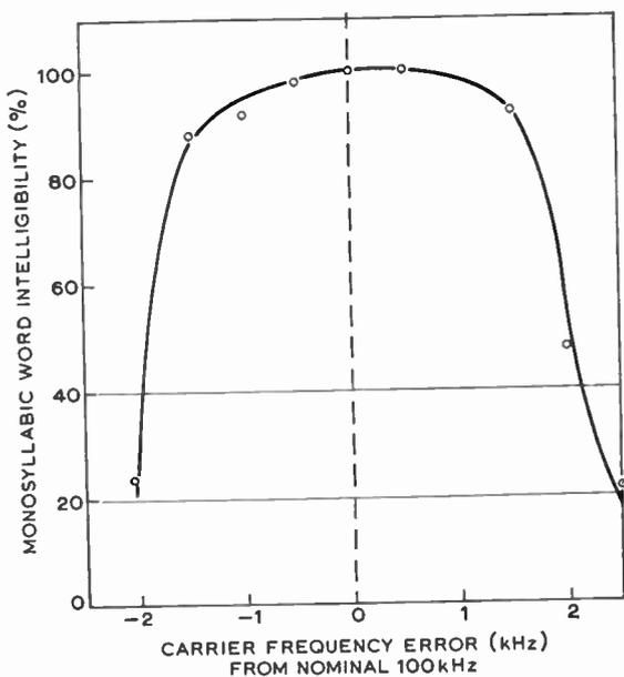
Fig. 4. Intelligibility of detector using 2F coil (Pinches, M. C., Private communication).
