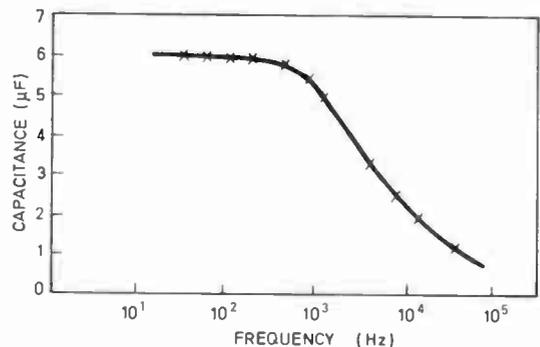
Fig. 21. Capacitance versus frequency for computed and experimental results on porous anode tantalum capacitor (after Morley<sup>14</sup>).
