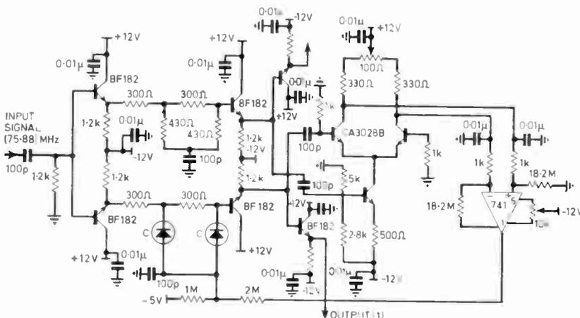
Fig. 4. A servo-controlled phase delay network producing equal amplitude quadrature outputs in the frequency range 66-100 MHz.
