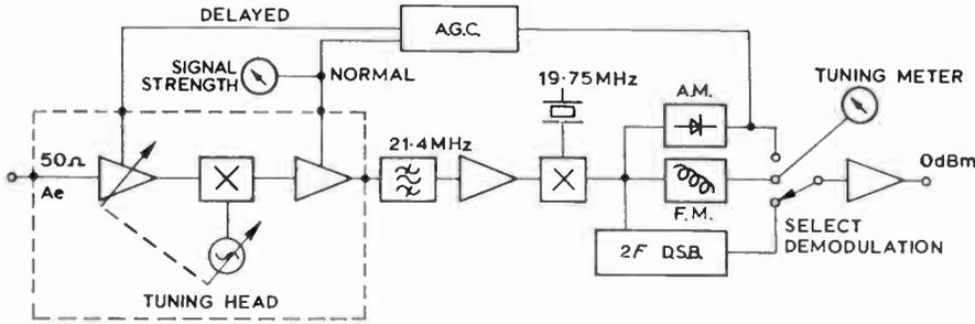
Fig. 1. Experimental receiver schematic.
