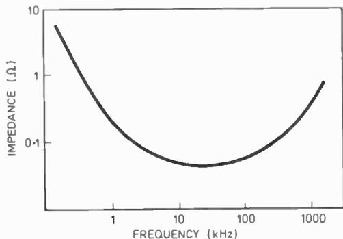
Fig. 6. Impedance versus frequency for 150 μF, 20 V capacitor (85°C).
