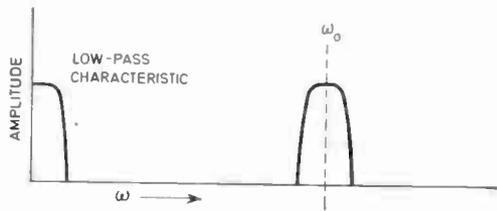
Fig. 2. Low-pass filter characteristic and the corresponding band-pass filter characteristic of the Barber receiver.
