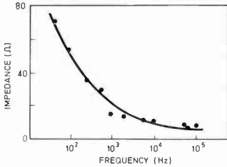
Fig. 19. Dispersion effects in electrolyte (300 Ω cm material).
