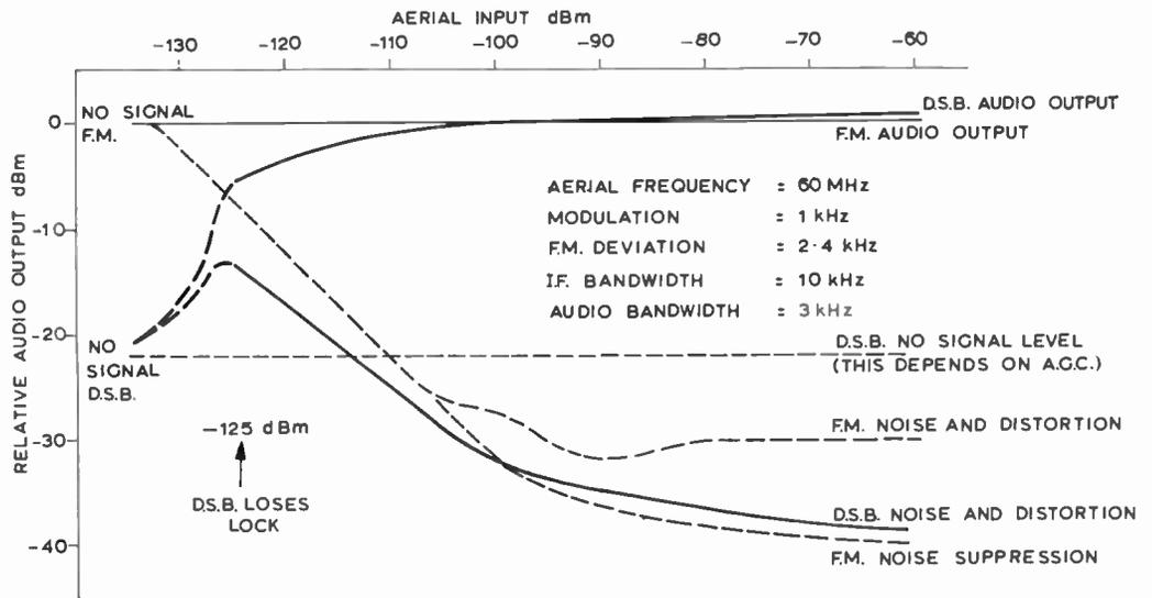
Fig. 11. SINAD performance of ACL receiver for d.s.b., f.m. and a.m.
