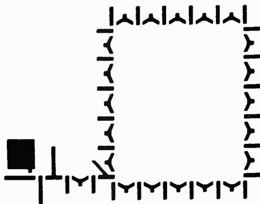
Fig. 1. Simple Y-bar shift register.
