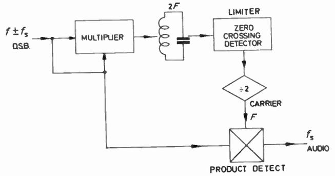
Fig. 3. Coil 2F d.s.b. demodulator.
