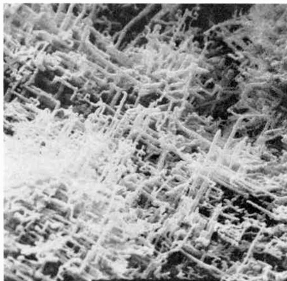
Fig. 7. Etched structure in aluminium foil. Anodized to 20 V (length of edge 40 μm).
