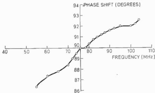
Fig. 5. Phase shift as a function of frequency for the SCPDN of Fig. 4.
