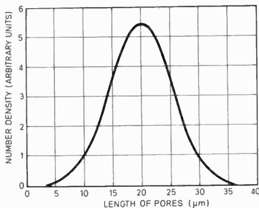
Fig. 9. Distribution of tunnel lengths for a practical low voltage foil (see Fig. 7).
