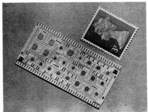
**Fig. 7.** Hybrid circuit module containing 23 integrated circuits.
