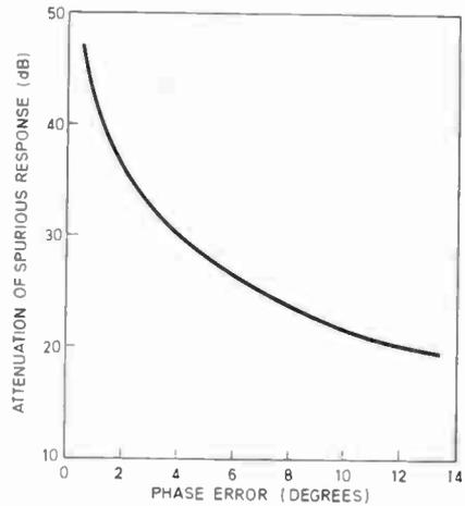
Fig. 3. Relationship between spurious response and total phase error of the quadrature oscillators.
