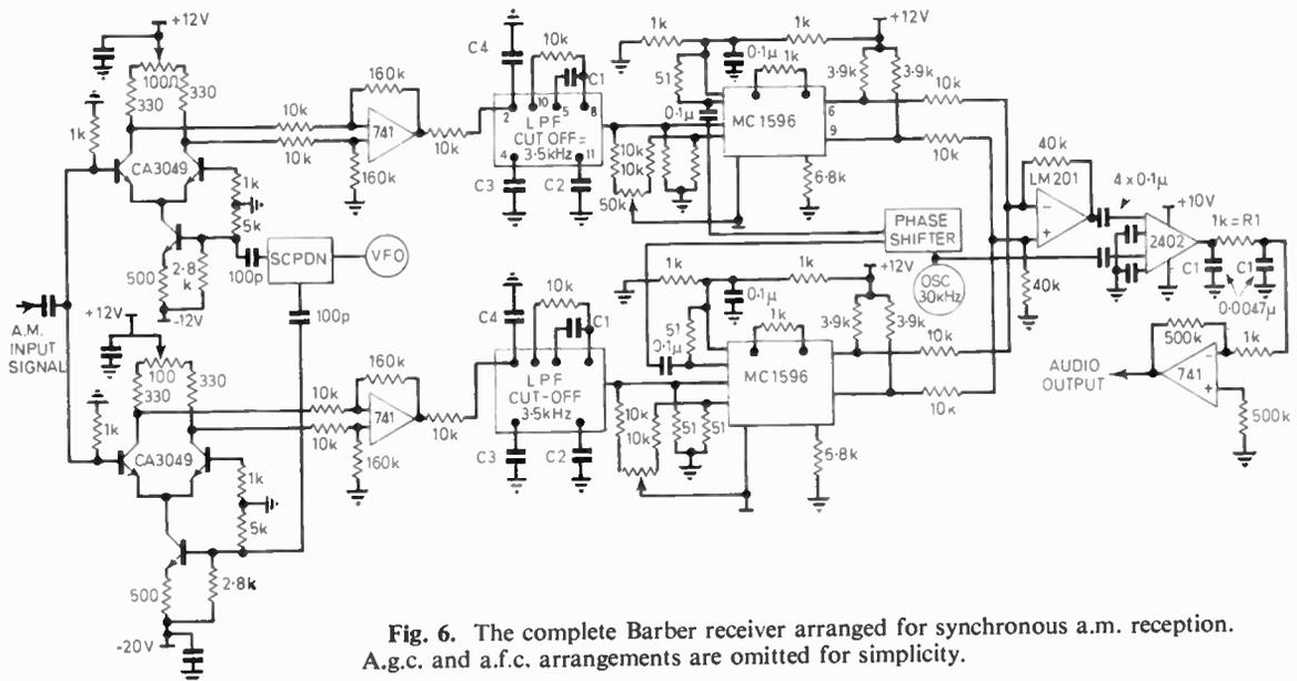
Fig. 6. The complete Barber receiver arranged for synchronous a.m. reception. A.g.c. and a.f.c. arrangements are omitted for simplicity.
