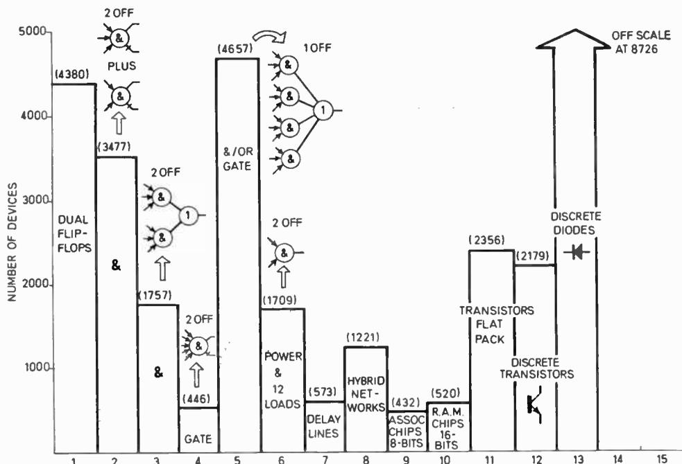
Fig. 2. *MU5* device types (excluding memory systems over 1k words (32 bits) capacity).
