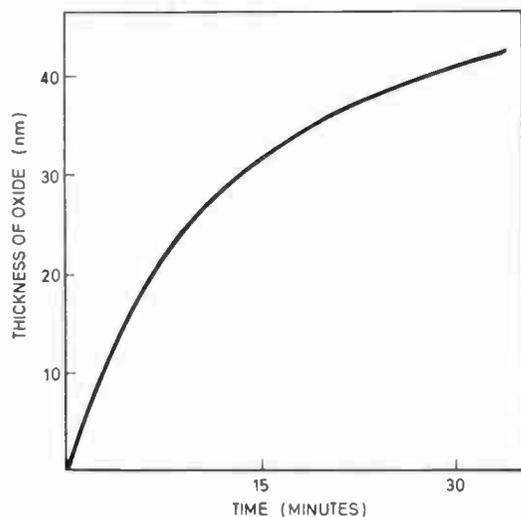
Fig. 3. Constant voltage growth of film of alumina on aluminium surface as a function of time (30 V applied).
