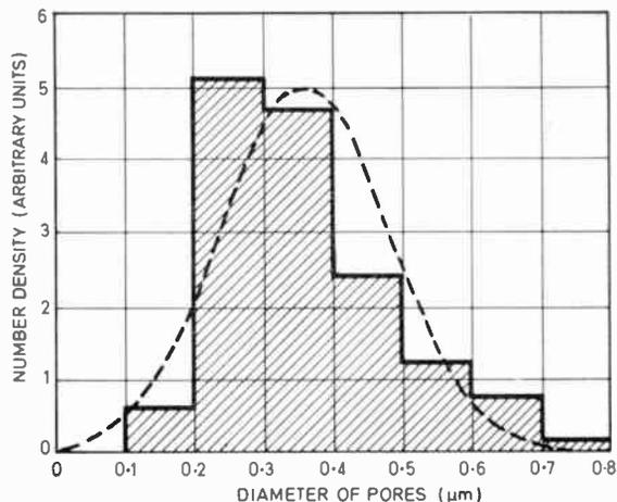
Fig. 8. Distribution of tunnel diameters for a practical low voltage foil (see Fig. 7).
