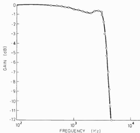
Fig. 7. Characteristic of 4th order low-pass filter used in Fig. 6.
