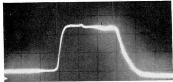
Fig. 3. (a) Waveform of detected output pulse from p-i-n diode gate, when the duration of the gating signal corresponds to the time delay around the waveguide ring. The time scale of the oscilloscope picture corresponds to 10 ns/cm.
