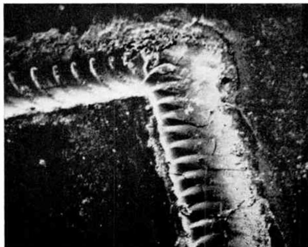
Fig. 8. Corner of rectangular pattern in epitaxial garnet.
