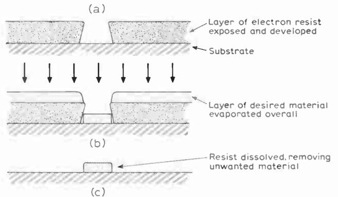
Fig. 5. Stages in the 'lift-off' process.
