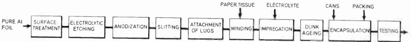
Fig. 1. Block diagram showing the preparation of an aluminium electrolytic capacitor.
