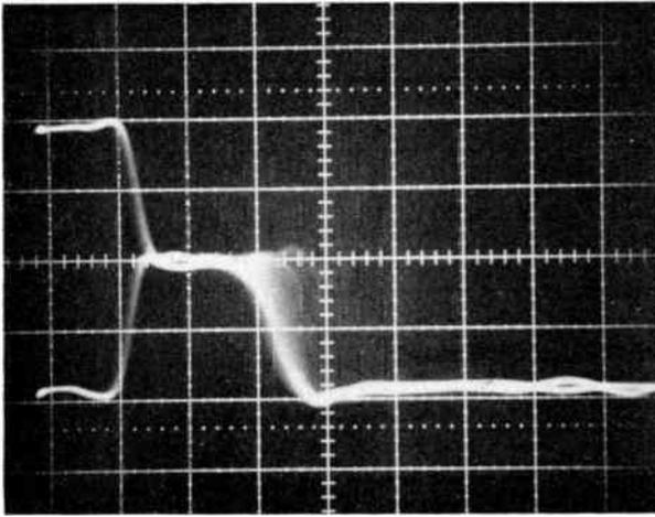
Fig. 5. E.c.l. flip-flop settling time.
