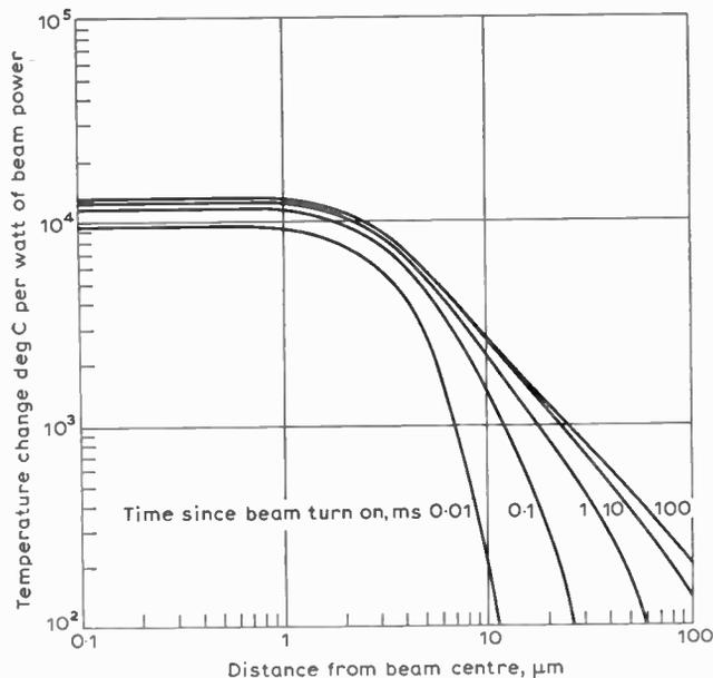
Fig. 6. Surface temperature rise for various exposure times of incident electron beam power.
