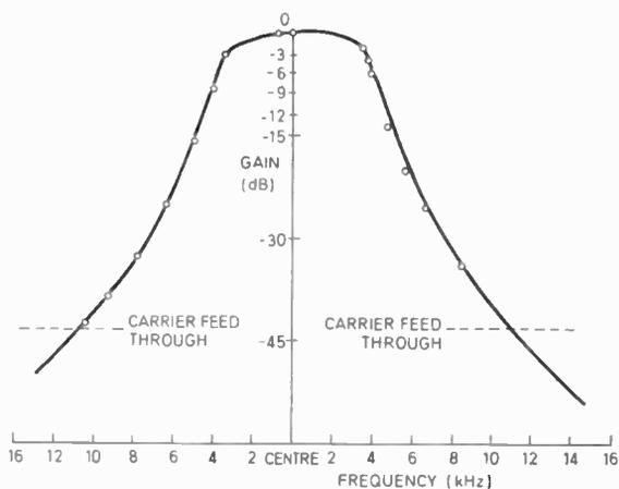
Fig. 8. Receiver selectivity curve. Centre frequency in the range 66–95 MHz.
