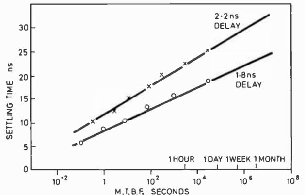
Fig. 6. Performance of e.c.l. flip-flops.
