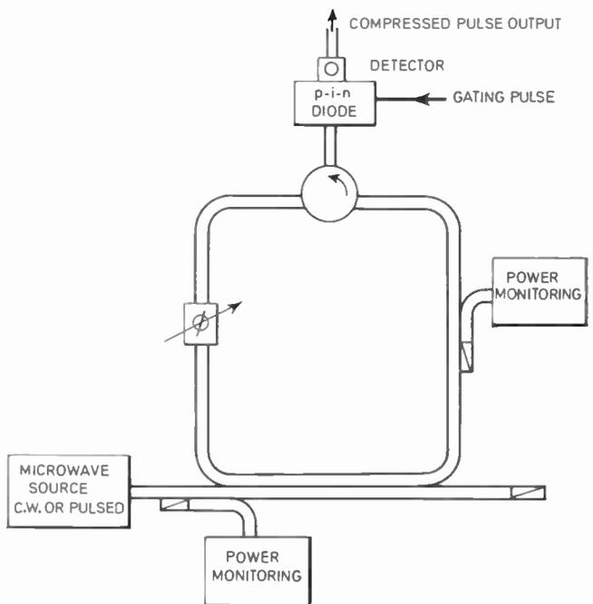
Fig. 1. Schematic diagram of experimental waveguide ring assembly with circulator and p-i-n diode gate.
