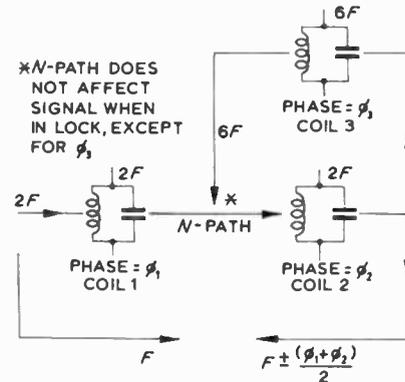
Fig. 7. The tuned components in the  $N$ -path demodulator.
