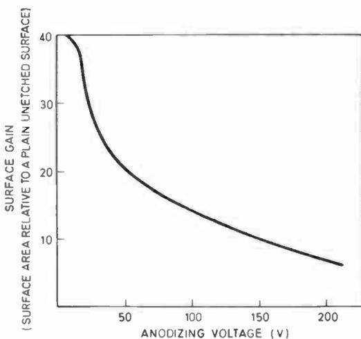
Fig. 2. Relationship between surface gain and anodizing voltage (for a low voltage type of foil etch).
