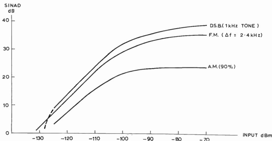
Fig. 12. Signal distortion improvement because of coherent demodulation.
