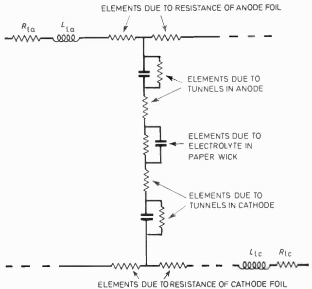
Fig. 17. Total transmission line equivalent of capacitor.
