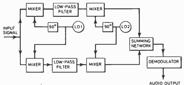
Fig. 1. The basic Barber receiver.
