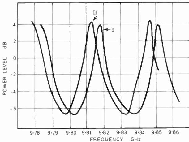
Fig. 2. Frequency response of resonant ring assembly. (0 dB represents input power level.)
