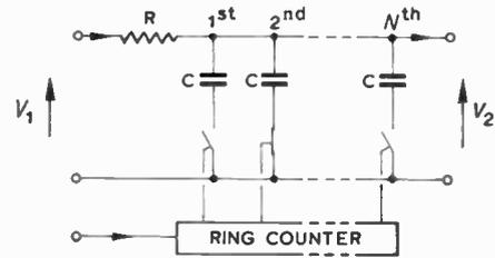
Fig. 5. Basic properties of  $N$ -path filter.
