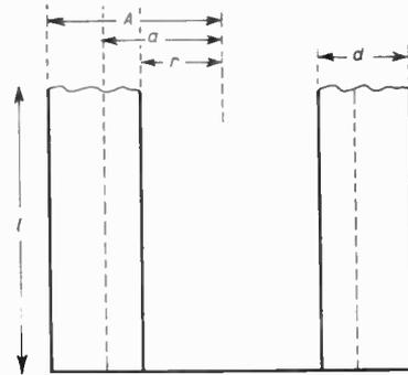
Fig. 10. Diagram of tunnel structure showing dimensions before and after anodization.
