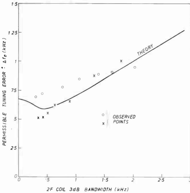
Fig. 15. Variation of tolerable carrier frequency error with 2F circuit Q-factor.
