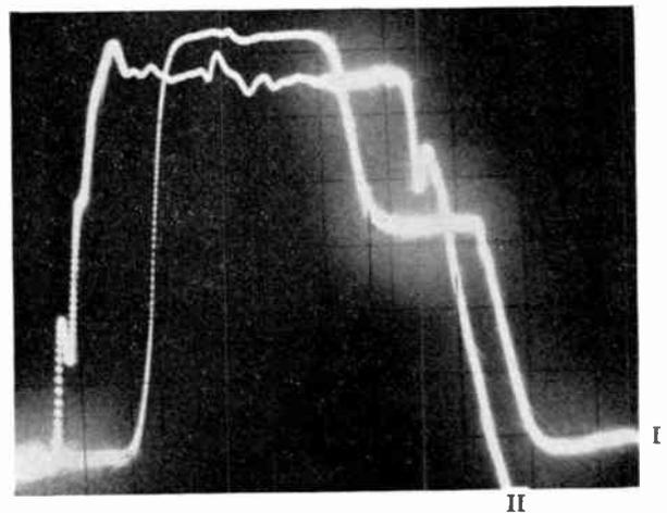
Fig. 3. (b) Waveform of the output detected pulse (waveform I) and of the gating pulse to the p-i-n diode (waveform II) when the diode gate is left open beyond the time delay around the ring. The time scale of the oscilloscope picture corresponds to 10 ns/cm.
