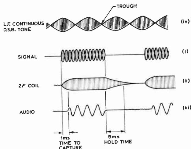
Fig. 8. Observed capture and hold time for demodulator.
