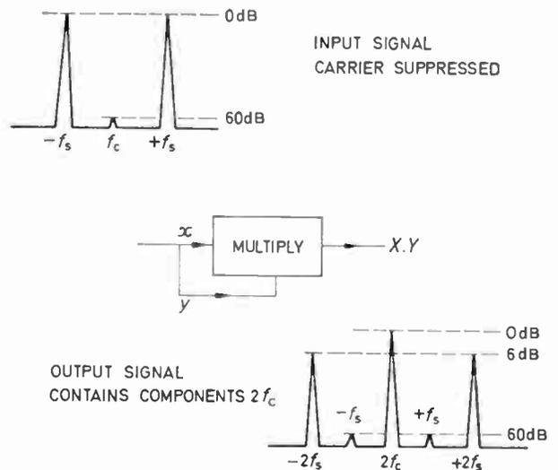
Fig. 2. The frequency doubling process.
