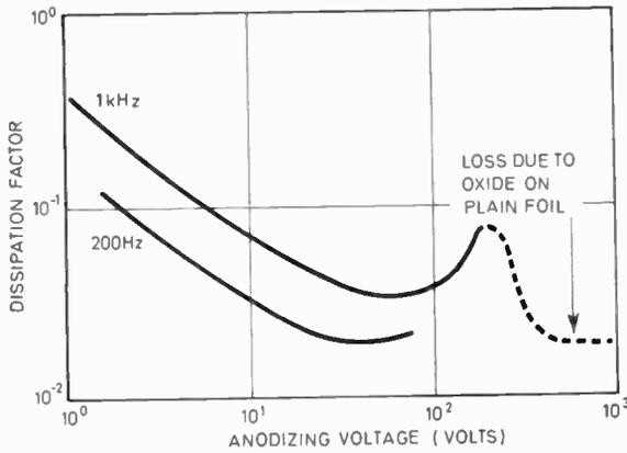
Fig. 15. Dissipation factor versus anodizing voltage for two frequencies.
