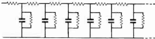
Fig. 11. Equivalent transmission line representation of a single tunnel.
