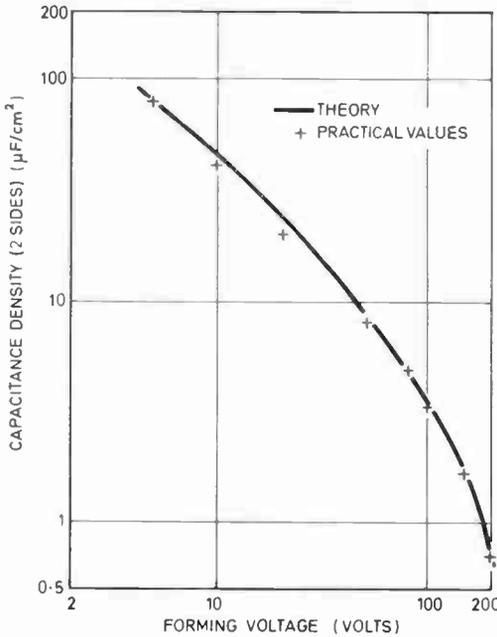
Fig. 13. Capacitance/unit area as a function of forming voltage (theory and practice).
