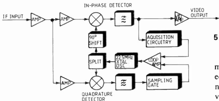
Fig. 4. Synchronous detector block diagram.
