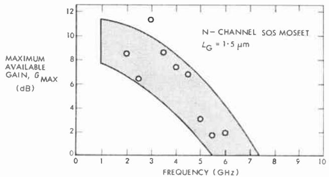
**Fig. 5. Gain versus frequency for n-channel s.o.s. m.o.s.f.e.t. showing cut-off frequency = 6.4 GHz.**
