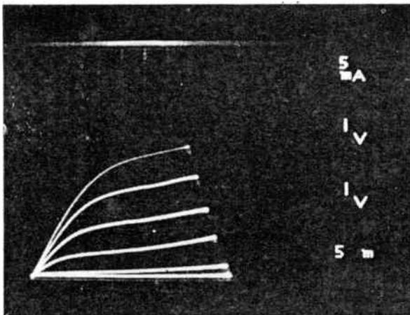
**Fig. 3. S.o.s. m.o.s.f.e.t. characteristics.**
