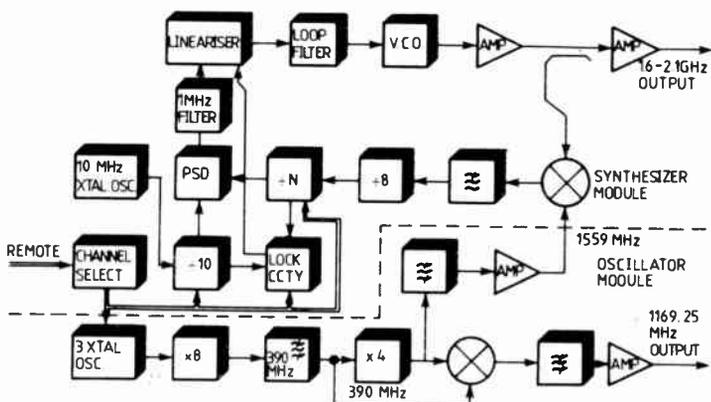
Fig. 3. Synthesizer block diagram.
