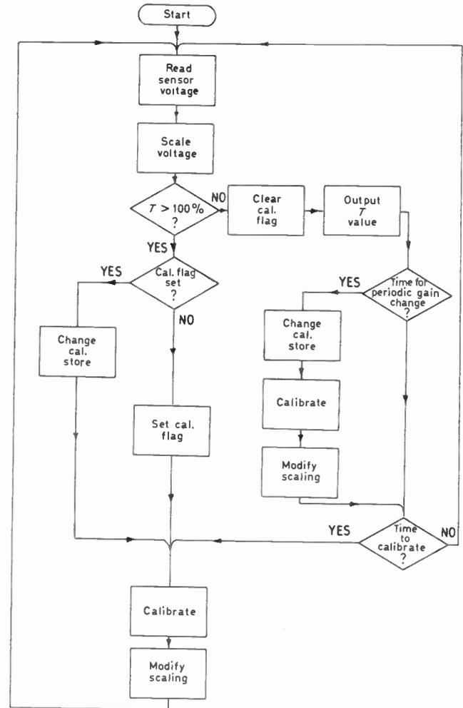
Fig. 15. MET-1 processor flow diagram.
