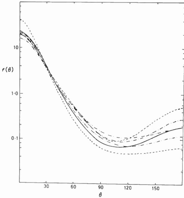
Fig. 3. Scattering functions for a visual range of 1 km (taken from reference 12).
