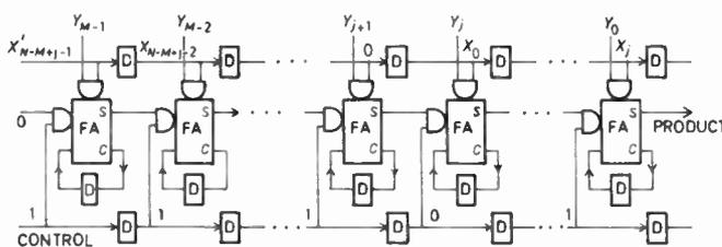
Fig. 1. The serial-pipeline multiplier for positive numbers.
