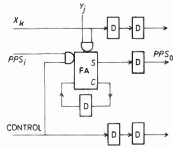
Fig. 2. The rudimentary cell of a pipeline multiplier.
