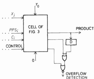
Fig. 6. The overflow detection circuit for  $|Y| < 2$  and in sign-magnitude representation.
