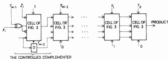
Fig. 7. The full multiplier for  $|Y| < 2$  and in sign-magnitude representation, including the capability to generate the function  $(X + Z)Y$ .
