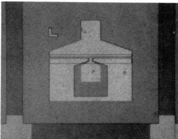
**Fig. 2. Silicon-on-sapphire m.o.s.f.e.t. device geometry.**
