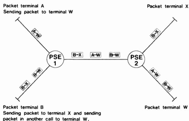
Fig. 3. Principles of packet switching.
