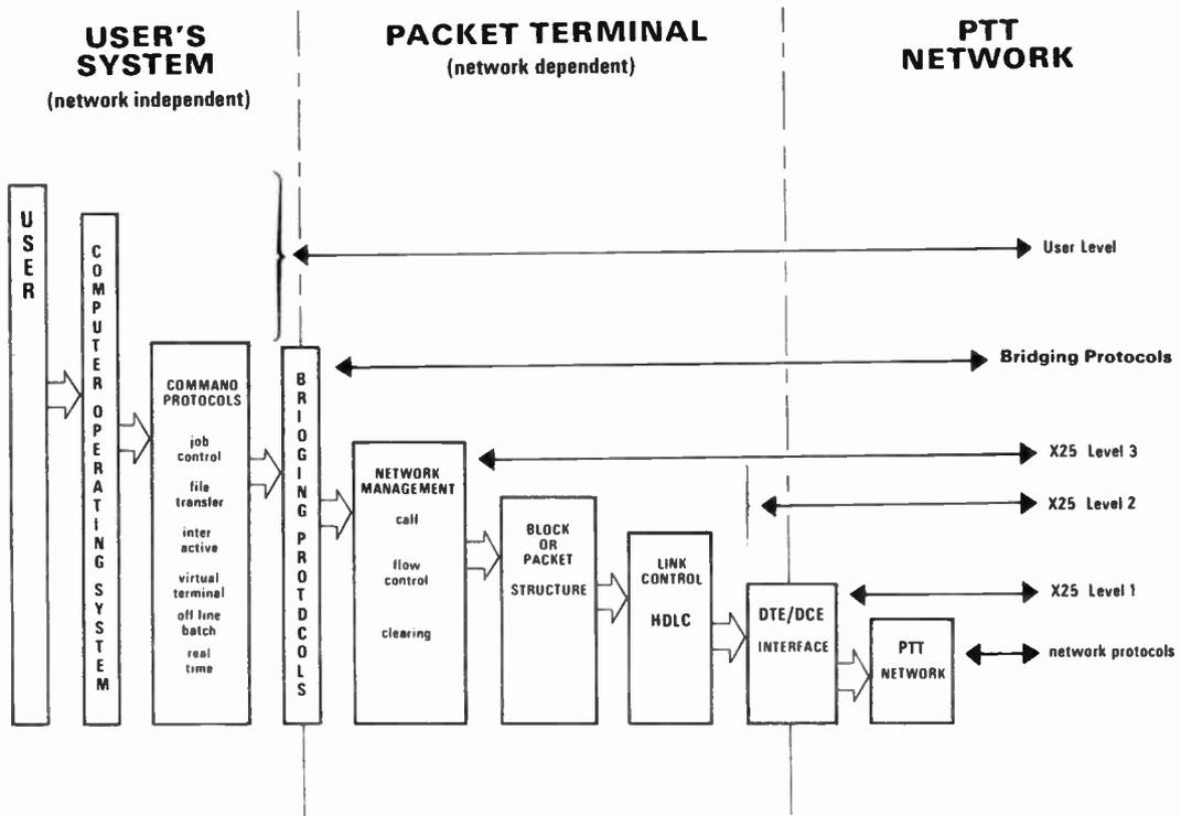
Fig. 5. Protocols for packet-mode terminals communicating via the network.
