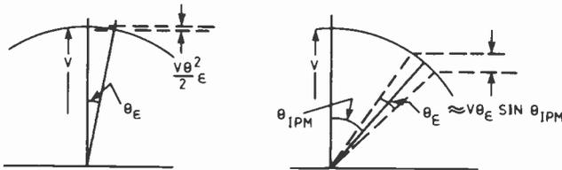
(a) Effect of phase deviation. (b) Effect of incidental phase modulation.
