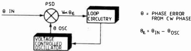
Fig. 6. Phase locked loop.
