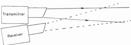
Fig. 4. Backscatter device showing sample of atmosphere defined by overlap of transmitted beam with receiver field view.
