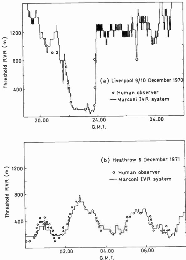
Fig. 12. Comparison of visibility data from Marconi IVR system and human observers.
