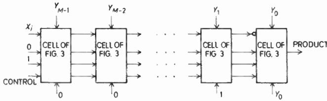
Fig. 4. The two's complement pipeline multiplier for  $|Y| < 1$ .
