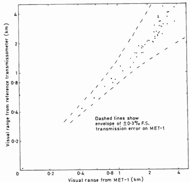
Fig. 17. Comparison of visual range data from MET-1 and reference transmissometer; 6th January 1977-8th January 1977.
