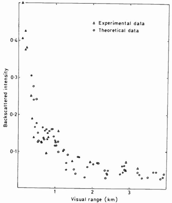
Fig. 5. Correlation between backscatter and visual range (taken from reference 14).
