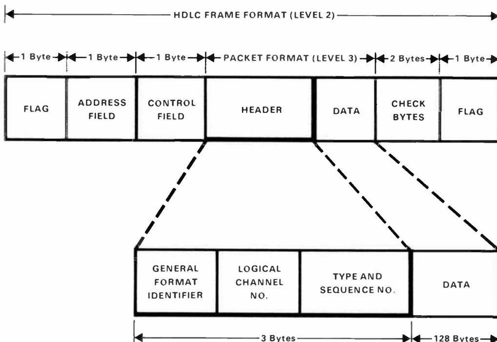
Fig. 2. Frame and packet structure.
