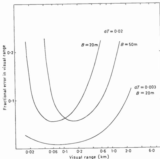
Fig. 7. Visual range error as a function of visual range for various transmissometer baselines and full scale errors.
