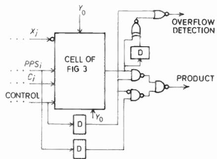
Fig. 5. The last stage for a coefficient with  $|Y| < 2$  and in two's complement representation.
