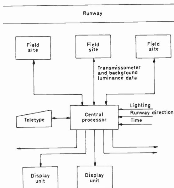
Fig. 9. Block diagram of three field site RVR system.
