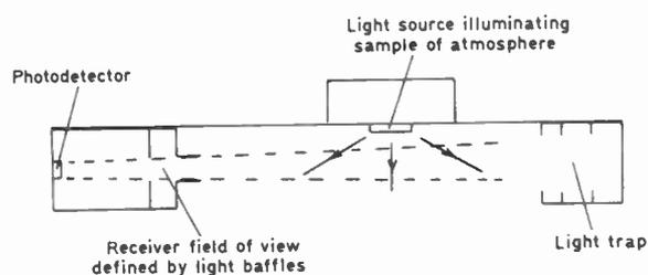
Fig. 2. General principles of an integrating nephelometer.
