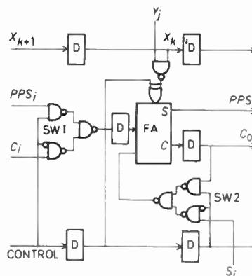
Fig. 3. The proposed two's complement multiplier cell.
