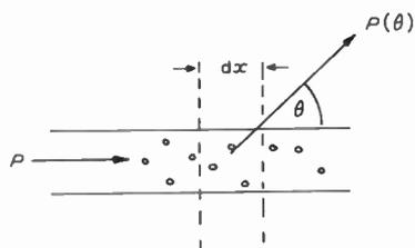
Total power scattered per unit length of beam  $\frac{dP}{dx} = P \cdot \sigma_{sc}$
