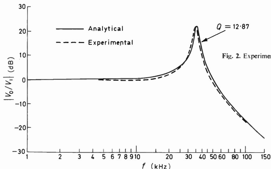
Fig. 2. Experimental and analytical plots of the inverting lowpass filter.
