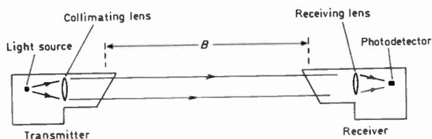
(a) Double ended, measurement path  $B$
