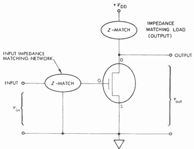
**Fig. 4. Silicon-on-sapphire transistor high frequency test.**
