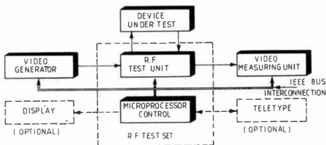
Fig. 8. Comprehensive transmitter/transposer maintenance equipment.
