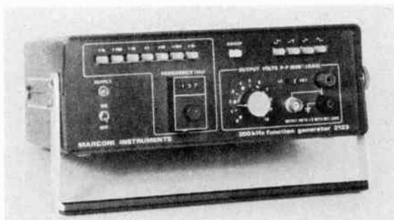
Marconi Instruments multi-purpose waveform generator 2123
