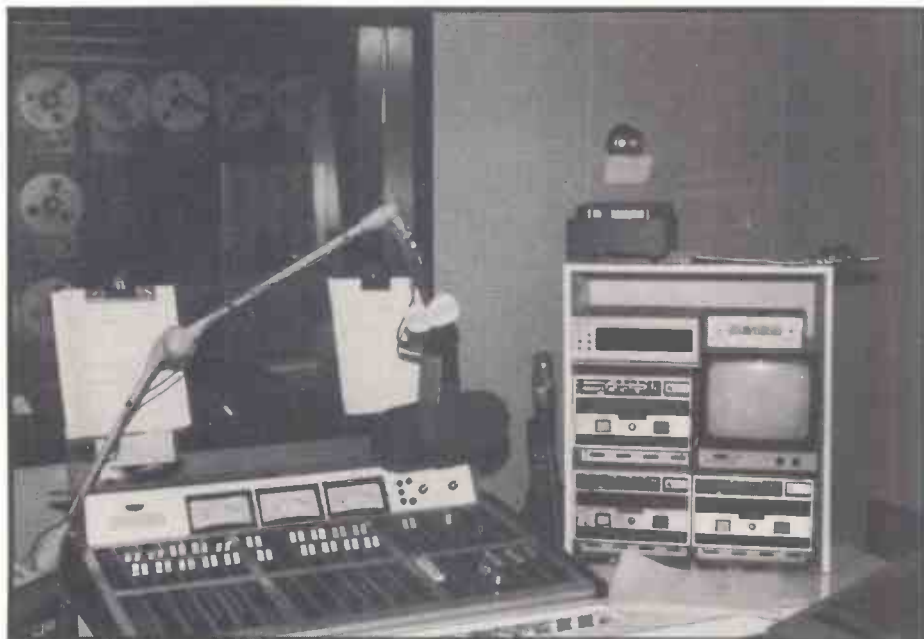
FM on-air/production studio with automation rack in the background
