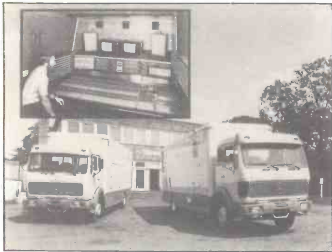
NOS OB vehicles. Inset: interior view with Neve 8108 console.
