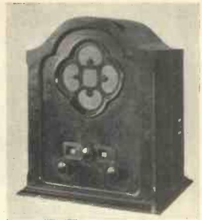
Five valves, excluding the rectifier, are employed in an unorthodox circuit in this Edison Bell set.
