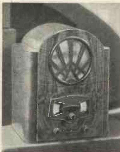
The Lumophon W.23 receiver is notable for its use of "direct coupling" which is stated to be very efficient.
