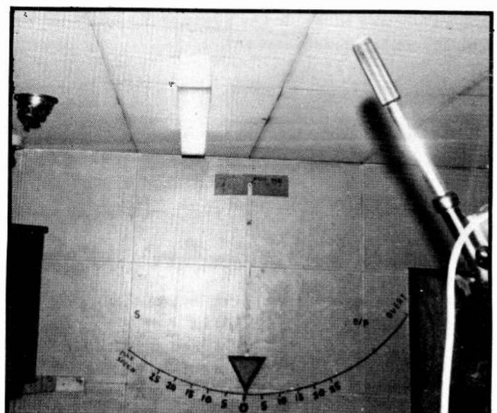
The "swingometer" denoting how far the Mebo II is rolling.
