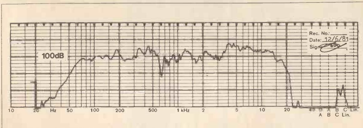
Figure 1. Response chart for Studio 12L & HF250 Crossover HPX4 taken at 1 watt/1 metre in the anechoic chamber. (The dip in response at 600kHz is due to the very small 1½ cu. ft. cabinet used in the test.)
