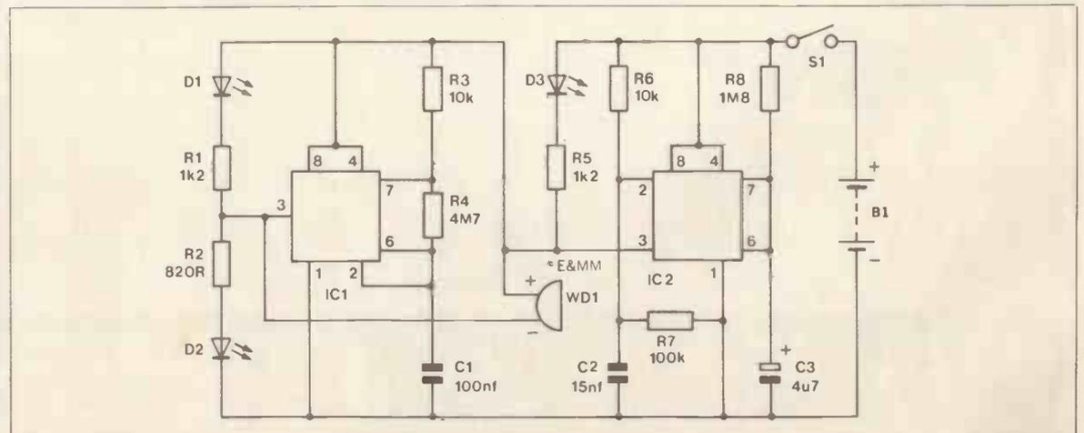
Figure 1. Car Race Starter circuit diagram.
