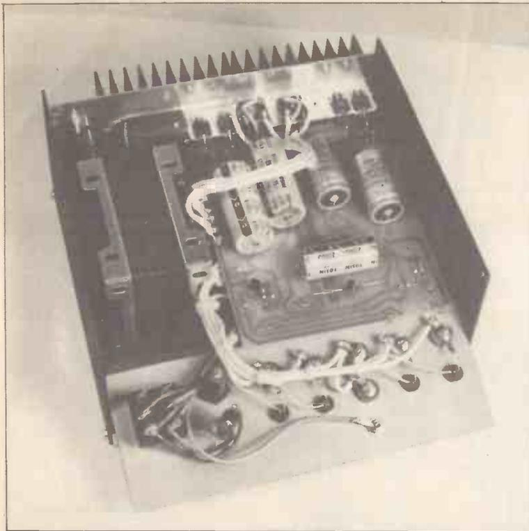
Completed power supply showing internal layout.
