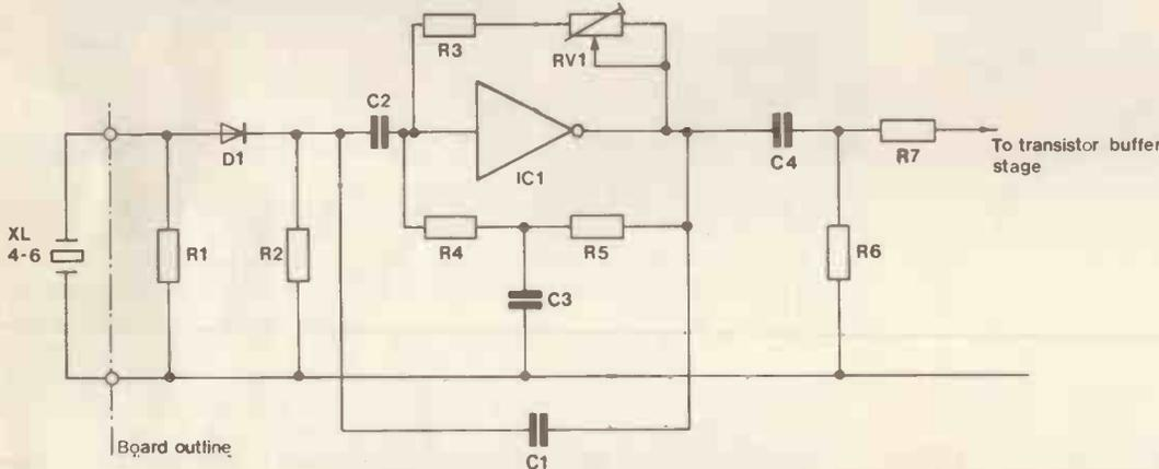
Figure 2(c). Circuit for lower-range drums.
