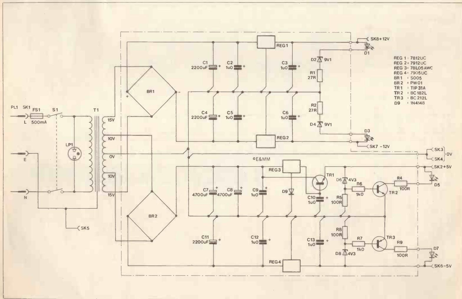
Figure 1. The power supply circuit.
