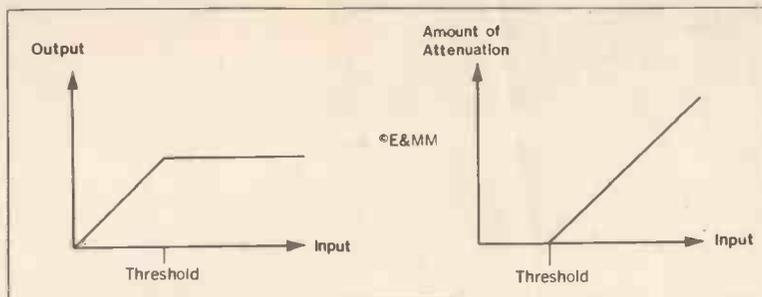
Figure 2. Ideal limiter characteristics.
