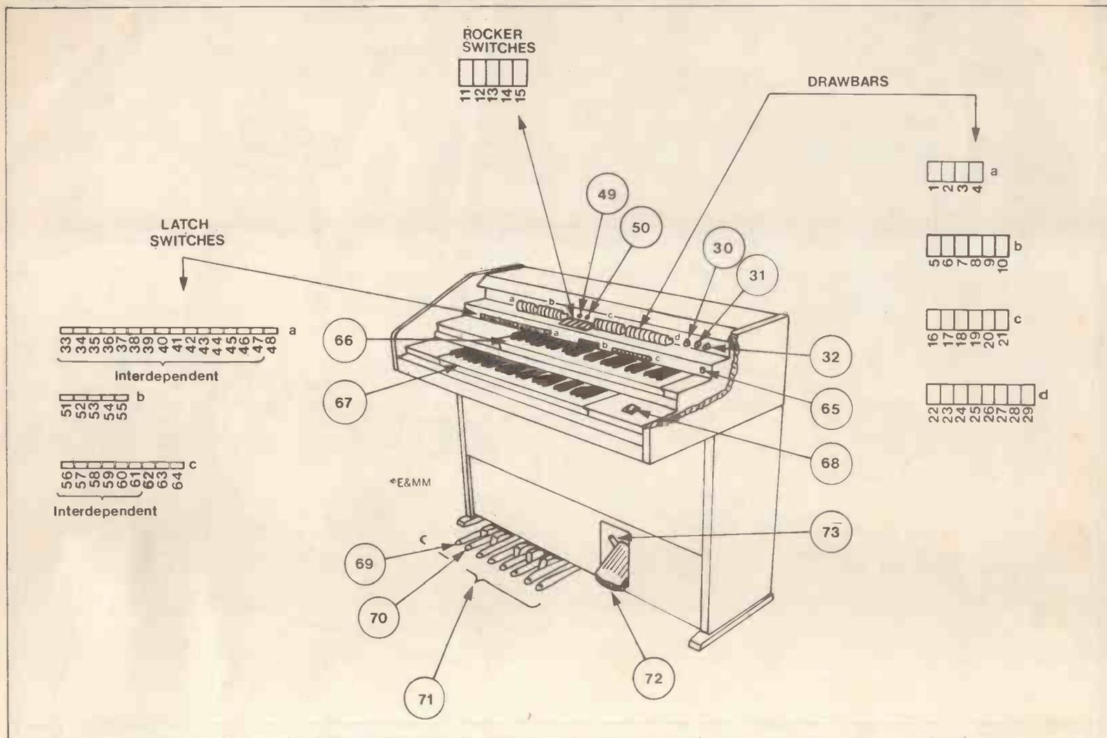
Figure 47. Layout of controls.
