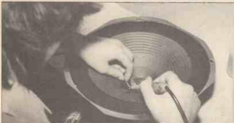
Soldering wire connections to cone.
