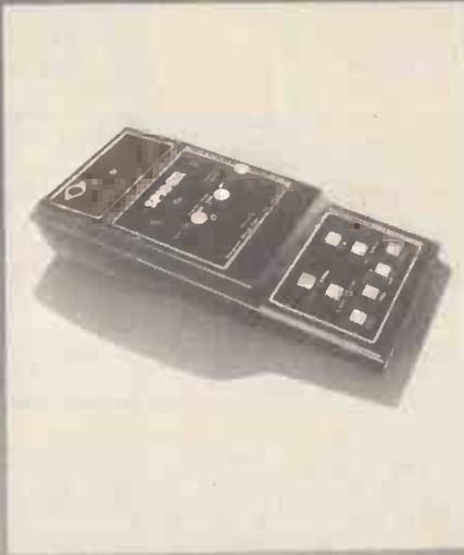
(£199 inc. VAT) A digital micro computer based sequencer designed for use with the Gnat and the Wasp synthesisers. Two modes of operation—
