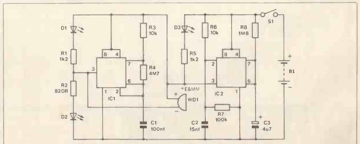
Figure 1. Car Race Starter circuit diagram.
