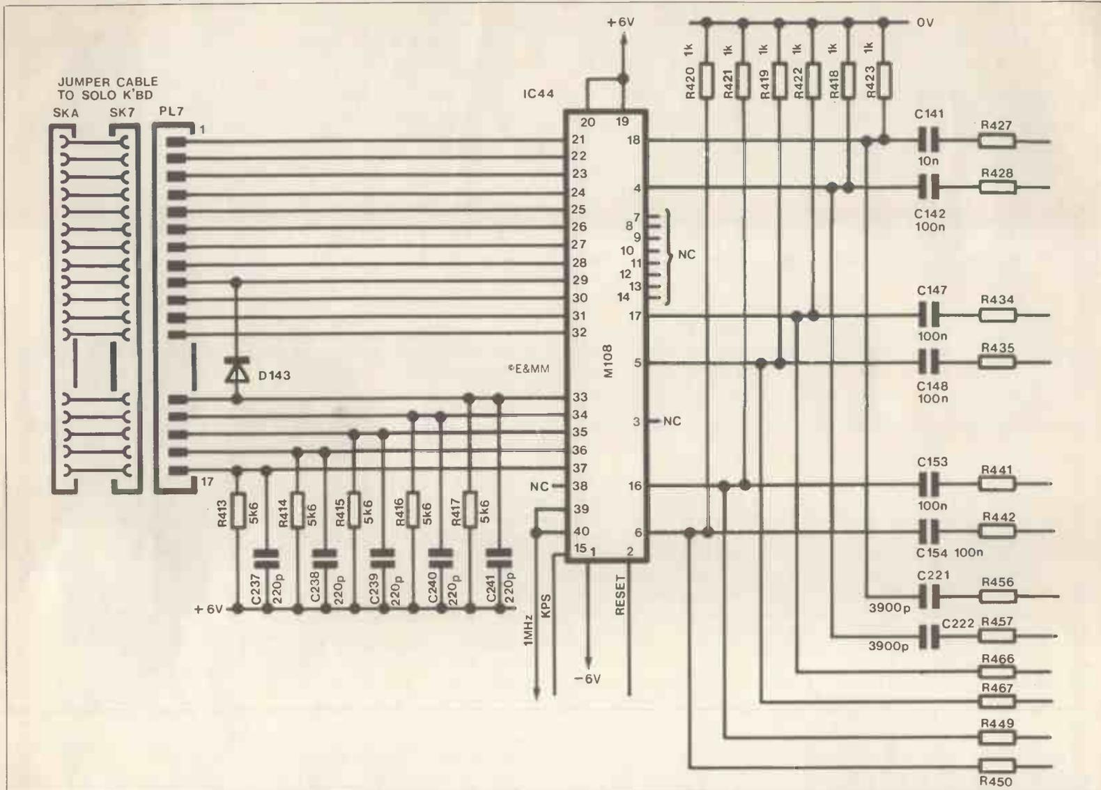
Figure 48. Amended upper manual M108 circuit.
