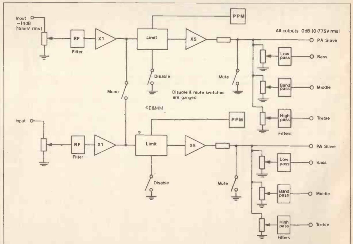
Figure 1. PA Signal Processor block diagram.
