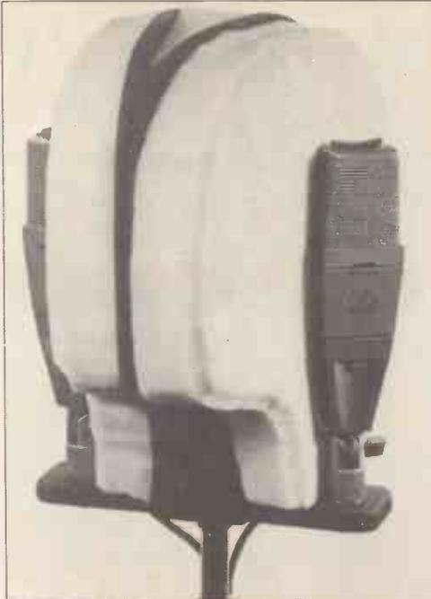
Figure 4. Omni mics baffled from each other for 'dummy head' binaural. Sennheiser MKE203 Electret Capacitor (left) and AKG C414 Capacitor set to omni.
