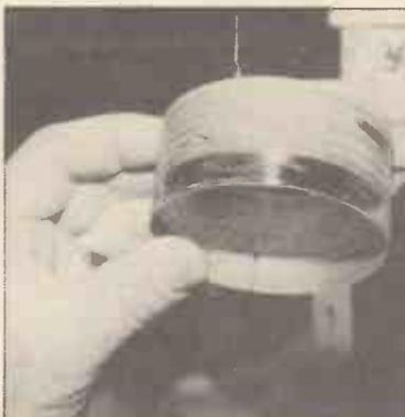
Completed voice coil on glass-fibre former.
