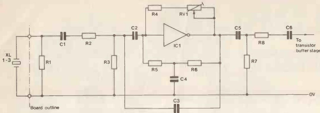
Figure 2(a). Circuit of upper range drums.
