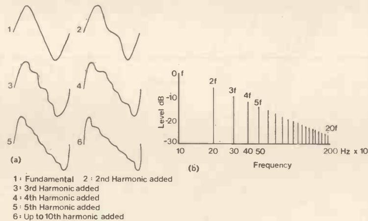
Figure 3. (a) Synthesis of sawtooth (ramp) wave, showing number of harmonics present. (b) Harmonic composition of sawtooth wave.
