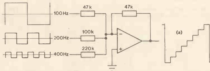
Figure 4. Op-Amp circuits giving (a) 'staircase' and (b) square wave.
