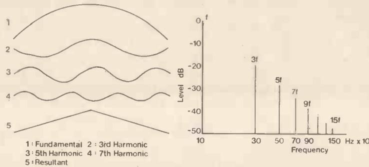
Figure 1. Frequency spectrum of triangle wave, showing harmonic content.
