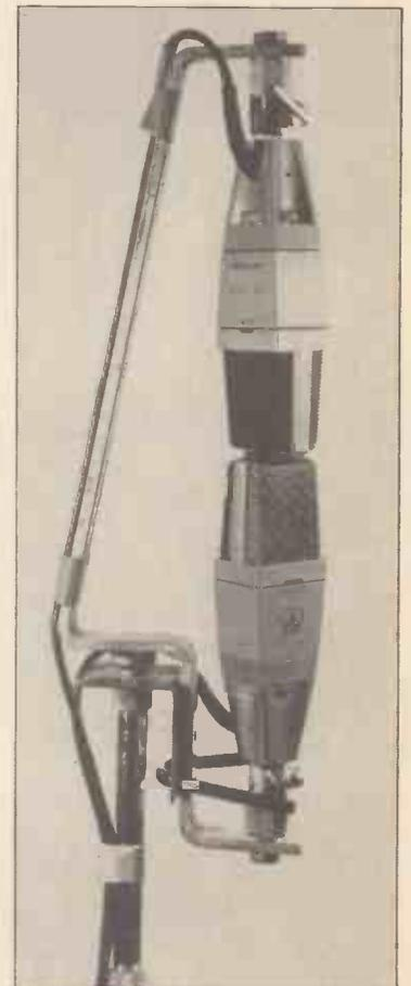
Figure 3. Crossed 'coincident' pairs. Shown above is AKG C414 Capacitor (switched to Cardioid or Hypercardioid or even 'figure of eight'), and below: Calrec CM652 Cardioid Capacitor pair.
