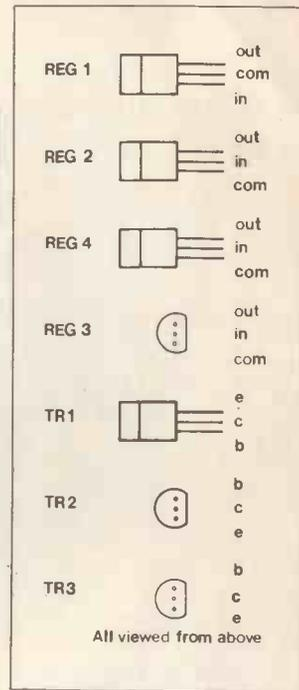
Regulator and transistor pin connections.
