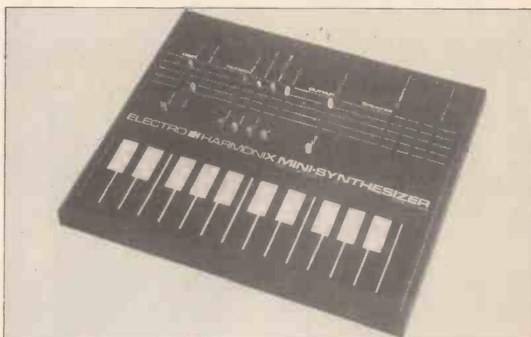
**ELECTRO-HARMONIX MINI-SYNTHESIZER (MODEL EH0400).** The Mini-Synthesizer is attractively presented in a light weight, slim, black case and is powered by two 9v batteries. Its main features are the easy-to-use controls and flat keyboard. The keyboard is touch-sensitive with the generated control voltage available for pitch and tone modulation. In addition, by sliding your finger along the upper portion of the white notes you have continuous pitch change instead of an individual note glissando.
