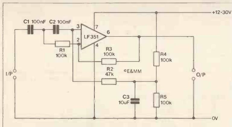
Figure 1. Suggested rumble filter circuit (one channel shown).
