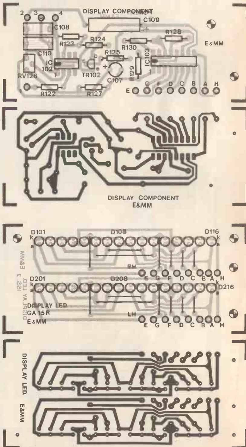
Figure 7. PPM PCBs and component overlays.
