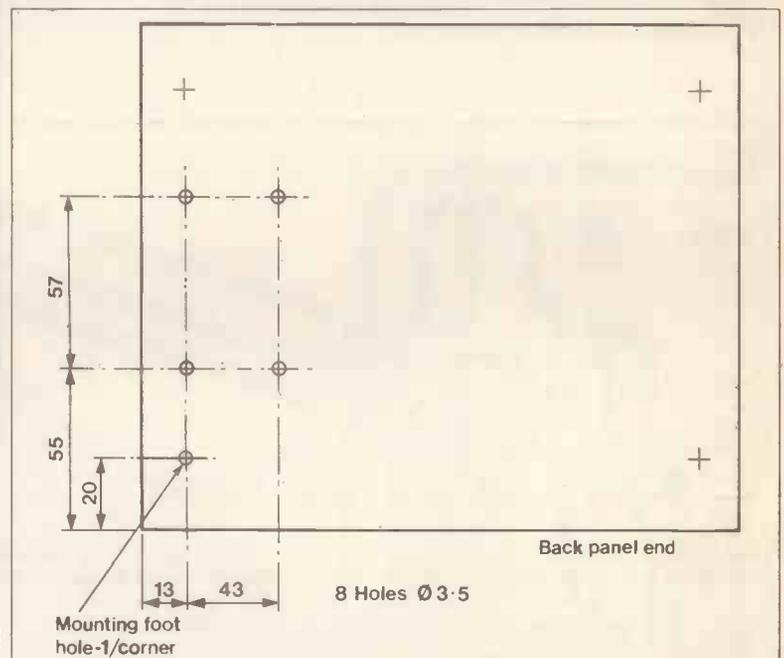
Figure 3(c). Drilling of base plate.
