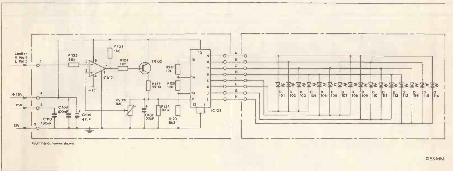
Figure 6. PPM circuit.
