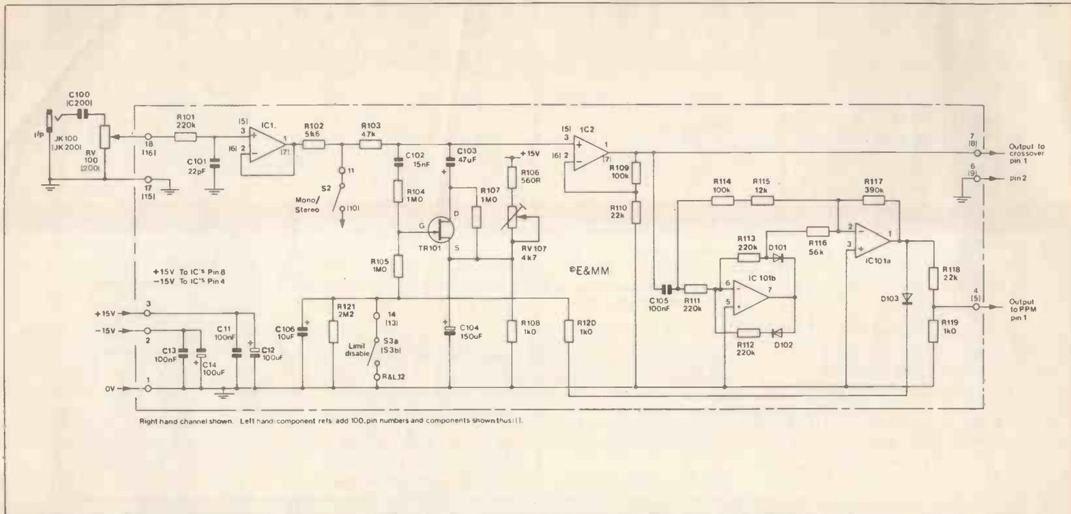
Figure 4. Limiter circuit.
