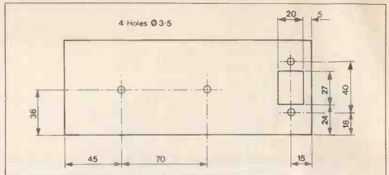
Figure 3(a). Drilling and cutting of back panel.
