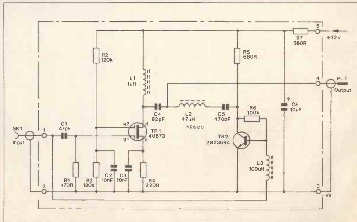
Figure 2. Car aerial booster: circuit diagram.
