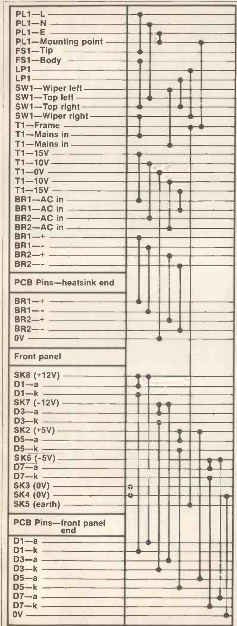
Figure 5. Pianola wiring diagram.
