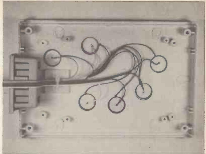
Wiring of the piezo transducers.
