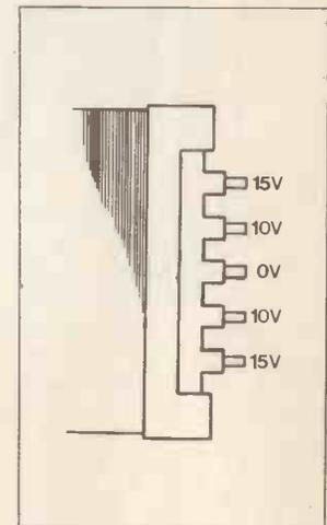
Figure 4. Transformer terminations.
