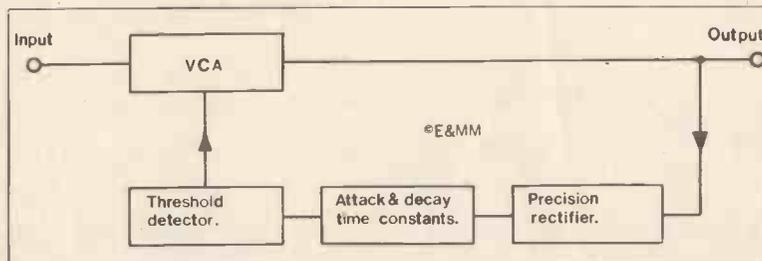
Figure 3. Limiter block diagram.
