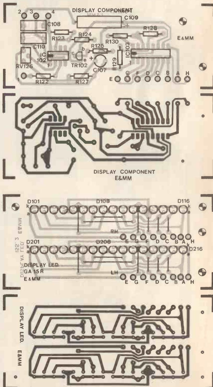
Figure 7. PPM PCBs and component overlays.
