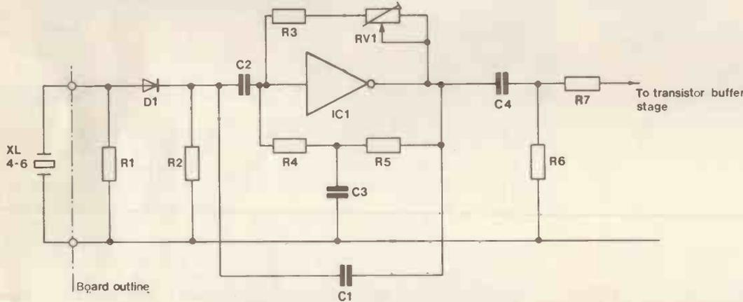
Figure 2(c). Circuit for lower-range drums.
