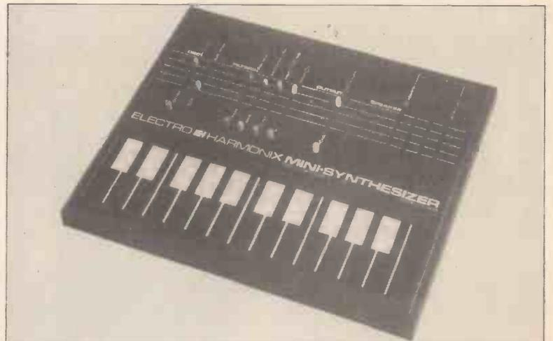
**ELECTRO-HARMONIX MINI-SYNTHESIZER (MODEL EH0400).** The Mini-Synthesizer is attractively presented in a light weight, slim, black case and is powered by two 9v batteries. Its main features are the easy-to-use controls and flat keyboard. The keyboard is touch-sensitive with the generated control voltage available for pitch and tone modulation. In addition, by sliding your finger along the upper portion of the white notes you have continuous pitch change instead of an individual note glissando.
