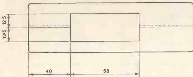
Figure 4. Battery box aperture. The cut-outs must be made in the top moulding end with the groove joint and bottom moulding end with the tongue.
