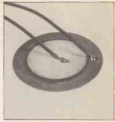
Soldering to the piezo transducers.
