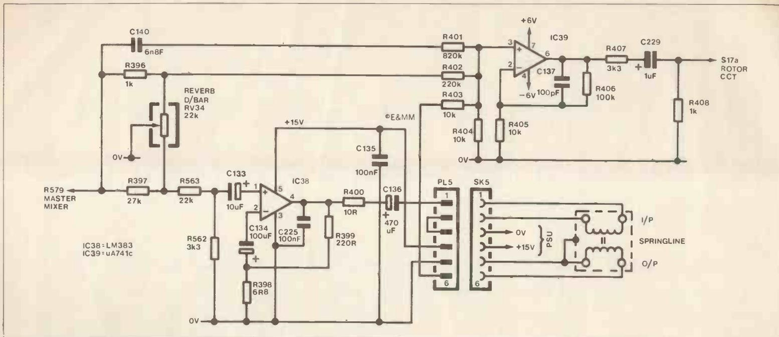
Figure 44. Circuit diagram of the reverb unit.
