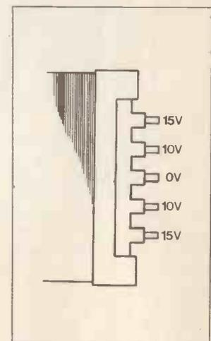
Figure 4. Transformer terminations.
