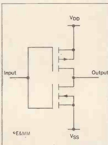
Figure 1. Output stage of 4069 inverter.
