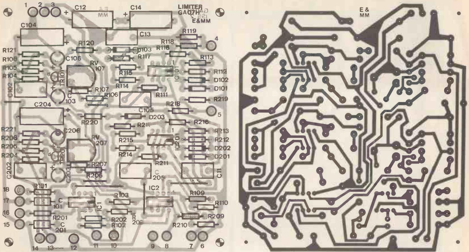
Figure 5. Limiter component overlay and PCB.
