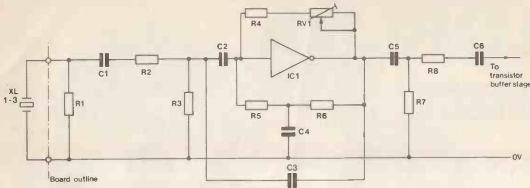
Figure 2(a). Circuit of upper range drums.
