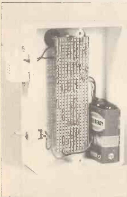
Rear view of unit showing Veroboard, buzzer, etc. in position.
