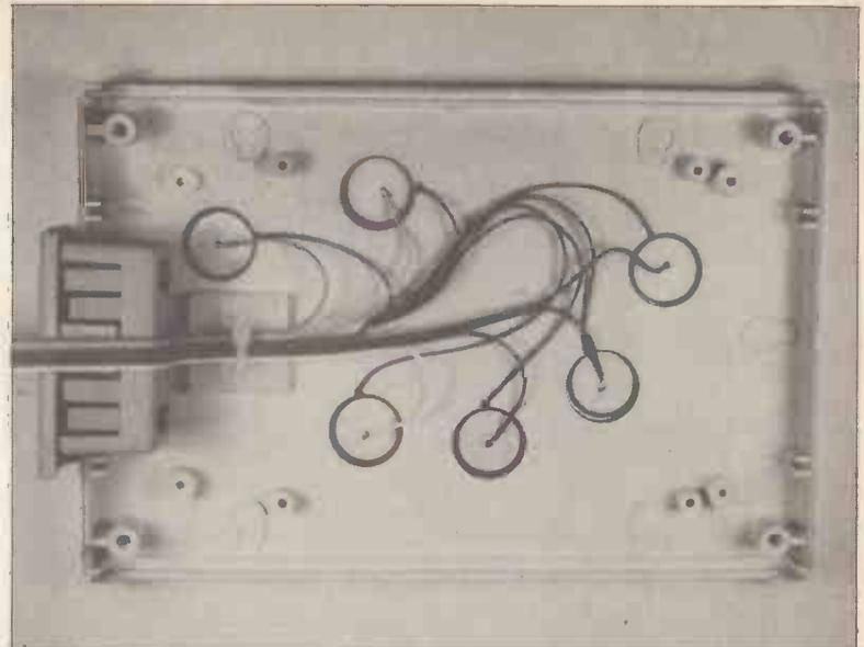
Wiring of the piezo transducers.
