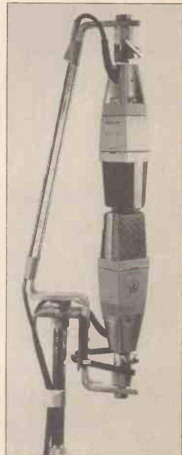
Figure 3. Crossed 'coincident' pairs. Shown above is AKG C414 Capacitor (switched to Cardioid or Hypercardioid or even 'figure of eight'), and below: Calrec CM652 Cardioid Capacitor pair.
