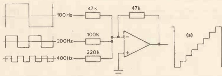
Figure 4. Op-Amp circuits giving (a) 'staircase' and (b) square wave.
