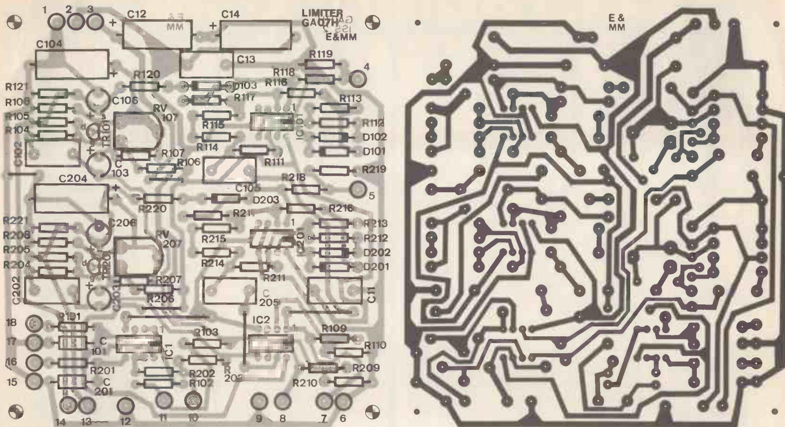
Figure 5. Limiter component overlay and PCB.
