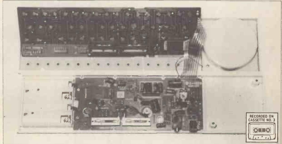
Inside the VL-Tone - the VLSI chip can be seen to the left of the ribbon cable.
