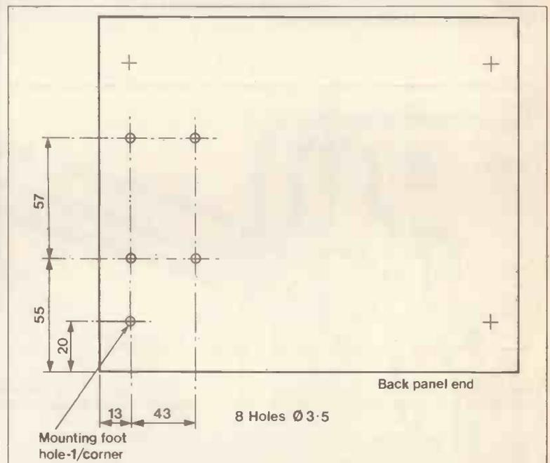
Figure 3(c). Drilling of base plate.
