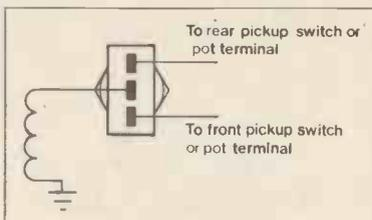
Figure 1. Centre pick-up wiring details.
