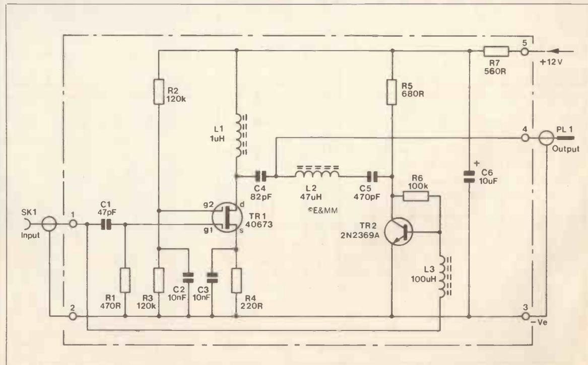
Figure 2. Car aerial booster: circuit diagram.
