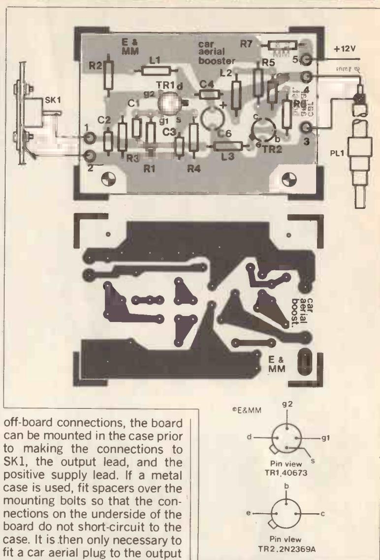
Figure 3. PCB track and component layout and SK1 fixing details.
