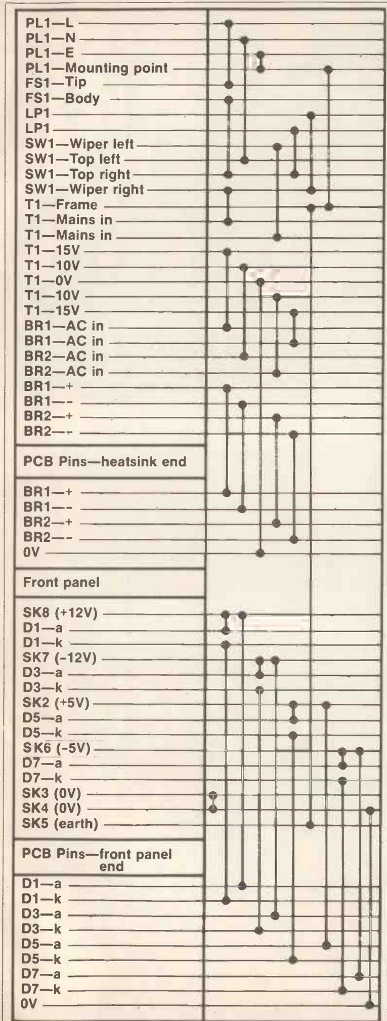
Figure 5. Pianola wiring diagram.
