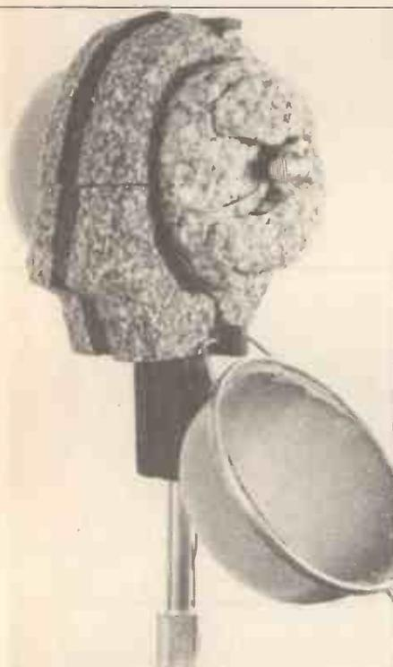
Figure 5. A really effective low cost dummy head using Omni tie clip (RS components 249-463) element mics in chipboard/foam/windshield construction.
