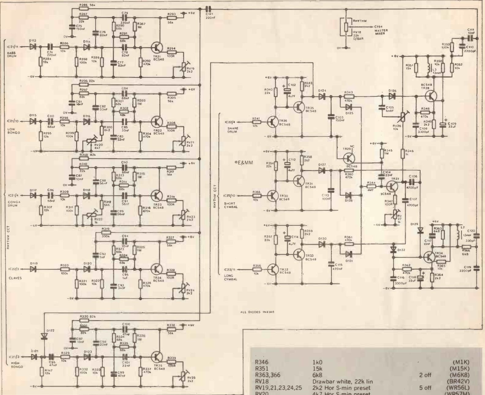
Figure 42. Circuit diagram of the rhythm voicing.
