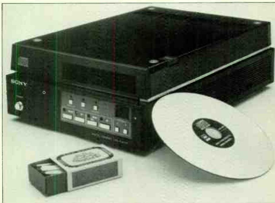
revolutionary design using an AlGaAs laser that was able to track pits etched on to a disc a fraction of the size of a normal disc. The success of this idea lay with some extremely sophisticated servo mechanisms, and, at that time, it wasn't possible to pack all the necessary electronics into a convenient LSI package.
