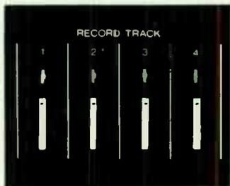
There are no restrictions, all four tracks can be recorded at once. Any input can be switched to any track. Or plug into the recorder direct, from another mixer, to add more channels or to capture a live performance.
