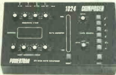
Programmed from a synthesiser, our latest design to be featured in *Electronics Today International*, the 1024 COMPOSER controls the synth with a sequence of up to 1024 notes or a large number of shorter sequences e.g. 64 of 16 notes all with programmable note length. In addition a rest or series of rests can be entered. It is mains powered but an automatically re-chargeable Nickel Cadmium battery, supplying the memory preserves the program after switch off.
