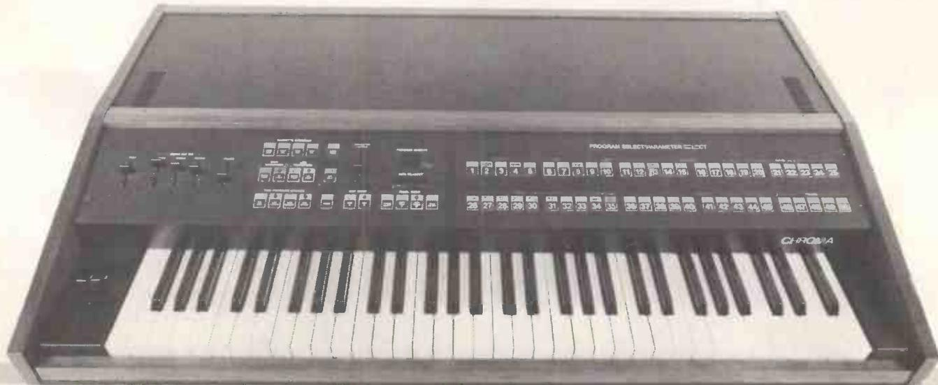
Readout display (prefixed by 'L'). Four switch buttons with indicator LEDs set link modes: LINK LOWER, LINK UPPER, LINK UNISON and NOLINK. The first two place the MAIN and LINK sounds above and below the specified 'Keyboard Split' point, whilst unison puts them together over the whole keyboard.
