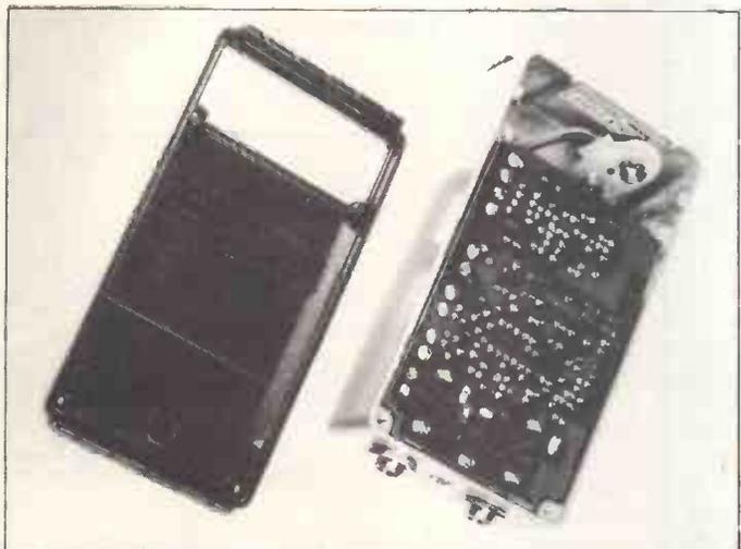
Step 17. PCB installed in case and insulation added to base plate.
