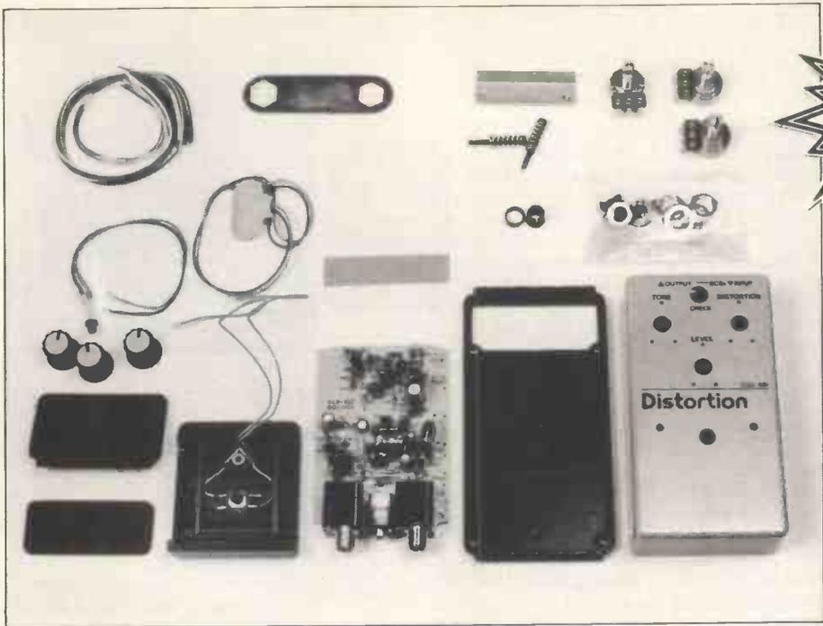
The complete set of parts laid out for checking prior to construction.
