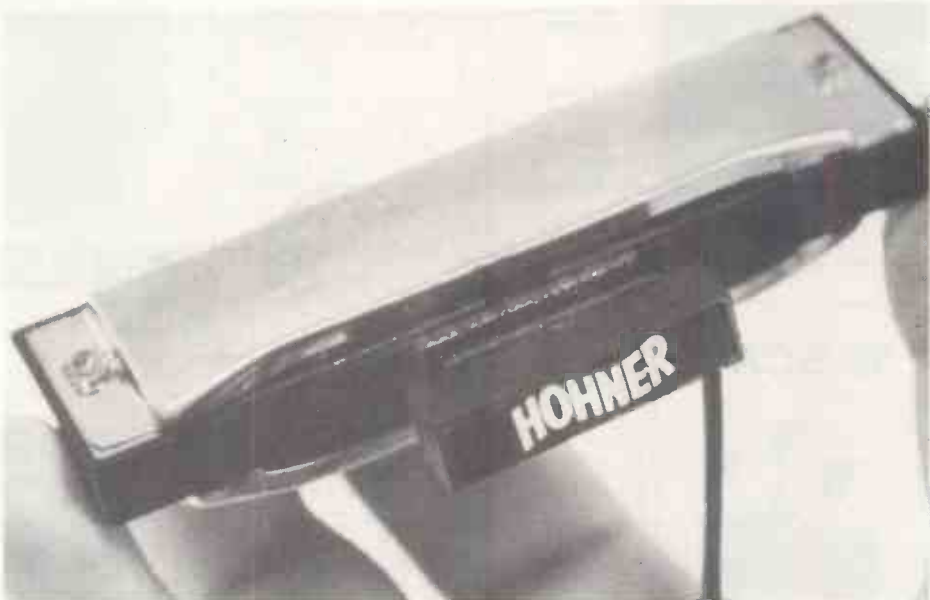
The bug in place on a diatonic harp, the Special 20.
