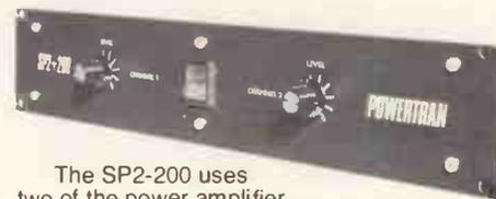
The SP2-200 uses two of the power amplifier sections of the MPA 200 (above), each with its own power supply. A custom designed toroidal transformer enables both channels to simultaneously deliver over 100W rms into 8 ohms. Each channel has its own volume control, and a sensitivity of 0.775mV (0dBm) makes this amplifier suitable for virtually all pre-amps or mixers.
