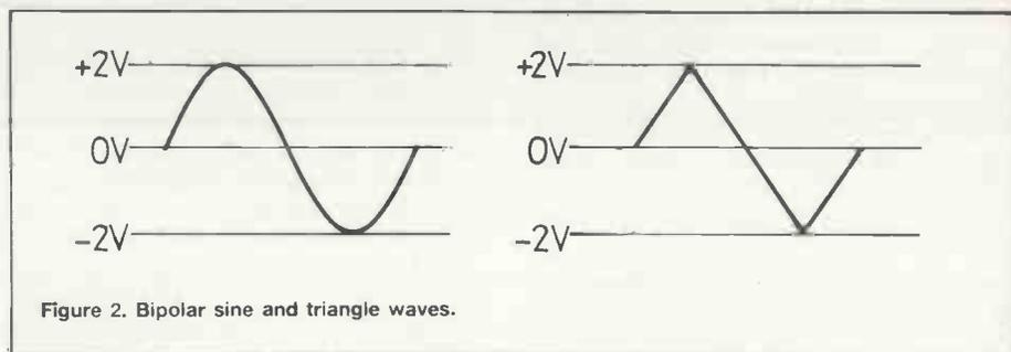
Figure 2. Bipolar sine and triangle waves.
