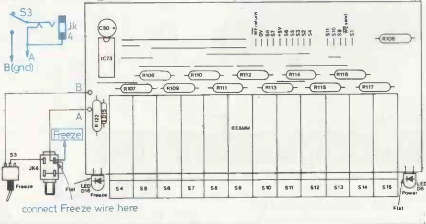
Figure 9. Mounting details (not to scale, dimensions in mm).
