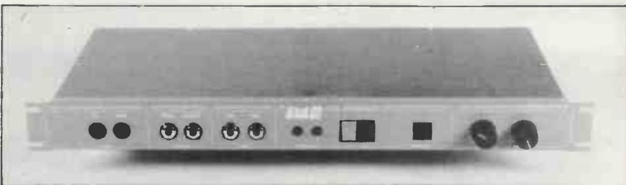
Yes, another 1U-high, 19" rack-mounting MIDI accessory, but this time with a purpose of some novelty: to bridge the frustrating gap between the composing power of MIDI sequencers and those treasured synth sounds that previously remained out of its reach, locked inside a box with only CV and Gate access.
