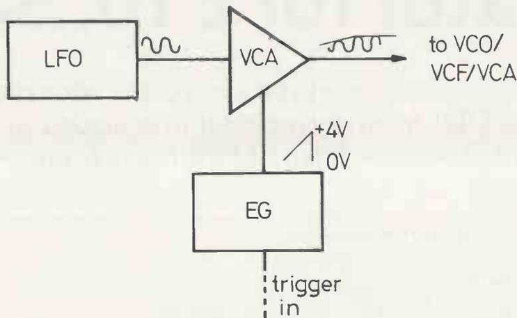
Figure 5(a). 'Traditional' delayed vibrato patch.
