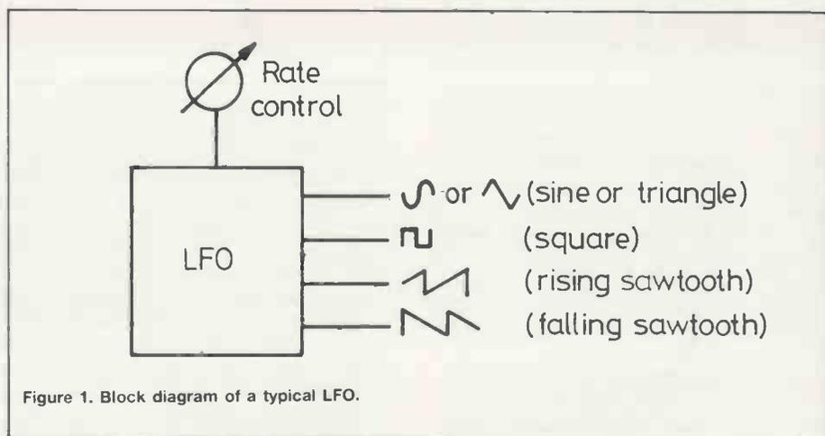
Figure 1. Block diagram of a typical LFO.
