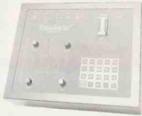
A microprocessor-controlled digital sound sampler, Eprom programmer, Eprom blower, Eprom copier, MIDI and computer serial in-output.
