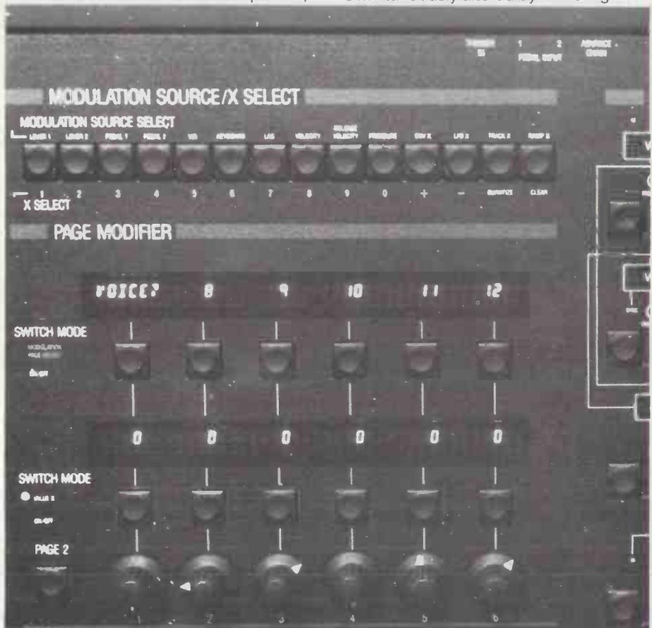
and tells you at a glance exactly what you can and can't modulate. These components are conceived as Pages, and are given stunning names like 'VCO1', 'FM/LAG' and 'LFO X'. Each Page has a Page Select button adjacent to it, which is used to call the associated parameters into the LED windows.
