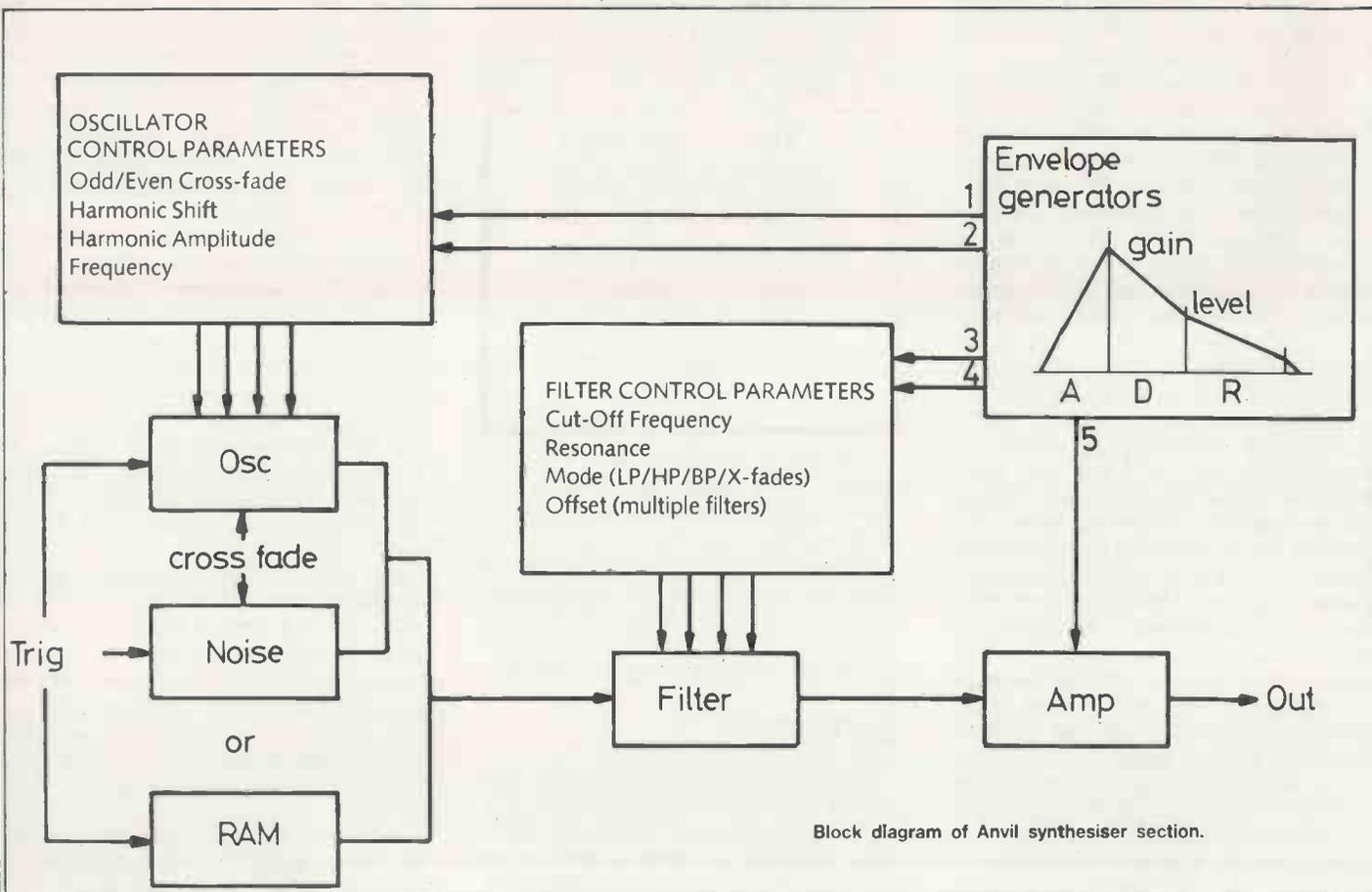
Block diagram of Anvil synthesiser section.
