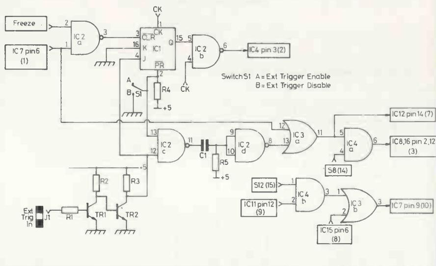
Figure 2. Circuit diagram of clock select section.
