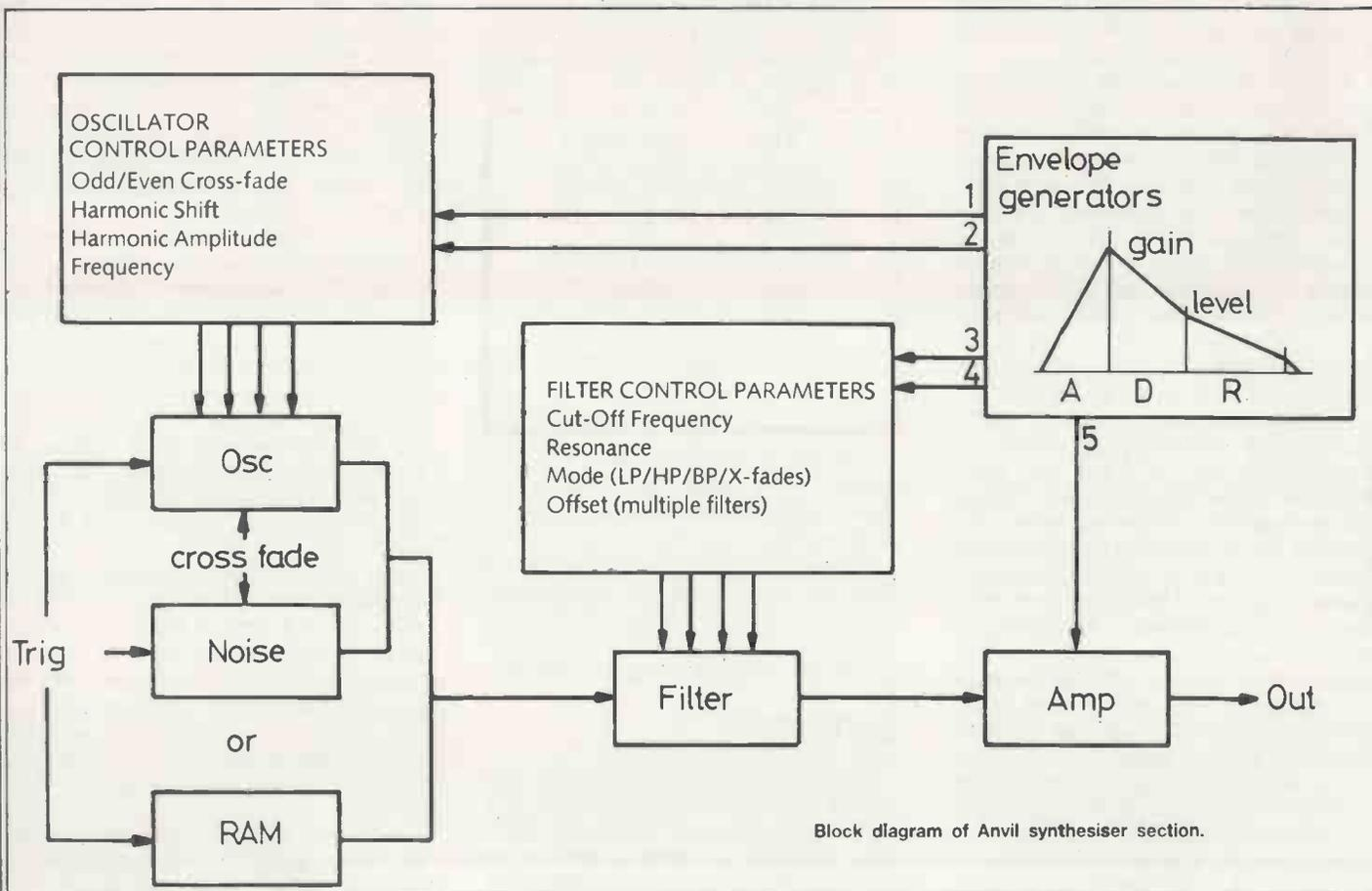
Block diagram of Anvil synthesiser section.
