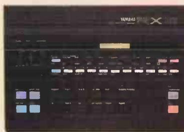
**RX15:** PCM Digital Drum Machine ■ MIDI compatible ■ 15 voices ■ real/step-time programming ■ Stereo Out with Pan ■ Cassette data storage.
