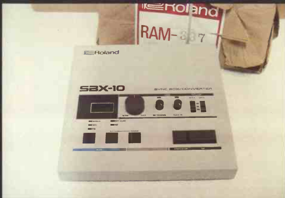
Roland SBX10 is new downmarket Sync Box; loses SMPTE, gains more realistic price-tag
