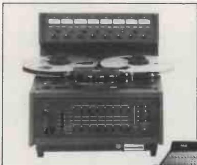
**16-TRACK:** The new Otari MX70 1" 16-track will change a lot of peoples' minds about 2" - versus-1"; with the TAC Matchless console, it makes a highly effective and versatile system. The MX70, in common with all Otari's multitracks, comes with a full synchroniser interface, making locking sound-to-video quick and simple.
