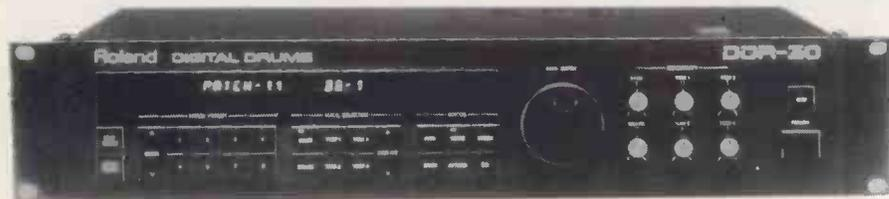
to eight variations of the basic sounds for each of the six drums in the kit. Then, you assemble these sounds in any combination to create a 'kit'; the system can store up to 32 of these. Extra storage of all parameters and sounds is available via external memory cartridges, which you insert into a slot on the DDR30's front panel.
