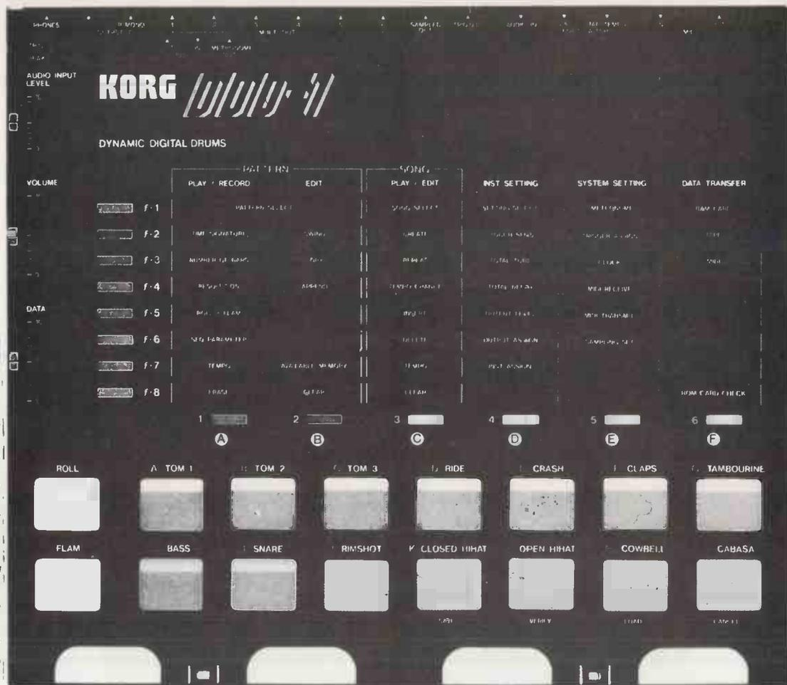
► “A clear matrix chart on the front panel lists all the machine’s parameters; it’s divided logically into six modes, and each mode is sub-divided into eight functions.”
