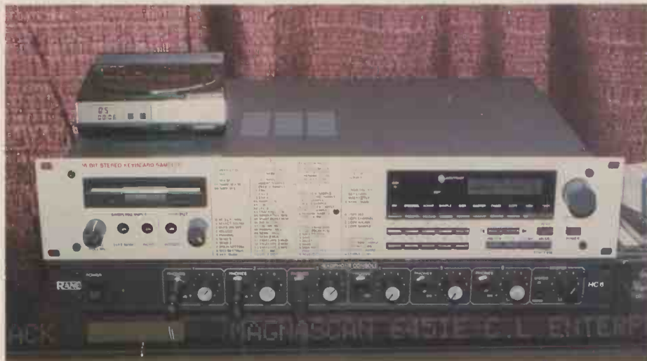
Dynacord's impressive new ADS, Advanced Digital Sampler, features 16-bit stereo sampling and extensive voice modulation capabilities.
