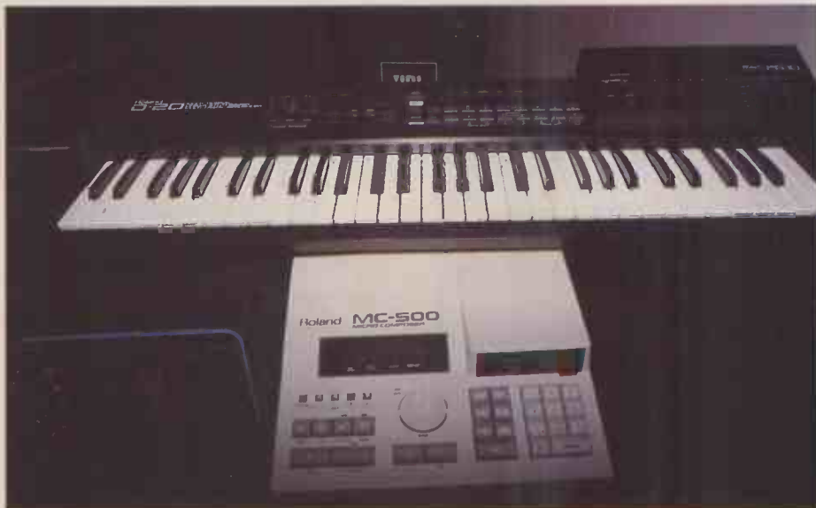
One of several new offerings from Roland is the D20, featuring an onboard 16,000 note, nine-track pattern sequencer and a 3½" disk drive.
