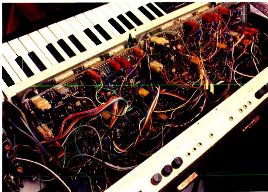
The innards of the analog hybrid V r oom ASS (Analog Stereo Sampler).
