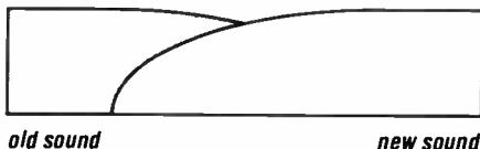
Figure 4. Wrongly applying panning curves to a crossfade.
