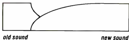
Figure 6. Proper exponential attack/decay crossfade.
