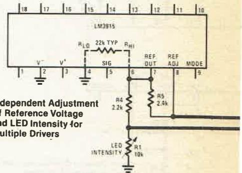
Independent Adjustment of Reference Voltage and LED Intensity for Multiple Drivers
