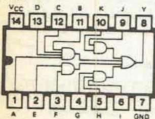
**7470 AND-GATED J-K POSITIVE EDGE-TRIGGERED FLIP-FLOP WITH PRESET AND CLEAR**
