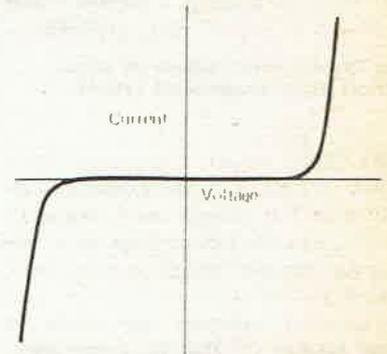
Fig.14. Varistor voltage-current characteristics.
