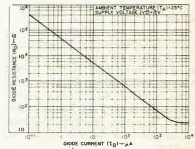
Diode resistance as a function of diode current.
