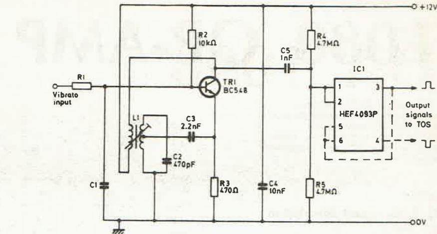
Fig. 2. Hartley oscillator and Wave-Shaping circuit.
