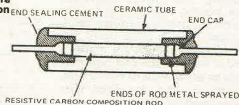
Fig.3(b). Assembly of a ceramic tube type insulated carbon composition resistance.
