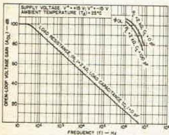
Open-loop voltage gain and phase lag vs frequency.
