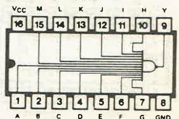
**74134** 12-INPUT NAND WITH TRI-STATE OUTPUT, OUTPUT IS DISABLED WHEN OUTPUT CONTROL IS HIGH
