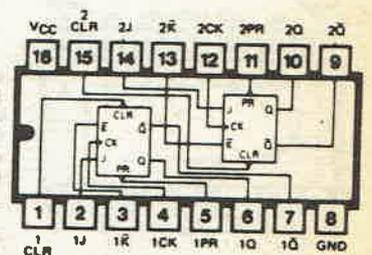
**74110 AND-GATED J-K MASTER-SLAVE FLIP-FLOP WITH DATA LOCK-OUT**
