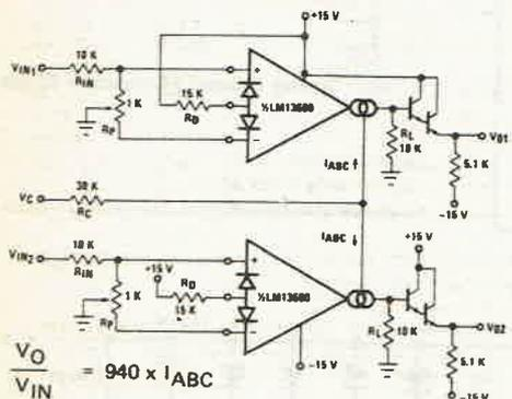
$$\frac{V_0}{V_{IN}} = 940 \times I_{ABC}$$
