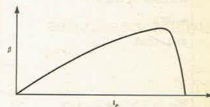
Typical gain ( $\beta$ ) variation of a transistor with increasing collector current.
