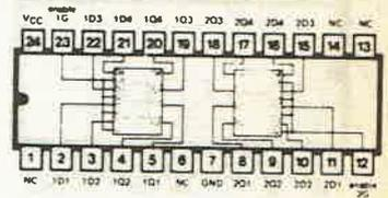
**74H101 AND-OR-GATED J-K NEGATIVE EDGE TRIGGERED FLIP-FLOP WITH PRESET**
