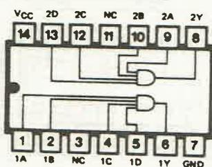
**7422 DUAL FOUR-INPUT NAND, OPEN COLLECTOR OUTPUTS**
