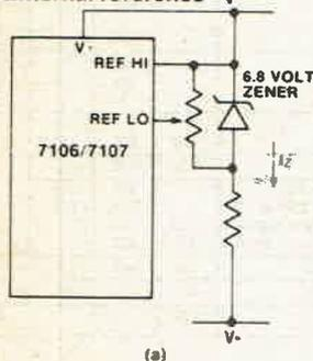
For many applications, the internal reference of 2.8 V between V+ and COMMON is adequate, but power dissipation in the 7107 LED version can wreck this. However, an external reference can be added as shown in Fig. 6.
