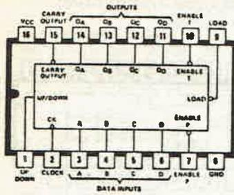
**74169 BINARY FOUR-BIT UP-DOWN COUNTER, SYNCHRONOUS**
