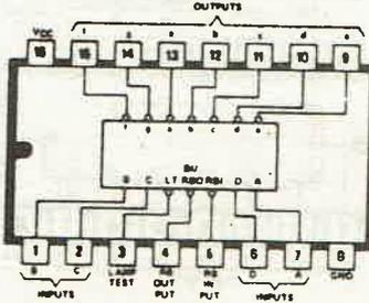
**74249** BCD TO SEVEN SEGMENT DECODER/DRIVER, OPEN-COLLECTOR OUTPUTS
