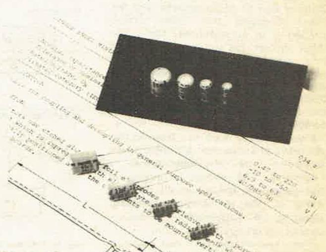
Fig. 11. PCB-mounting electrolytics allow greater component density.
