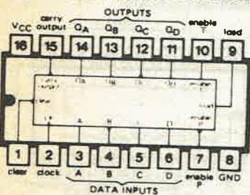
**74163 SYNCHRONOUS BINARY COUNTER, FOUR BIT WITH SYNCHRONOUS CLEAR**
