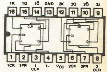
**7478 DUAL J-K FLIP-FLOP WITH PRESET, COMMON CLEAR AND COMMON CLOCK**
