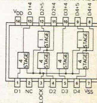
**4009/4049 HEX INVERTER/BUFFER TO TTL CONVERTER**
