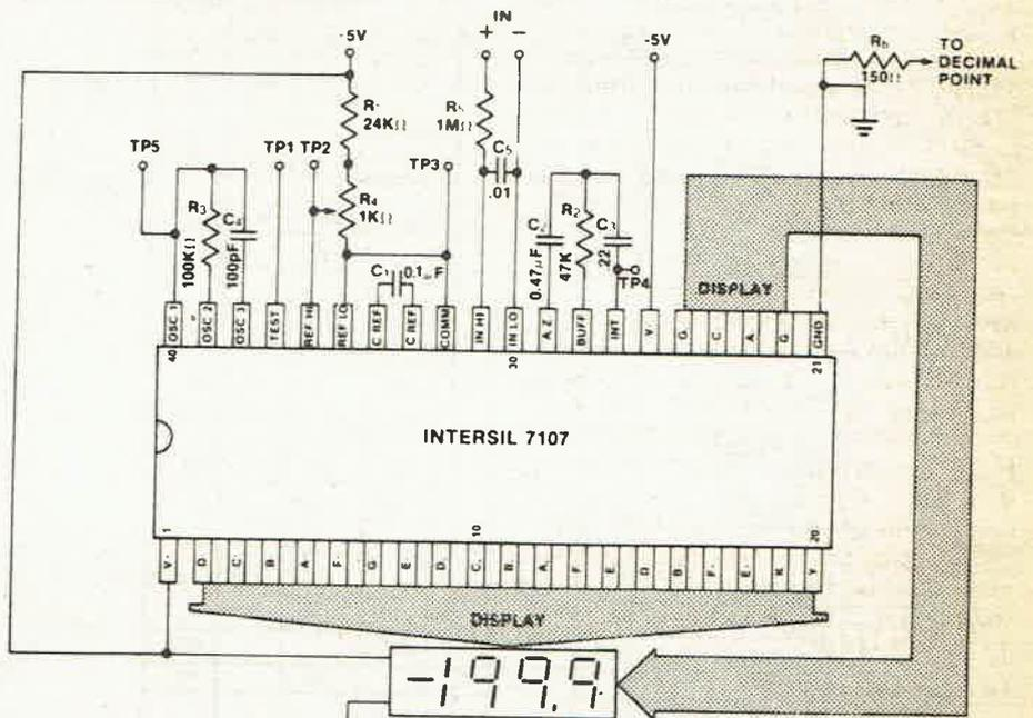
Fig. 1 LED Digital Panel Meter using ICL 7107
