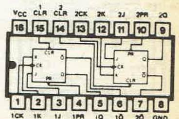
**74113 DUAL J-K NEGATIVE EDGE TRIGGERED FLIP-FLOP WITH PRESET**
