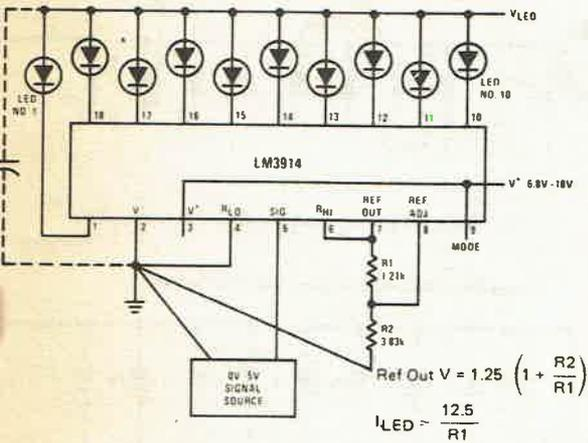
**Note 1:** Grounding method is typical of all uses. The 2.2 μF capacitor is needed if leads to the LED supply are 6" or longer.
