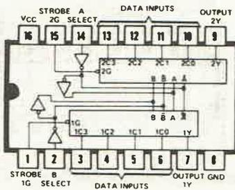
74353 DUAL FOUR LINE TO SINGLE LINE DATA SELECTORS/MULTIPLEXERS, TRI-STATE OUTPUTS
