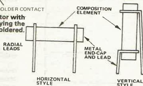
Fig.2(c). Carbon composition resistor with pressed metal end-cap and lead connections for plugging into p.c. boards — the 'plug-gable' style. The end-caps are forced over the ends of the composition rod element.
