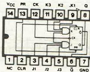
**74H103 DUAL J-K NEGATIVE EDGE TRIGGERED FLIP-FLOP WITH PRESET AND CLEAR**
