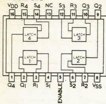
**4044 QUAD NAND R/S LATCHES WITH TRI-STATE OUTPUTS**
