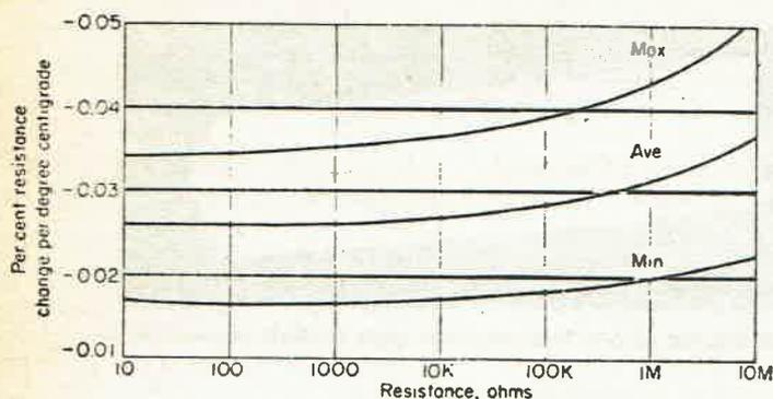
Fig. 6. Typical temperature-coefficient spread for deposited-carbon resistors.
