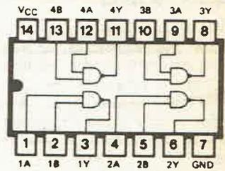
**7401 QUAD TWO-INPUT NAND, OPEN COLLECTOR OUTPUTS**
