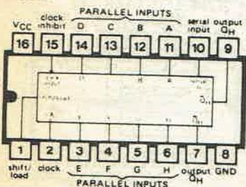
**74166 EIGHT-BIT SHIFT REGISTER, SERIAL/PARALLEL INPUT, SERIAL OUTPUT**
