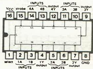
**74159 FOUR-TO-16-LINE DECODER/DEMULTIPLEXER, OPEN COLLECTOR OUTPUTS**
