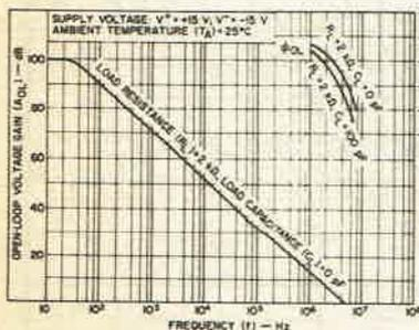
Open-loop voltage gain and phase lag as a function of frequency.
