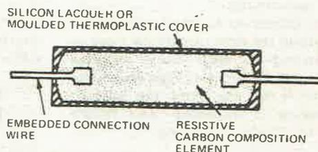
Fig.3(a). Insulated carbon composition resistor construction.
