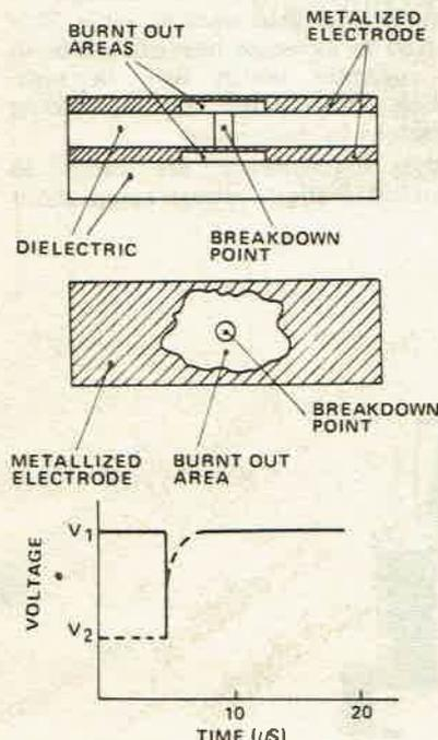
Fig. 8. Process of self healing of a metallized dielectric capacitor. The voltage trace is typical during the process.
