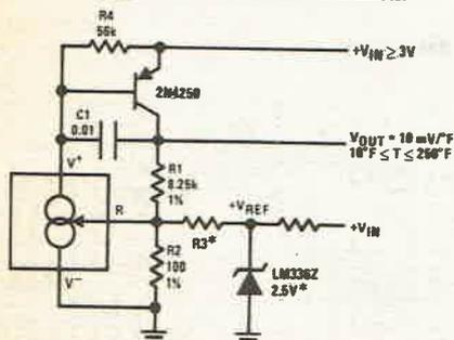
\*Select  $R3 = V_{REF} / 583 \mu A$ .  $V_{REF}$  may be any stable positive voltage  $\geq 2V$ . Trim R3 to calibrate.
