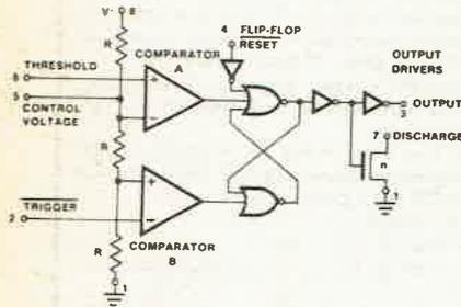
This block diagram reduces the circuitry down to its simplest equivalent components
