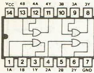
7433 QUAD TWO-INPUT NOR, OPEN COLLECTOR OUTPUTS
