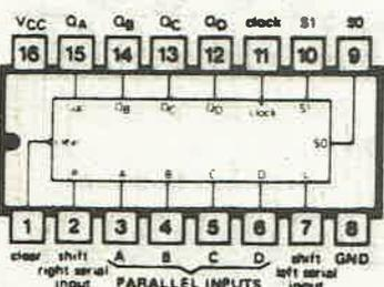
**74195 FOUR-BIT PARALLEL ACCESS SHIFT REGISTER**
