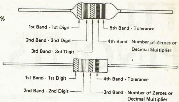
Fig.16. The standard resistor colour code marking.
