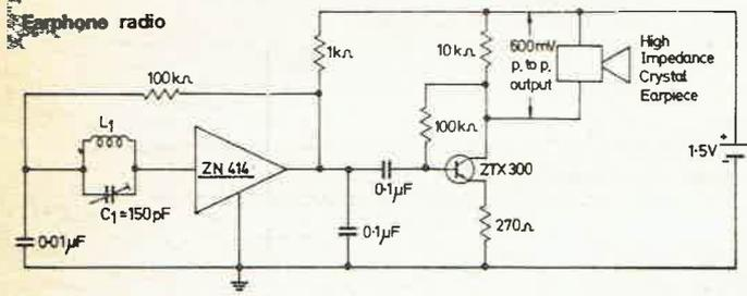
$L_1 \sim 80$  turns of 0.3 mm. dia. enamelled copper wire on a 5 cm. or 7.5 cm. long ferrite rod. Do not expect to adhere rigidly to the coil-capacitor details given. Any value of  $L_1$  and  $C_1$  which will give a high 'Q' at the desired frequencies may be used.
