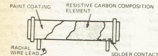
Fig.2(a). Carbon composition resistor with the end connections made by spraying the ends with metal and the leads soldered.
