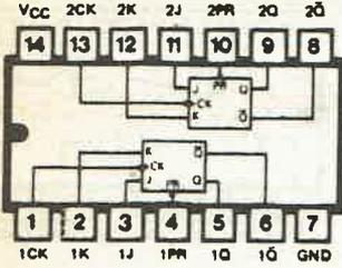
**74114 DUAL J-K NEGATIVE EDGE TRIGGERED FLIP-FLOP WITH PRESET COMMON CLEAR AND COMMON CLOCK**
