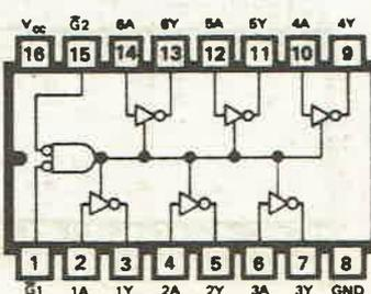
74367 HEX BUS DRIVER, TRI-STATE OUTPUTS, FOUR-LINE AND TWO-LINE ENABLE INPUTS
