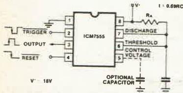
Figure 4: Monostable Operation
