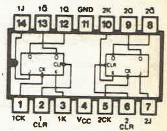
**7474 DUAL D-TYPE POSITIVE EDGE TRIGGERED FLIP-FLOP WITH PRESET AND CLEAR**
