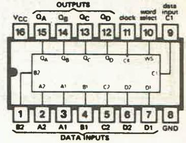
74299 EIGHT-BIT BI-DIRECTIONAL UNIVERSAL SHIFT/STORAGE REGISTER, TRI-STATE OUTPUTS, DIRECT CLEAR
