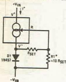
\*Select ratio of R1 to  $R_{SET}$  to obtain zero drift.  $I^+ \approx 2 I_{SET}$
