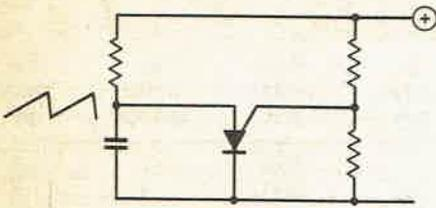
of current the gain drops quickly and the device turns off. These devices are typically used as switches and oscillators.
