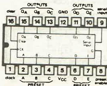
7497 SYNCHRONOUS SIX-BIT BINARY RATE MULTIPLIER
