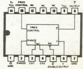
74326 DUAL VCO WITH TWO-PHASE OUTPUT AND ENABLE CONTROL
