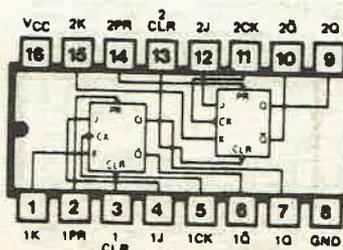
**74112 DUAL J-K NEGATIVE EDGE TRIGGERED FLIP-FLOP WITH PRESET AND CLEAR**
