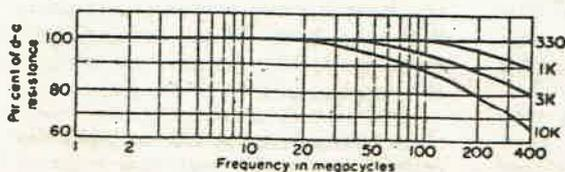
Fig. 8. Approximate frequency characteristics for ½-watt deposited-carbon resistor.
