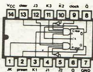
**74H106 DUAL J-K EDGE TRIGGERED FLIP-FLOP WITH PRESET AND CLEAR**
