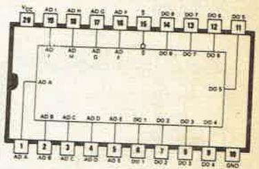
74670 FOUR-BY-FOUR REGISTER FILE, TRI-STATE OUTPUTS, SIMULTANEOUS READ/WRITE, EXPANDABLE TO 1024 WORDS
