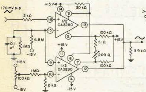
Triangle wave-to-sine wave converter.
