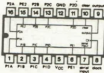
7495 FOUR-BIT SHIFT REGISTER, PIPO AND BIDIRECTIONAL
