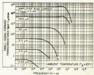
Amplifier gain as a function of frequency.
