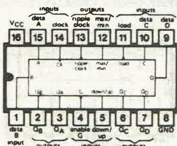
**74192 BINARY SYNCHRONOUS UP/DOWN COUNTER, WITH DUAL CLOCK AND CLEAR**
