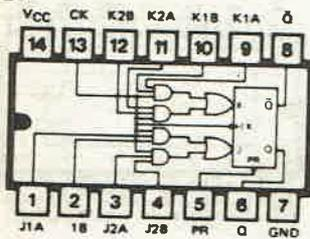
**74H102 AND-GATED NEGATIVE EDGE TRIGGERED FLIP-FLOP WITH PRESET AND CLEAR**
