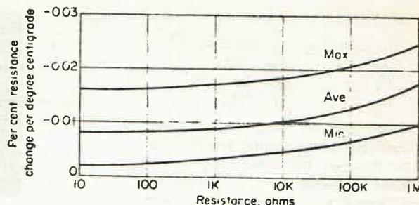
Fig. 7. Typical temperature-coefficient spread for boron-carbon resistors.
