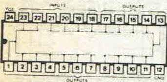
**74160 SYNCHRONOUS DECADE COUNTER, FOUR BIT WITH DIRECT CLEAR**
