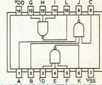
**4026 DECADE COUNTER DIVIDER, SEVEN-SEGMENT DECODED OUTPUTS**
