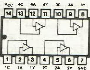
**74126 QUAD BUS BUFFER WITH TRI-STATE OUTPUTS (DISABLED WHEN C IS LOW)**
