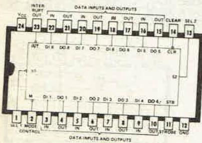
74474, 74475 512-BY-8-BIT PROM, GATED STORE; 474 HAS TRI-STATE OUTPUTS, 475 HAS OPEN-COLLECTOR OUTPUTS
