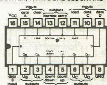
**74193 BINARY SYNCHRONOUS UP/DOWN COUNTER, WITH DUAL CLOCK AND CLEAR**
