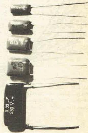
Fig. 6. Resin dipped polyester capacitors.
