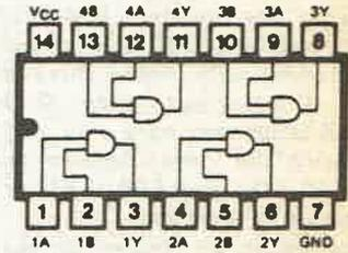
**7409 QUAD TWO-INPUT AND, OPEN COLLECTOR OUTPUTS**
