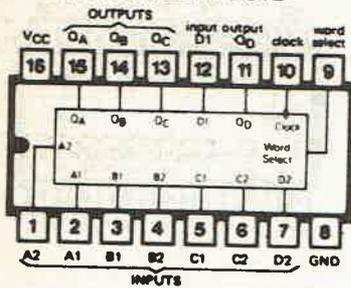
**74L99 FOUR-BIT BIDIRECTIONAL UNIVERSAL SHIFT REGISTER, SERIAL J-K INPUTS**
