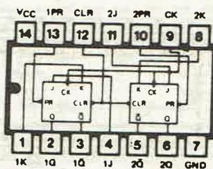
**74109 DUAL J-K POSITIVE EDGE TRIGGERED FLIP-FLOP WITH PRESET AND CLEAR**
