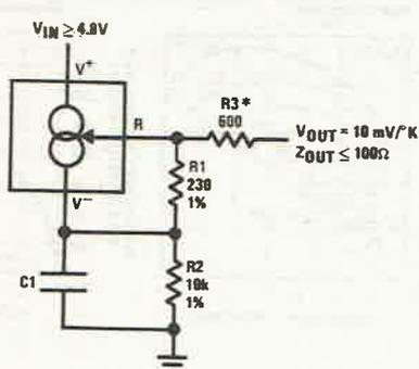
\*Output impedance of the LM134 at the "R" pin is approximately  $-R_O / 16\Omega$ , where  $R_O$  is the equivalent external resistance connected to the  $V^-$  pin. This negative resistance can be reduced by a factor of 5 or more by inserting an equivalent resistor in series with the output.
