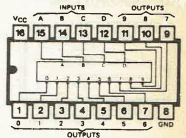
7446 BCD TO SEVEN-SEGMENT DECODER/DRIVER, 30 V OPEN COLLECTOR OUTPUTS, ACTIVE LOW
