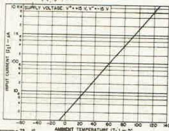
Input current vs ambient temperature.
