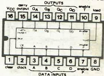
**74162 SYNCHRONOUS DECADE COUNTER, FOUR BIT WITH SYNCHRONOUS CLEAR**
