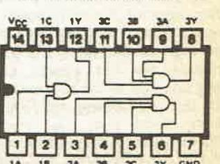
**7412 TRIPLE THREE-INPUT NAND, OPEN COLLECTOR OUTPUTS**
