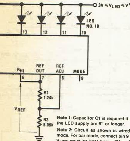
**Note 1:** Capacitor C1 is required if leads to the LED supply are 6" or longer.
