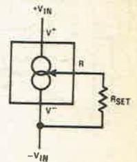
Terminating Remote Sensor for Voltage Output
