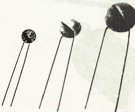
Fig.13. Typical PTC thermistors (actual size).
