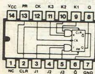
**74111 DUAL J-K MASTER-SLAVE FLIP-FLOP WITH DATA LOCK-OUT**
