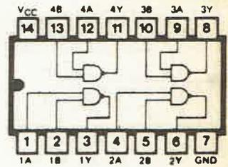
7438 QUAD TWO-INPUT NAND/BUFFER, OPEN COLLECTOR OUTPUTS
