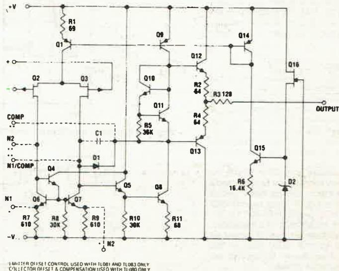
Fig 1. Schematic diagram for TL080 family.
