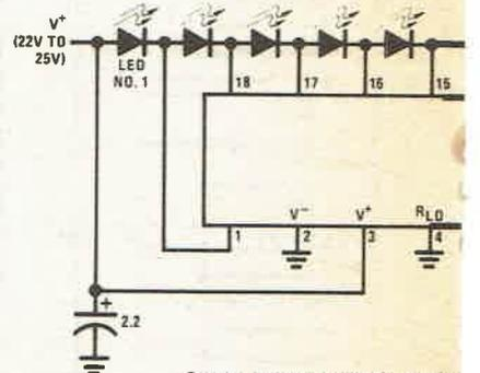
Supply current drain is only 15 mA with LEDs illuminated.
