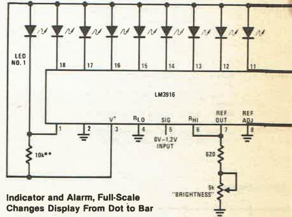
Indicator and Alarm, Full-Scale Changes Display From Dot to Bar
