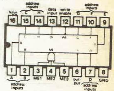
**74247** BCD TO SEVEN-SEGMENT DECODER/DRIVER, 15 V OPEN-COLLECTOR ACTIVE-LOW OUTPUTS
