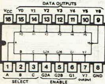
**74139** DUAL TWO-TO-FOUR-LINE DECODER/MULTIPLEXER
