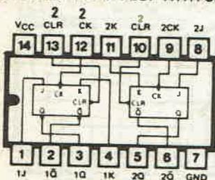
**74108 DUAL J-K NEGATIVE EDGE TRIGGERED FLIP-FLOP WITH PRESET, COMMON CLEAR, AND COMMON CLOCK**
