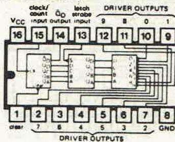
**74143** COUNTER/LATCH/DECODER/DRIVER (15 mA CONSTANT CURRENT 1 TO 5 V OUTPUT RANGE)
