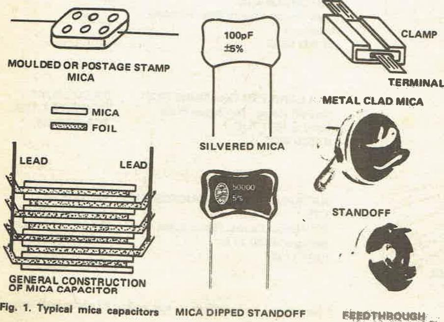
Fig. 1. Typical mica capacitors
