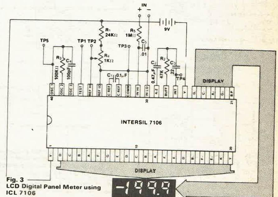
Fig. 3 LCD Digital Panel Meter using ICL 7106
