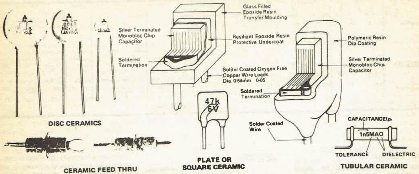
Fig. 2. Ceramic capacitors.
