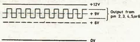
Fig. 5. Output signal from pin 2, 3, 4, 5 or 6.
