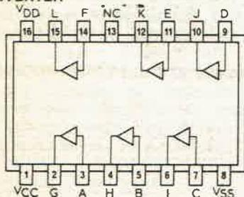
Note:  $V_{DD}$  is input supply and is not used on 4049/4050;  $V_{CC}$  supplies output circuitry, plus input on 4049/4050
