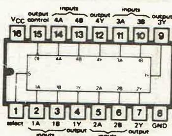
**74289** 64-BIT (16 BY 4) RAM, OPEN-COLLECTOR OUTPUTS
