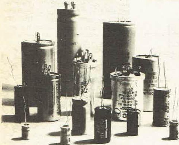
Fig. 10. A selection of electrolytic capacitors.
