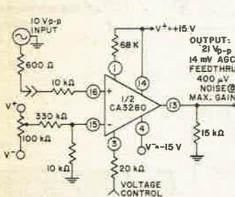
Typical gain control circuit.
