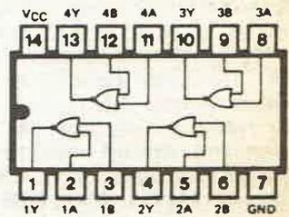
**7403 QUAD TWO-INPUT NAND WITH OPEN COLLECTOR OUTPUTS**
