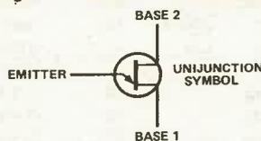
Unijunction transistors consist of a base region of N-type silicon with two connections, and a tiny area of P-type silicon, called the emitter with its own connection. The two connections to the base are used to set up a potential gradient across the base region.
