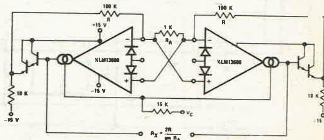
Floating Voltage Controlled Resistor
