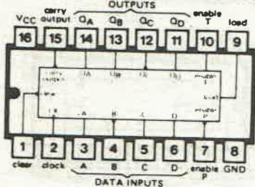
**74161 SYNCHRONOUS BINARY COUNTER, FOUR BIT WITH DIRECT CLEAR**
