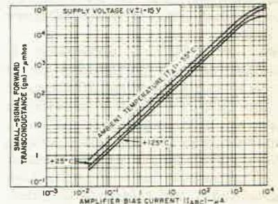
Amplifier gain as a function of amplifier bias current.
