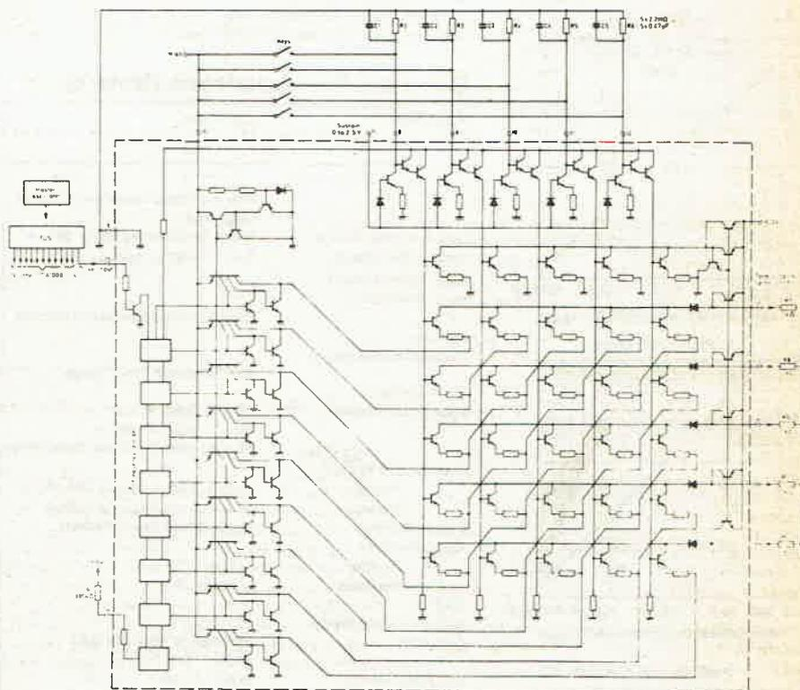
Fig. 1. TDA1008 and basic peripheral circuit.
