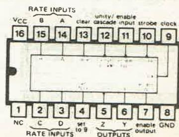
**74168 DECADE FOUR-BIT UP-DOWN COUNTER, SYNCHRONOUS**
