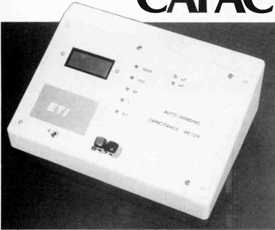
This project is designed to measure capacitance in the range of 100pF to 1000uF with no help (or hindrance) from the operator once the component is connected. Apart from the power switch, there are no external switches or knobs to adjust and only one internal adjustment. Once the instrument is working, setting up and using it is very simple.
