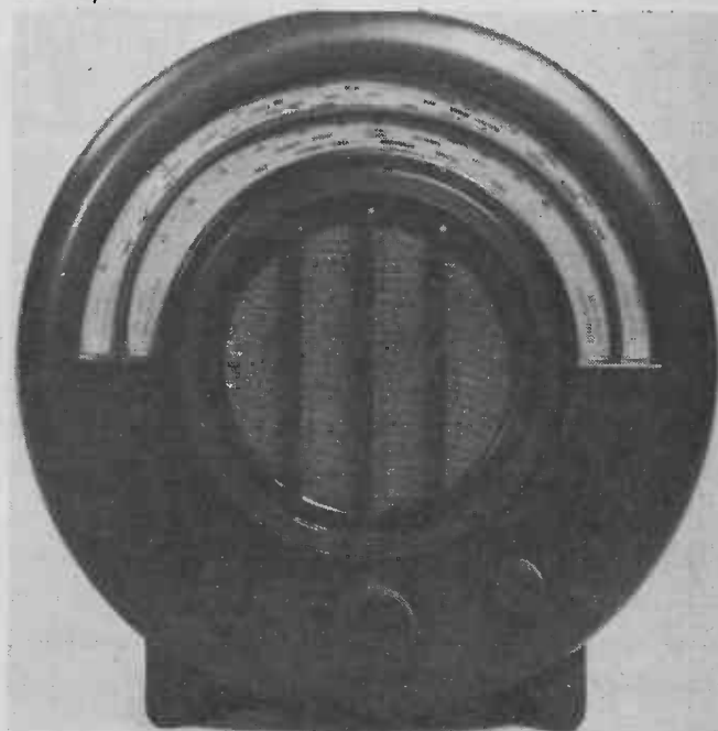
Superhet from 1932 and Ekco, 3-valve design, could be battery run.
