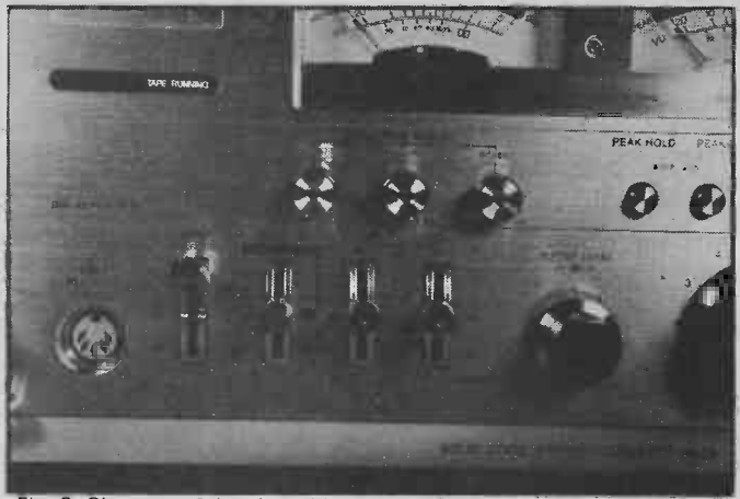
Fig. 3. Close-up of the clever bits. Above the general input controls can be seen the bias fine adjust control which allow tuning up for each tape formulation available. The control to be used is illuminated once the input is set to 'Test'.
