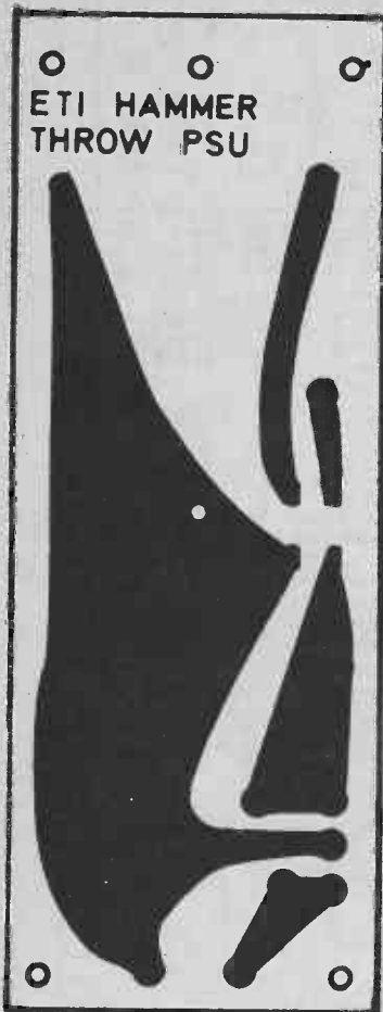
Fig. 3. Foil pattern of power supply board shown full size (120 x 45 mm).
