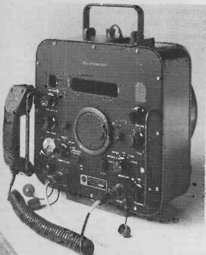
Figure 2. Tellurometer model MRAS, uses the microwave method to measure distance from 100 m to 50 km to an accuracy better than 1 in 500,000. Modern electronics have made it easy to operate. Readout is a 7-digit display of range.
