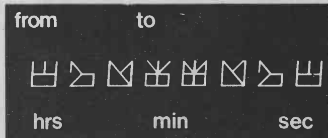
The symbols BORIS uses to identify the chess pieces. Shown here is the back rank of the white men. The black appear upside down so you can tell which men are which. Pawns appear as triangles.
