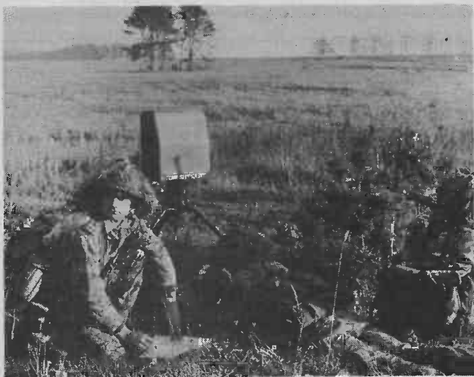
Above left: the ZB298 is a mobile ground surveillance radar for the detection and location of moving targets.
