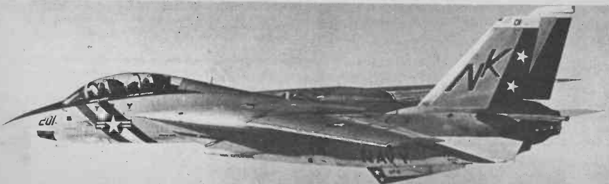
Below, the F-14 combat aircraft. It has a fire control system which can attack six targets simultaneously at 200km range, while tracking 18 others, deciding for itself which pose the greatest threats and facing them in that order! In addition the wings are automatically swept back to the optimum position by MPU control.
