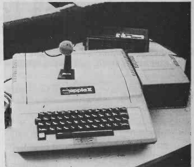
The familiar Apple II with a speech recognition board installed. It worked remarkably well and 'echoed' back your word through a synthesizer.
