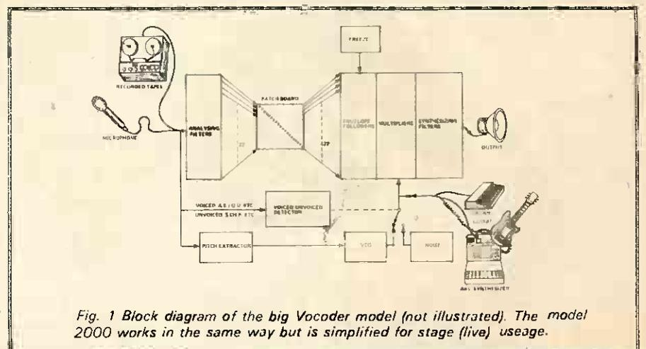
Fig. 1 Block diagram of the big Vocoder model (not illustrated). The model 2000 works in the same way but is simplified for stage (live) useage.
