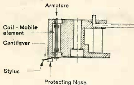
Cutaway drawing of an early Ortofon moving coil device. An interesting feature is the vertical armature mounting. Note the protective nose mounted to safeguard the stylus!
