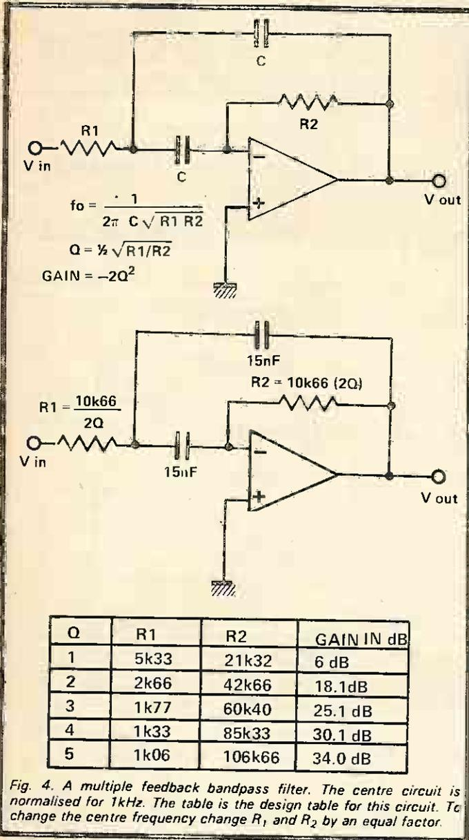
gives a design chart, normalised for 1kHz operation. First, choose a Q factor and then perform the frequency scaling. For instance, if the centre is 250Hz, then multiply both  $R_1$  and  $R_2$  by a factor of 4. If a high Q is required, then a multiple op amp circuit must be used. The 'state variable' and the 'Bi-Quad' are two such circuits and Q's as high as 500 may be obtained with them.
