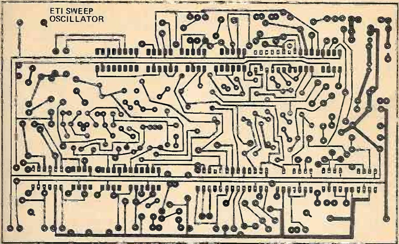
Fig. 5 Full size pattern for the PCB.
