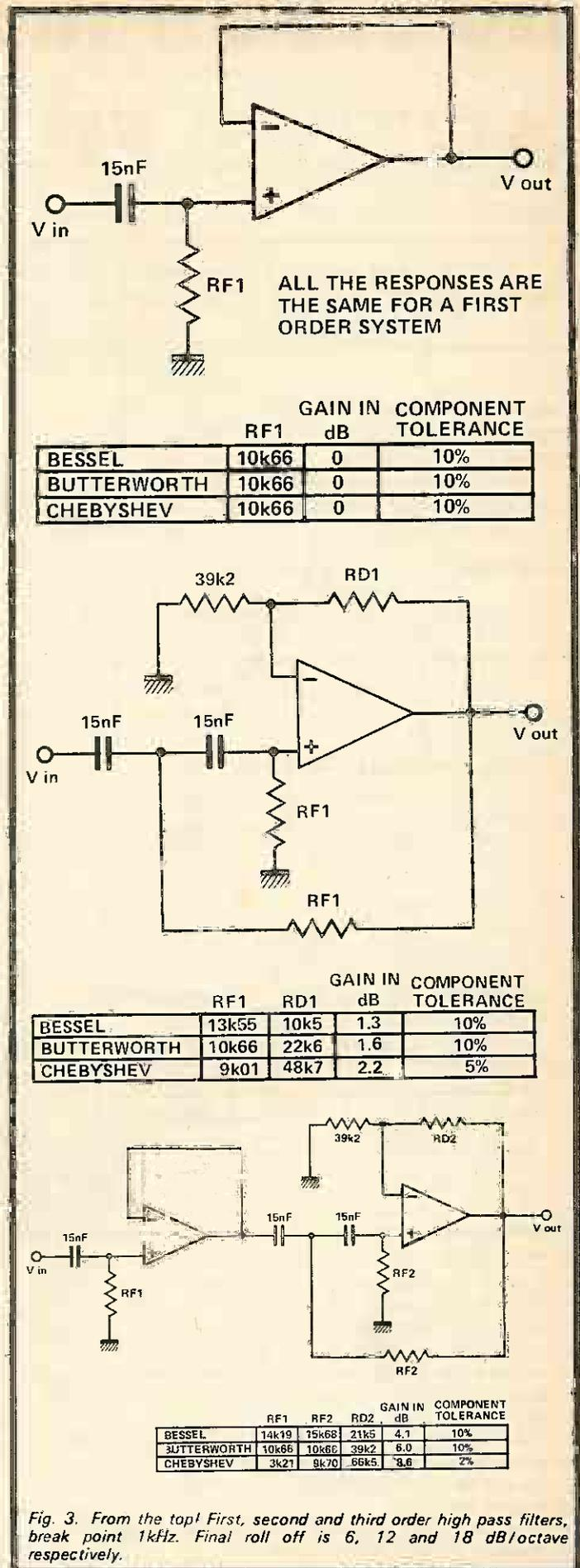
Fig. 3. From the top: First, second and third order high pass filters, break point 1kHz. Final roll off is 6, 12 and 18 dB/octave respectively.
