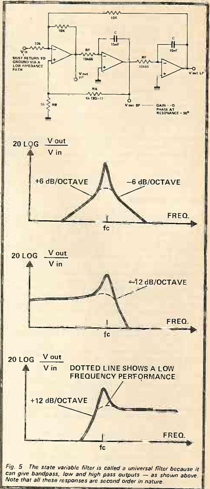
The Q is determined by the ratio of two resistors,  $R_A$  and  $R_B$ , where  $R_A/R_B = 3Q - 1$ . The resonant frequency  $f_c =$
