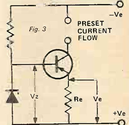
the collector current too) is thus defined as  $I_e = V_e R_e$  and by selection of  $R_e$  the value of  $I_e$  (or  $I_c$ ) is determined. As long as there is about one volt between emitter and collector the collector current remains constant at this chosen value - or at least until a resistor or load of too large a voltage and so robs the collector of its working voltage.
