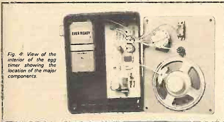
Fig. 4. View of the interior of the egg timer showing the location of the major components.
