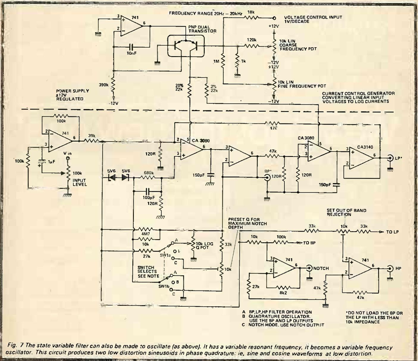
Fig. 7 The state variable filter can also be made to oscillate (as above). It has a variable resonant frequency, it becomes a variable frequency oscillator. This circuit produces two low distortion sineusoids in phase quadrature: ie, sine and cosine waveforms at low distortion.
