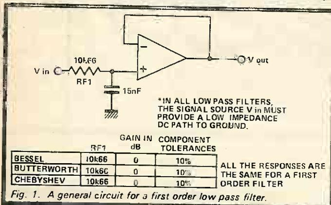
Key' filters have been used as the basic building blocks. If operation at a frequency other than 1kHz is required, then the resistor/s R<sub>f</sub> should be scaled accordingly, (the R<sub>d</sub> resistors are not altered). For example, if operation is required at 250Hz, then the R<sub>f</sub> in the chart must be multiplied by
