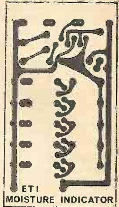
Above left: Component overlay for our Soil Moisture Indicator. The only thing to be careful of here is the orientation of the semiconductors.
