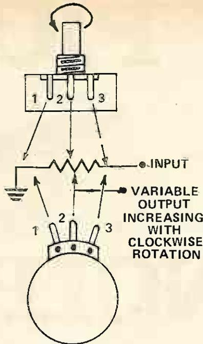
Fig. 6. Connecting a pot as a simple 'increase clockwise' control (e.g. volume).
