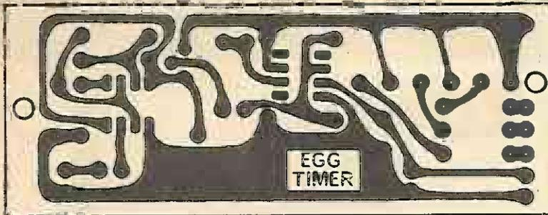
Fig. 2. Foil pattern of egg timer shown full size (100mm x 40mm).
