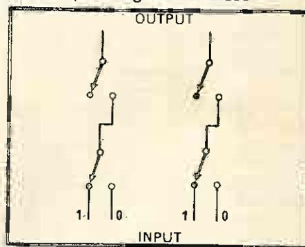
Fig. 4 A TRI-STATE gate may be represented by switches as shown above.
