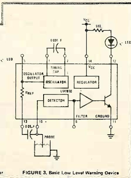
FIGURE 3. Basic Low Level Warning Device
