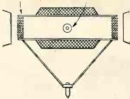
A highly simplified model of how a moving coil cartridge works. The blocks to either side represent the magnets, and the little flocks of circles are the coils.
