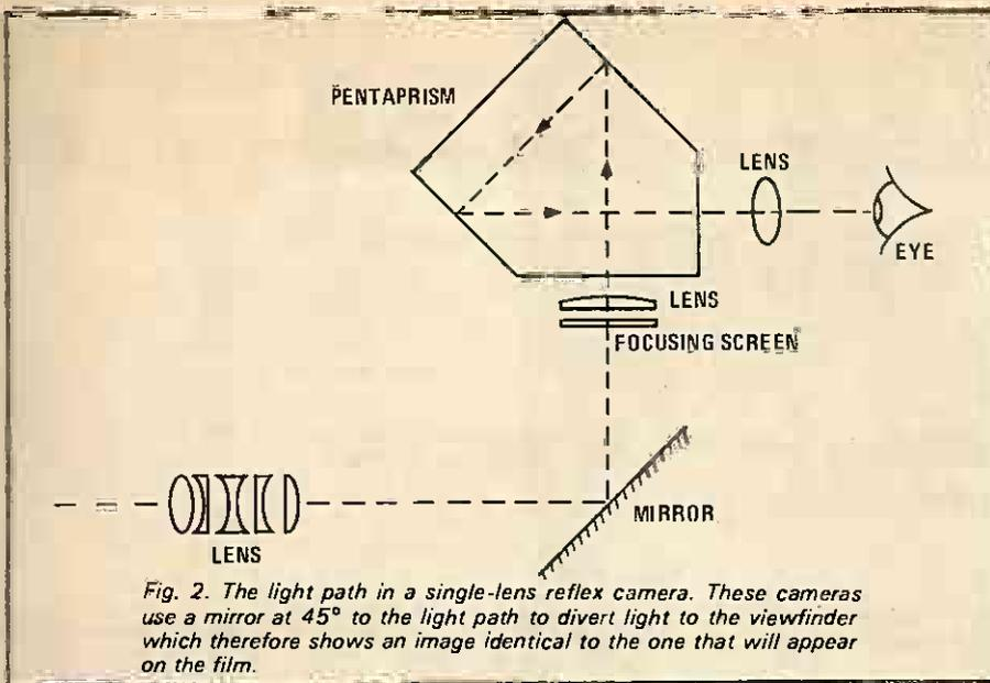
Fig. 2. The light path in a single-lens reflex camera. These cameras use a mirror at 45° to the light path to divert light to the viewfinder which therefore shows an image identical to the one that will appear on the film.
