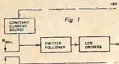
resistance that is higher or lower than that given by the correct moisture content should also be indicated, so five LEDs are incorporated to cover the range of 'too wet' to 'too dry'.
