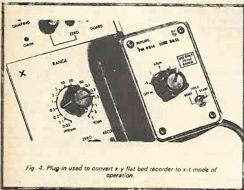
Fig. 4. Plug-in used to convert x-y flat bed recorder to x-t mode of operation.
