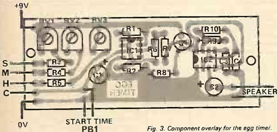
Fig. 3. Component overlay for the egg timer.
