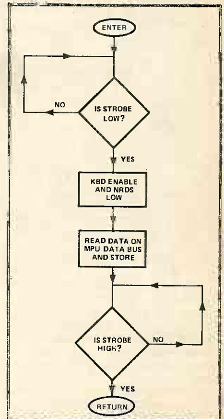
Fig. 2 Flow chart showing routine to implement a read from keyboard operation.
