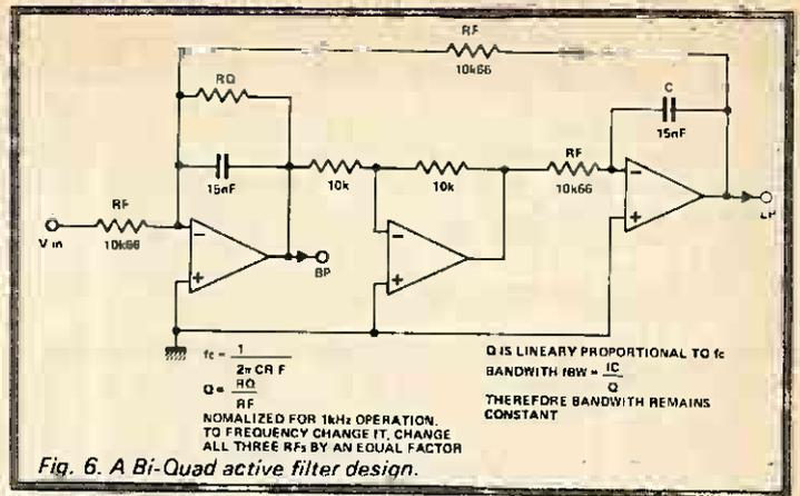
Fig. 6. A Bi-Quad active filter design.
