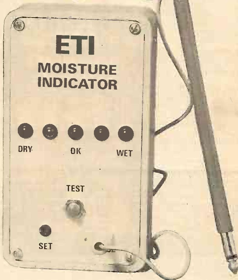
ing the device is the actual 'building up' of the probe. Ours was fabricated from a Japanese 1/4" mono jack plug. Remove the cap, and upon inspecting the contents within, you will see that the tip contact is held in place by what appears to be a splayed rivet.
