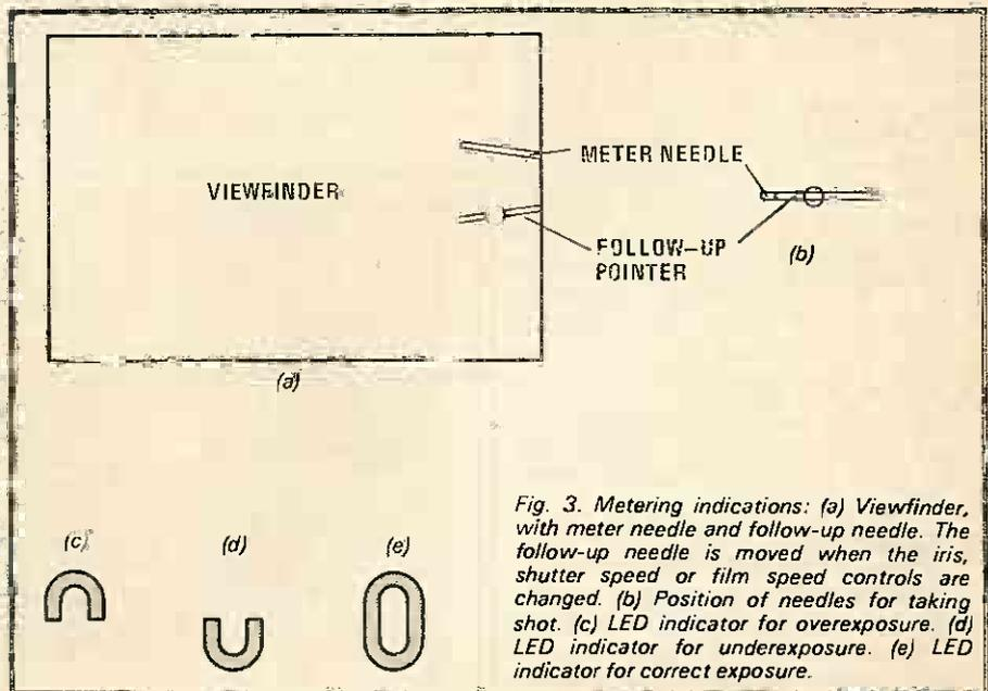
Fig. 3. Metering indications: (a) Viewfinder, with meter needle and follow-up needle. The follow-up needle is moved when the iris, shutter speed or film speed controls are changed. (b) Position of needles for taking shot. (c) LED indicator for overexposure. (d) LED indicator for underexposure. (e) LED indicator for correct exposure.
