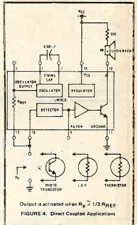
Output is activated when  $R_p \geq 1/3 R_{REF}$
