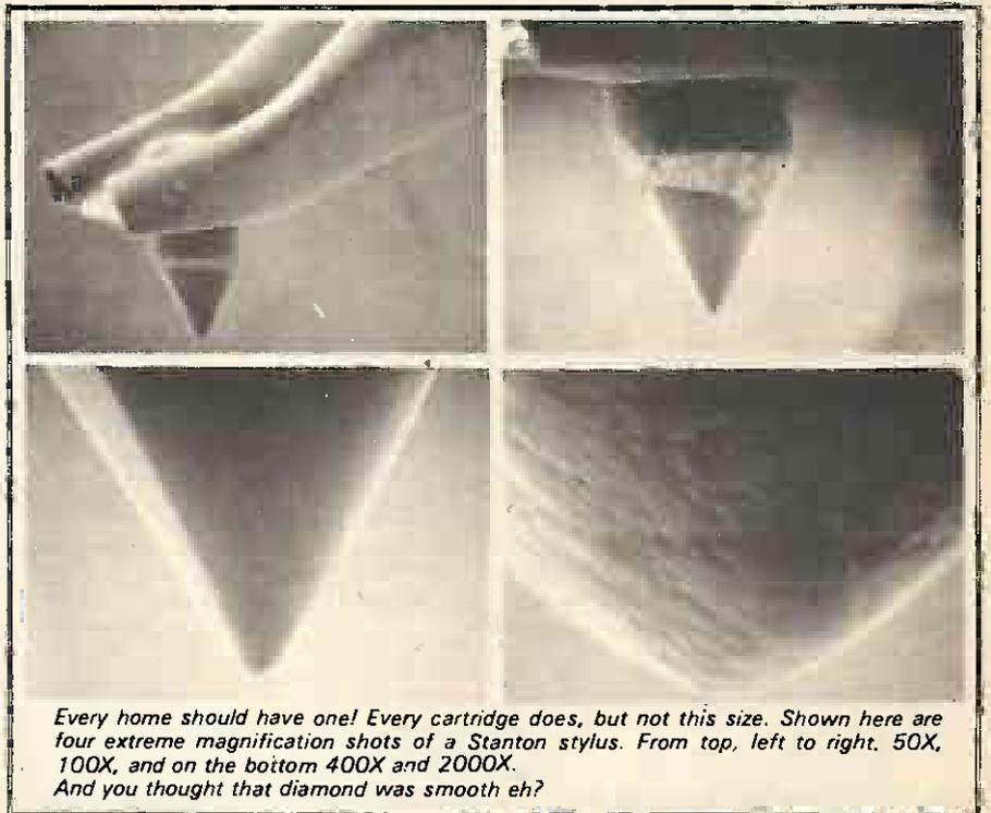
*Every home should have one! Every cartridge does, but not this size. Shown here are four extreme magnification shots of a Stanton stylus. From top, left to right, 50X, 100X, and on the bottom 400X and 2000X. And you thought that diamond was smooth eh?*
