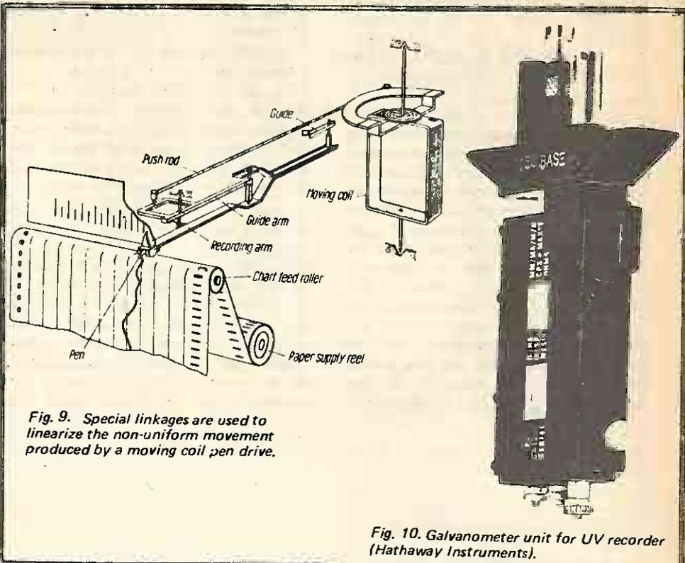
Fig. 9. Special linkages are used to linearize the non-uniform movement produced by a moving coil pen drive.
