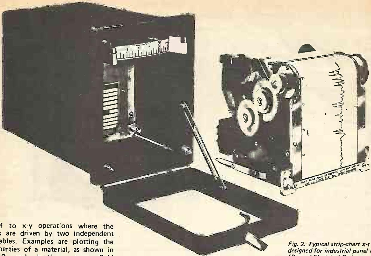
Fig. 2. Typical strip-chart x-t recorder designed for industrial panel mounting. (Record Electrical Co.).
