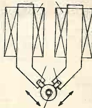
Audio Technica's dual magnet system. On the left an actual stylus assembly, and on the right how that bit in the circle operates, copying the cutting head movements.
