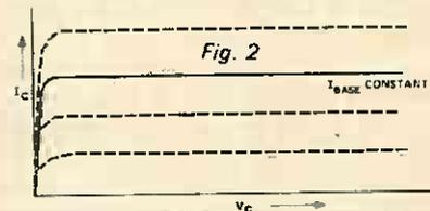
current curve when the base is supplied with a steady value of current and voltage, this voltage being about 0.6 V. In Fig.3 the base voltage is clamped or set by a zener diode to a particular value,
