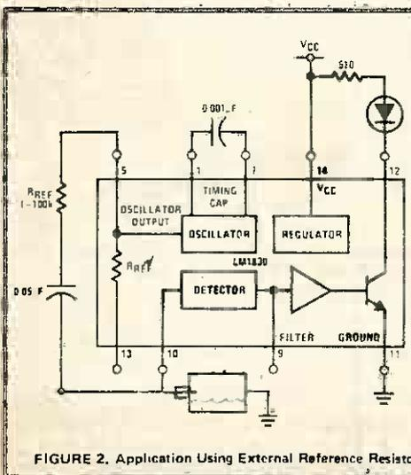
FIGURE 2. Application Using External Reference Resistor
