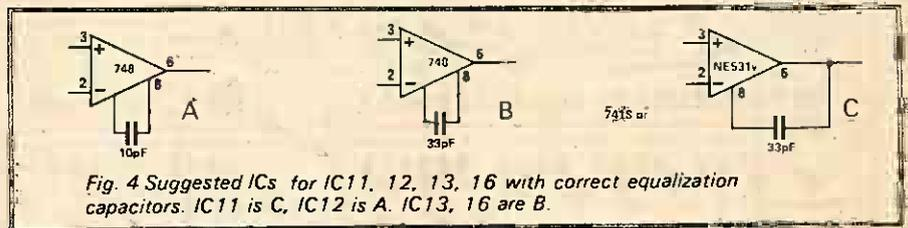
Fig. 4 Suggested ICs for IC11, 12, 13, 16 with correct equalization capacitors. IC11 is C, IC12 is A. IC13, 16 are B.
