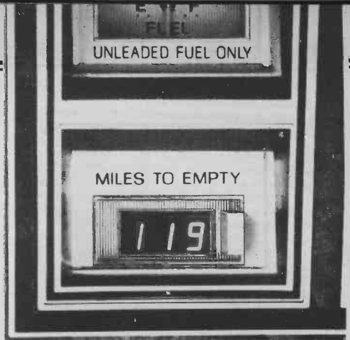
Fig. 5. Fifth among the digital microprocessors in the 1978 cars is the miles-to-empty system used, as an option, in the Lincoln Continental Mark V. Its LSI chip carries the equivalent of 3600 transistors on a surface less than a quarter-inch square. Picking up indications of car speed and fuel tank level, it calculates the distance travelled, fuel used and the resulting miles per gallon. Then it multiplies fuel mileage by the amount of fuel left in the tank to get the miles-to-empty reading shown on the dash.
