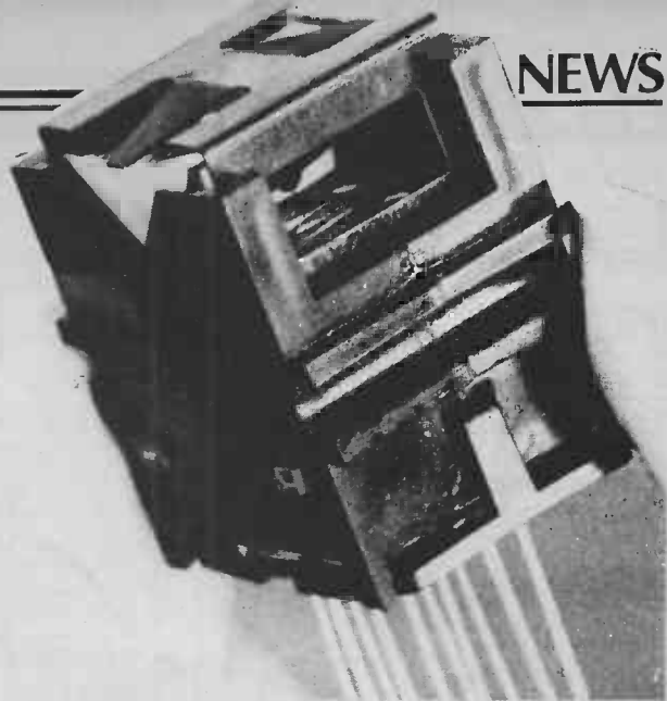
Fig. 2. The Visitronic module, with prism, two lenses and linear IC chips.
