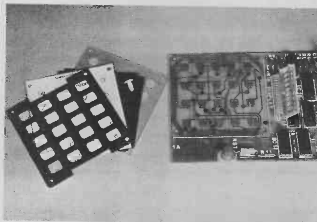
The pieces that go to make up the MK14's keyboard.
