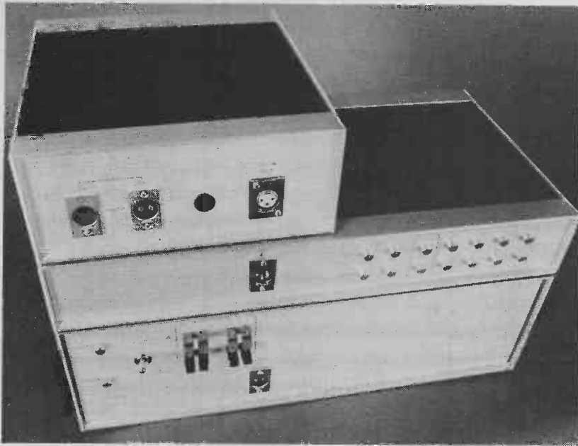
Above: the rear end of the 4000 system. Note the use of Cannon connectors for power.
