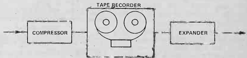
A compander circuit expander-compressor showing how a 2:1 compressor ratio functions in practise to give, in theory, a 100dB S/N ratio from a tape with a 50dB noise 'floor'.
