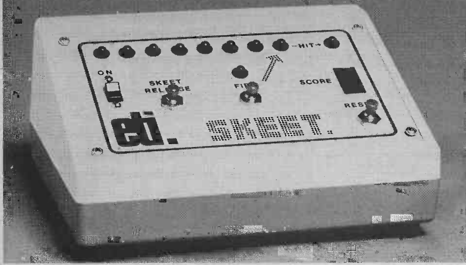
The photograph shows the completed Skeet unit. This shows the layout of the various front panel controls.
