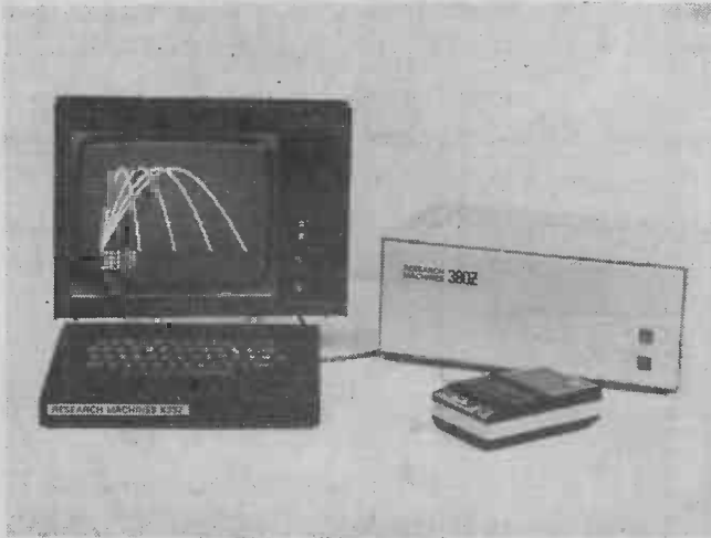
The RESEARCH MACHINES 380Z Computer System in use with an unmodified domestic television and a cassette recorder
