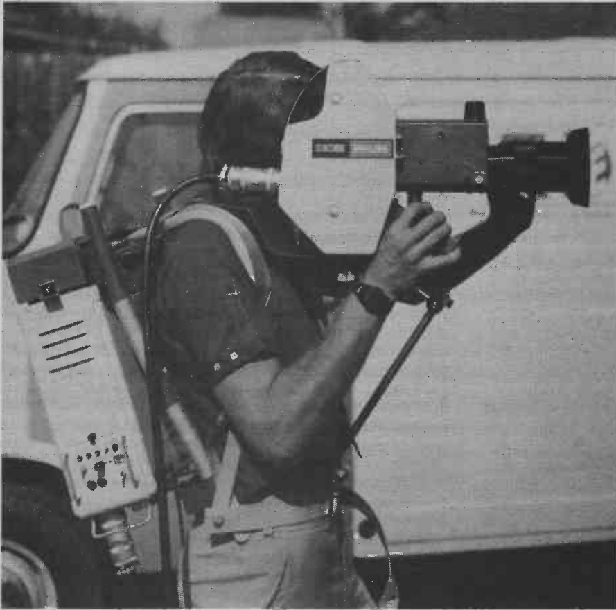
To the left is a picture of the new Philips LDK-11 colour camera.
