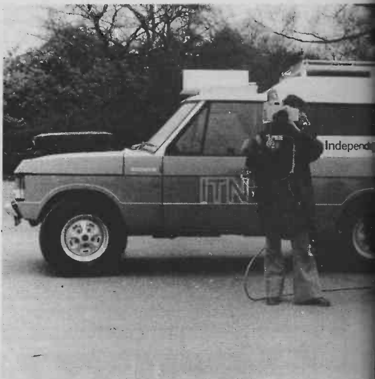
The Independent Television News Landrover based unit with two handheld Fernseh cameras.
