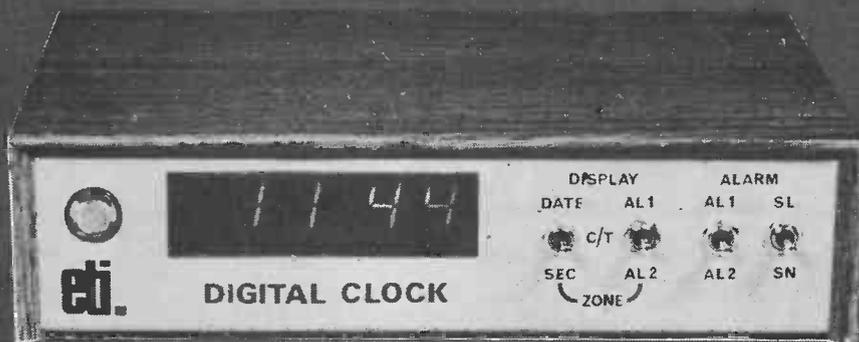
**Concluding our digital clock design is a fluorescent display unit with a battery back-up circuit, brightness control and even a volume control for the alarm. As an extra a four year calendar is also included.**
