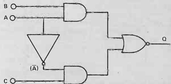
IF B=1 AND C=1, THEN A CHANGE OF A FROM 1 TO 0 CAUSES A BRIEF PULSE AT Q.
