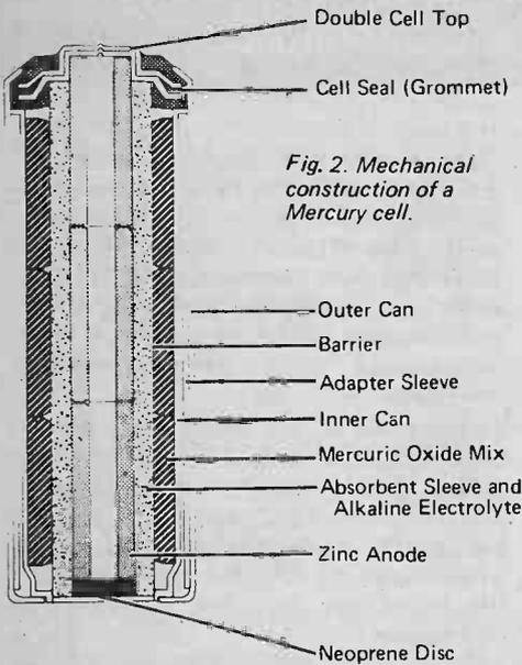
Fig. 2. Mechanical construction of a Mercury cell.
