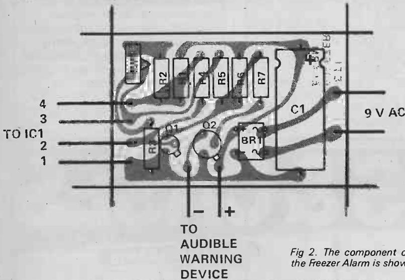
Fig 2. The component overlay for the Freezer Alarm is shown above.
