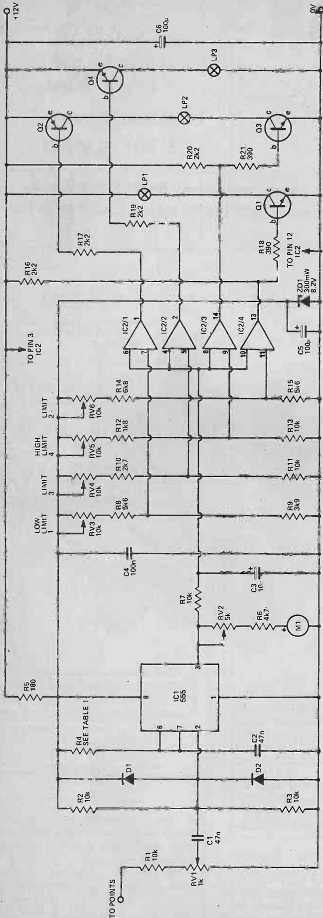
Fig. 1. Circuit diagram of the rev. monitor - counter.
