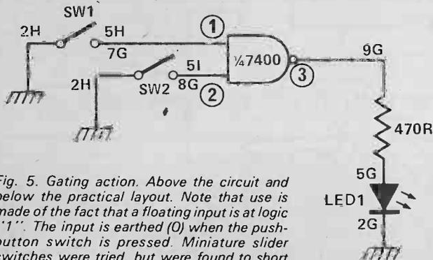
Fig. 5. Gating action. Above the circuit and below the practical layout. Note that use is made of the fact that a floating input is at logic "1". The input is earthed (0) when the push-button switch is pressed. Miniature slider switches were tried, but were found to short momentarily between the 1 and 0 positions.
