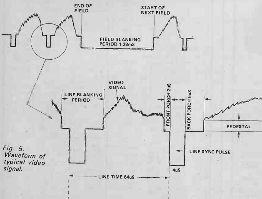
Fig. 5. Waveform of typical video signal.
