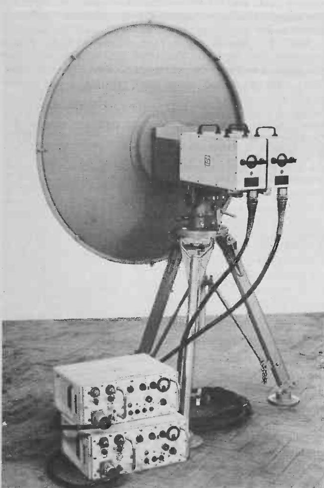
microwave link (or sound-in-synchs), and a VHF communications transmitter in North London for the return circuit. Thus the OB can sit in a field with its own generator and full communication facilities without having to disturb the Post Office. Incidentally, when requested to do so by the right people, the PO can provide a telephone virtually anywhere in a road or car park within a couple of hours.
