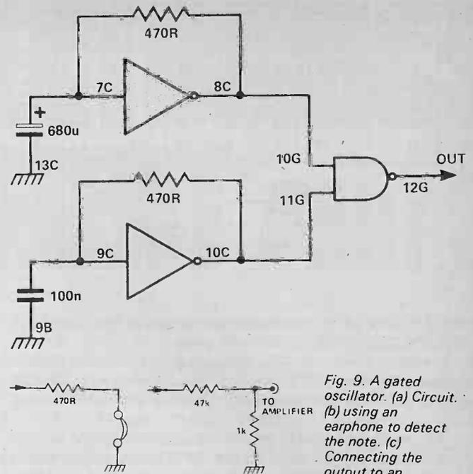
Fig. 9. A gated oscillator. (a) Circuit. (b) using an earphone to detect the note. (c) Connecting the output to an amplifier.
