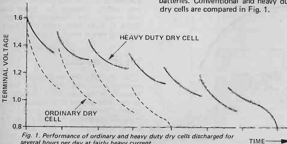
Fig. 1. Performance of ordinary and heavy duty dry cells discharged for several hours per day at fairly heavy current.
