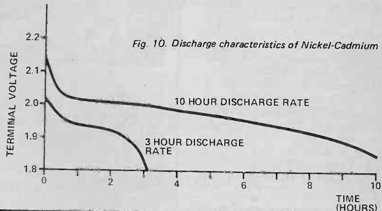
Fig. 10. Discharge characteristics of Nickel-Cadmium cells.
