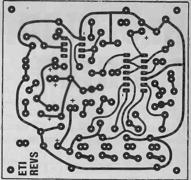
The outputs of IC2 control the transistors Q1 to Q4 which handle the current required by the lamps. If the rpm is below the lower limit Q1 and Q3 will be on lighting LP1 but as Q2 is off LP2 will be off. Above the first limit Q2 will be turned on and so LP2. Above the next limit Q1 and LP1 will turn off, above the next Q4 and LP3 will turn on, and finally when the upper limit is reached Q3 will turn off LP2 leaving only LP3 on.
