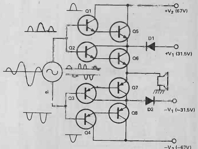
because in the former circuit each transistor in the output stage is working close to its optimum efficiency point *all* of the time, while in class B this only occurs close to rated output power.
