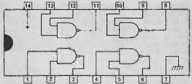
7400, using single strand insulated wire. Use the LED which is connected to pin 3 of the 7400 as an indicator.
