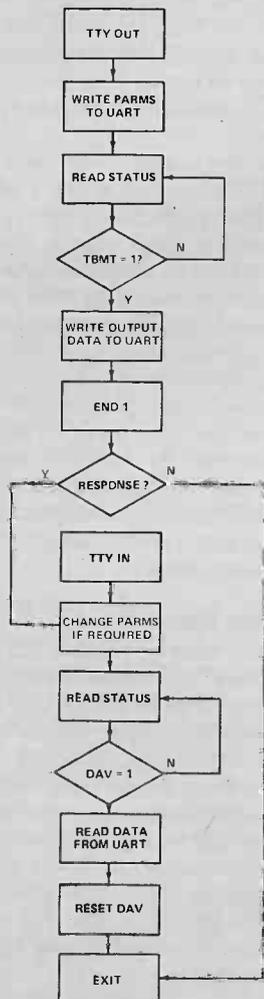
I/O sub-routine. When the DAV bit goes to logic 1 it indicates that a complete word is available at the UART for the MPU. The MPU now reads that data word and then writes to the RESET DAV address to cause the DAV signal to be reset. With the data word input still in the accumulator the logic reaches the EXIT and returns control to the calling program.
