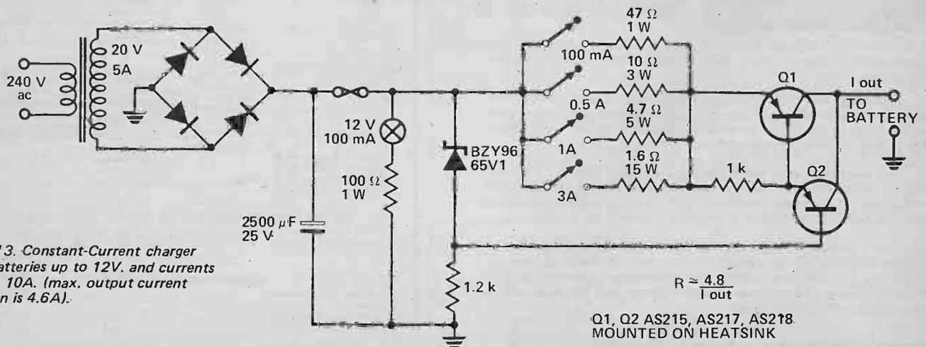
Fig. 13. Constant-Current charger for batteries up to 12V, and currents up to 10A. (max. output current shown is 4.6A).
