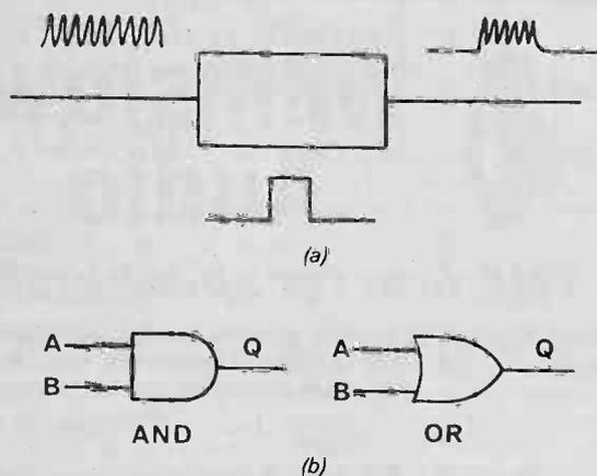
Fig. 1. Gates. (a) General gating action. (b) Logic gate symbols.
