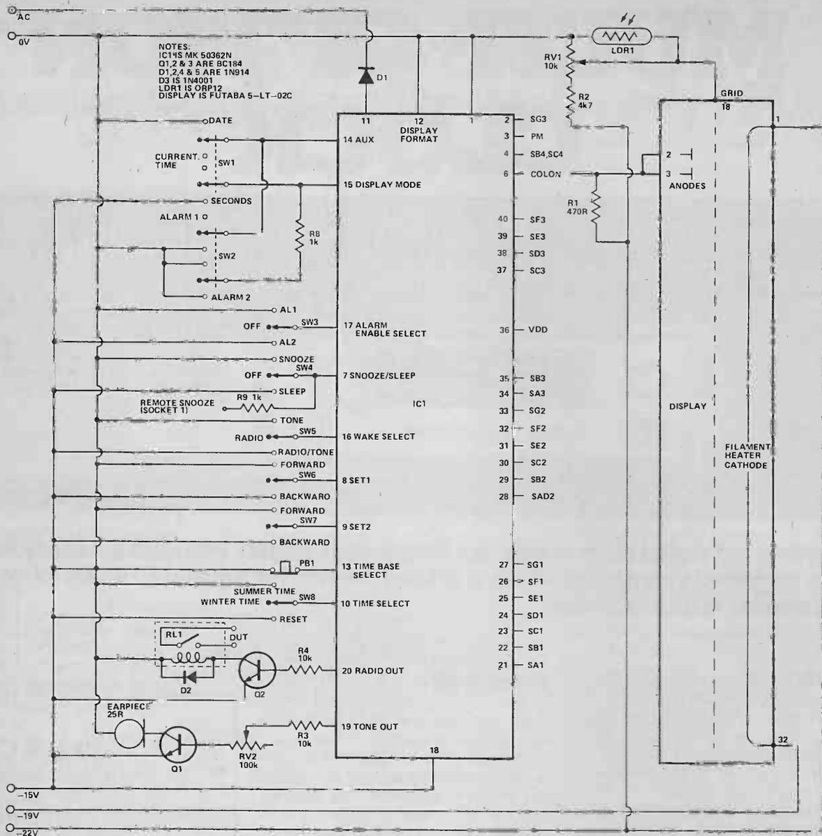
Fig 1 (above). Circuit diagram for the clock. The reed relay should be a 12V-18V type and is available from Doram.
