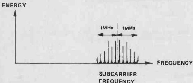
c) Modulating a high frequency (subcarrier) by a colour difference signal produces sidebands to  $\pm 1$  MHz.
