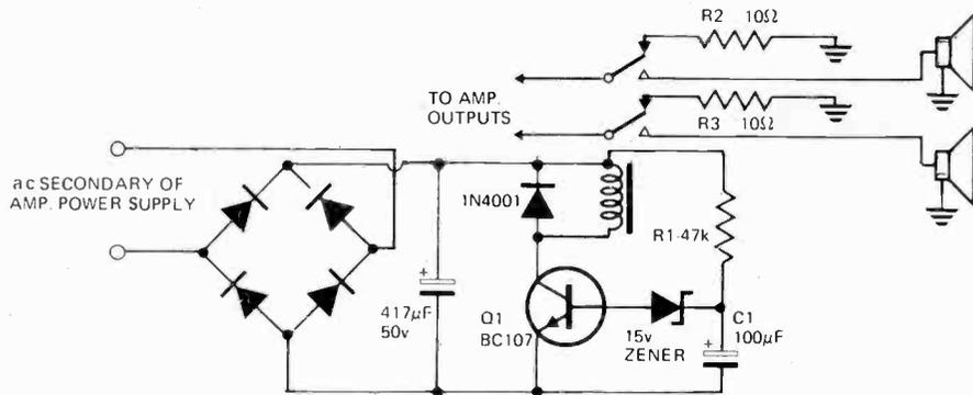
Many hi-fi amplifiers cause an only-too audible 'plop' in the speakers when switched on. The 'plop' is not only disconcerting but can also be damaging to low-power capacity speakers.
