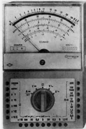
A second version of the instrument is available with an additional internal universal signal injector. The USI version provides a modulated r.f. output rich in harmonics up to uhf.
