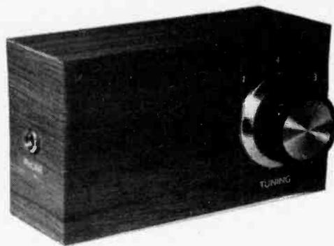
The only active device in this ingenious medium wave design is a single integrated circuit. The receiver is powered by a 1.5 volt cell and current consumption is exceptionally low.
