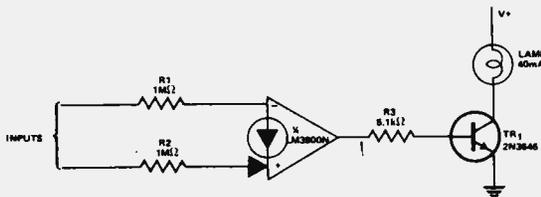
Fig. 12. A voltage comparator with an indicator lamp.
