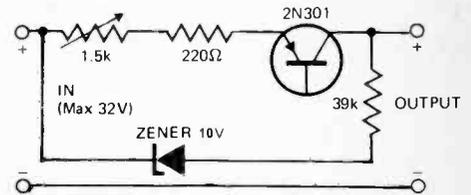
A series transistor is used as a variable resistor for this constant current supply.
