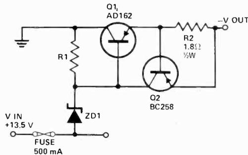
These short-circuit protected stabilisers give 6, 7.5 and 9 V from an automobile battery supply of 13.5 V nominal, however, they will function just as well if connected to a smoothed dc output from a transformer/rectifier circuit.
