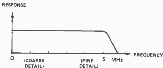
Fig. 13. a) To ensure a luminance signal does not occupy excessive bandwidth it is passed through a filter of the response shown, which permits adequate picture resolution.
