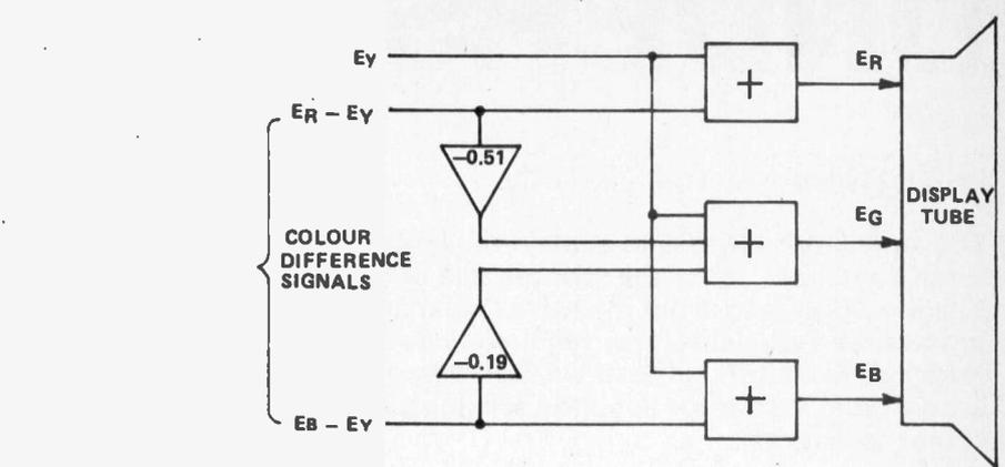
Fig. 10. Process by which a receiver reconstructs the primary colour signals required by the display tube from the luminance signal E<sub>Y</sub> plus the two colour difference signals.
