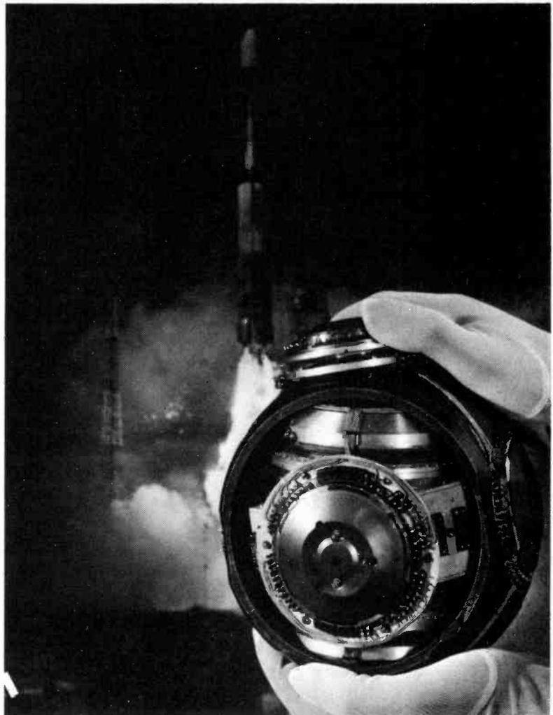
This is the sensing element of the inertial guidance system used in the ELDO satellite launch vehicle. This was developed by Ferranti in 1969 when ELDO decided that an onboard navigation system was needed to replace ground control. Previously the vehicles had only attitude monitoring equipment.
