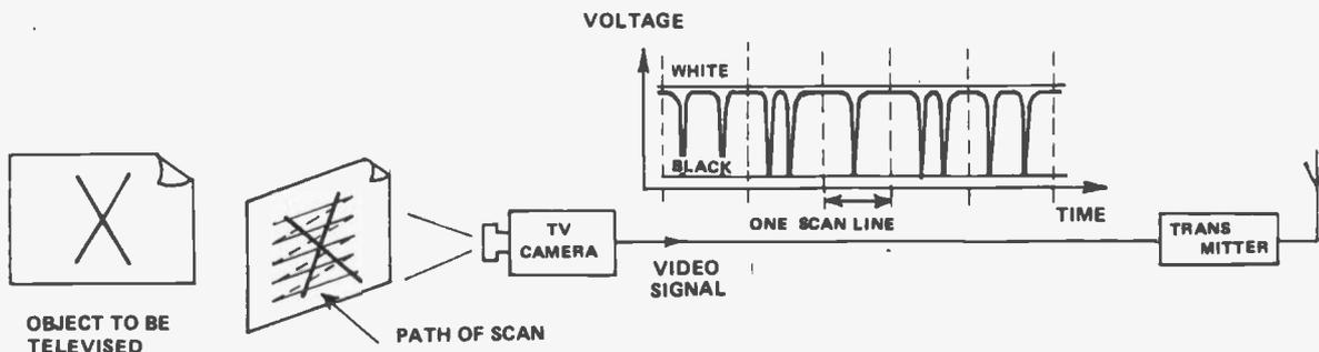
Fig. 11. Principle of tv scanning. The flyback at the end of a scan line to the start of the next is assumed to be instantaneous.
