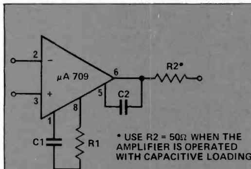
\* USE  $R_2 = 50\Omega$  WHEN THE AMPLIFIER IS OPERATED WITH CAPACITIVE LOADING
