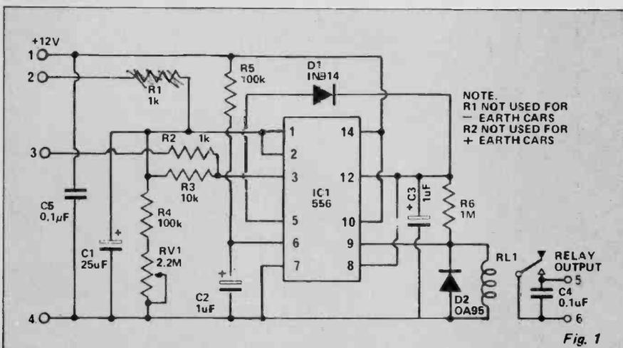
taken by adding further alarm microswitches. For example microswitches may be fitted to the suspension such that if anyone tries to lift the car, in order to tow it away, the alarm will go off. If such switches are used they should be connected between terminal 2 or 3 of the alarm (see Fig 1 and 2), depending on whether the vehicle has a positive or negative earth system, and earth.
