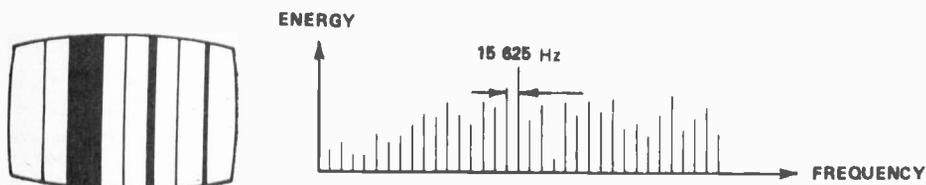
b) A scene containing only horizontal detail would cause a luminance signal containing only harmonic frequencies of 15 625 Hz.
