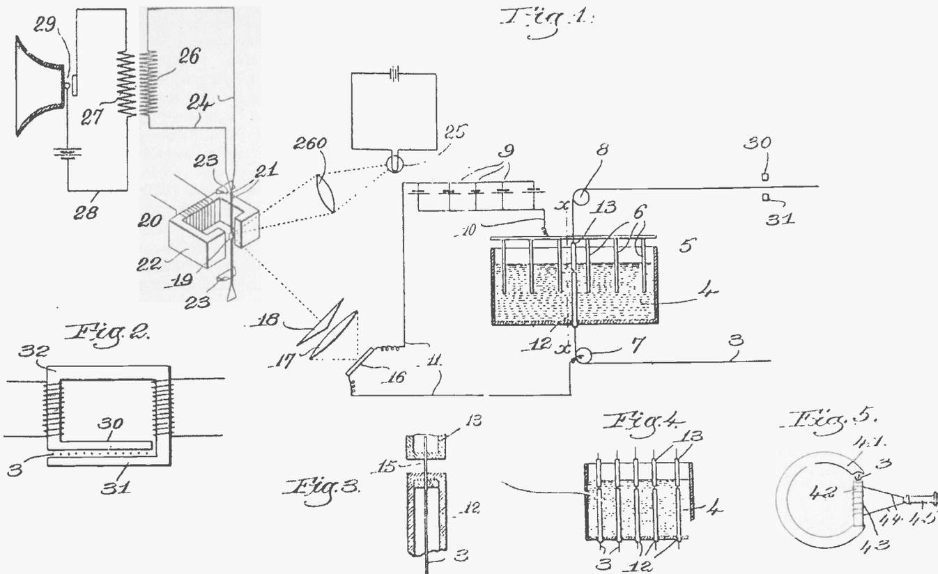
British Patent No. 22962 of 1908. A magnetic recording system with which recorded sounds vary the electrolytic deposition of magnetic material on a wire.
