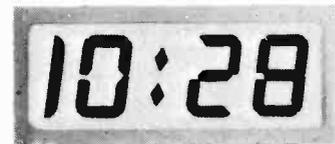
All the liquid crystal displays in field effect technology have dark symbols on a light background and are suitable for reflection operation, all with high contrast ratios, low operating voltage and low power draw. Such features allow the displays to be driven by CMOS and other ICs.
