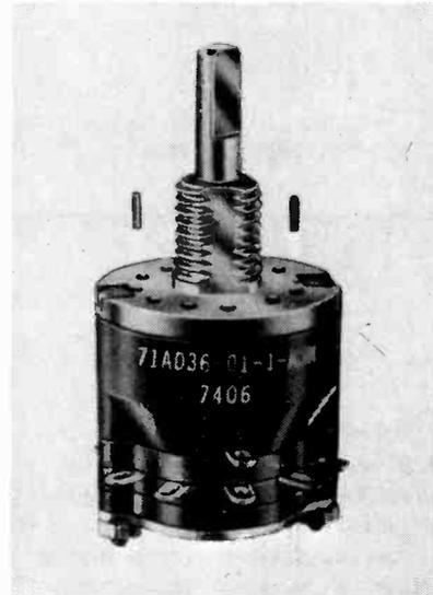
Miniature rotary switches with adjustable stops are available from Highland Electronics Limited (33 Dallington Street, London EC1V 0BD). The position of the stops can easily be changed from front of switch, which is available with 30° or 36° index angles, one to four poles per deck and up to 12 decks per switch. This 0.75 in diameter series is coded "71AD".
