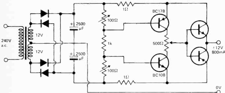
A variable power supply using complementary output transistors is capable of swinging the voltage at the output from +12 V through zero to -12 V.
