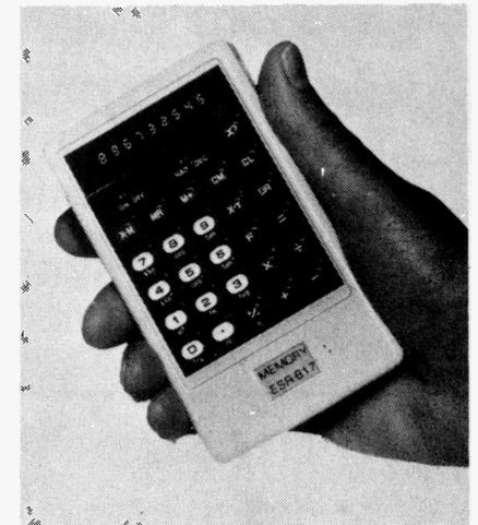
All the numerical entry keys have double functions. Additional features include chain operation, constant operation with any arithmetical function mode and a memory with an accumulating capability. Also when overflow in mid calculation is indicated, calculations can proceed to 8 figure accuracy by using the clear key.
