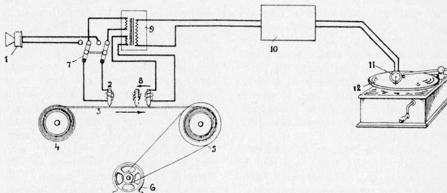
British Patent No. 328721 (1929). Recording phonographic records from a magnetic tape master. A second playback head is provided to give an echo effect.
