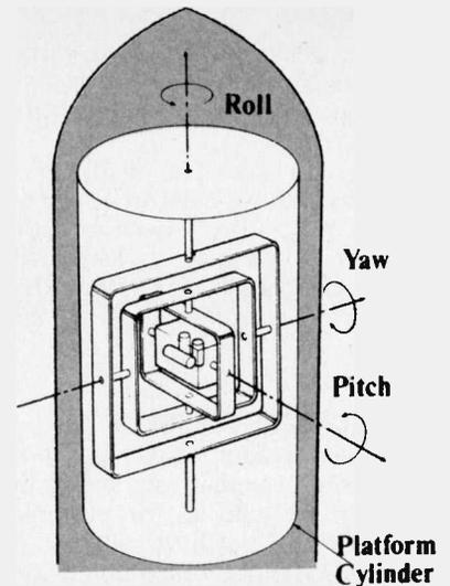
Fig. 5. Orientation of the gimbals at the launch of the Black Arrow launch vehicle which put "Prospero" (Britain's first technology satellite) into orbit in 1971.
