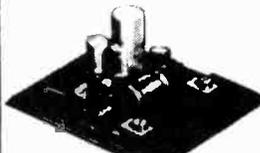
The AL10, AL20 and AL30 units are similar in their appearance and in their general specification. However, careful selection of the plastic power devices has resulted in a range of output powers from 3 to 10 watts R.M.S. The versatility of their design makes them ideal for use in record players, tape recorders, stereo amplifiers and cassette and cartridge tape players in the car and at home.
