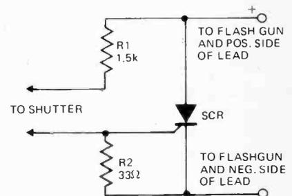
This three component device will keep sparks out of your camera shutter, when using a flash gun, by letting an SCR carry the firing current.
