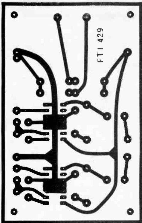
Fig. 5. Printed circuit board. Full size 97 x 61mm.
