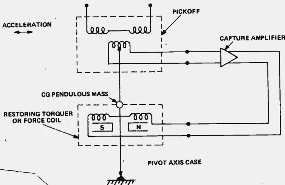
ical force balance pendulous accelerometer utilizes a differential transformer type gain capture amplifier, and a dc permanent magnet force coil. These features many of the high precision force-balance accelerometers currently manufactured.
