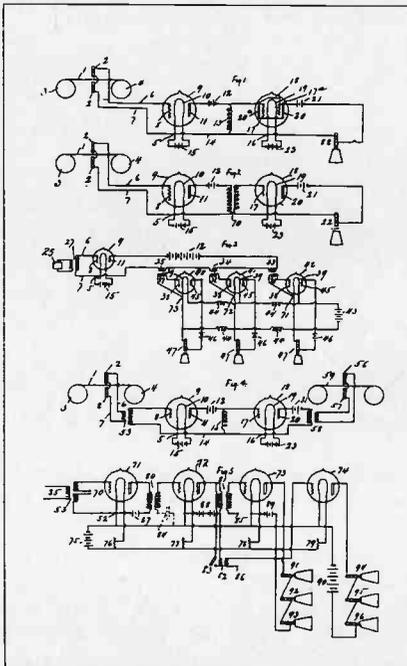
British Patent No. 2059 of 1914. de Forest's use of the 'audion' or triode valve to amplify tape recorder playback volume.
