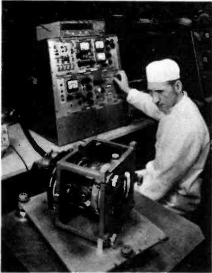
Testing an Inertial Platform at the Edinburgh Labs. of Ferranti.
