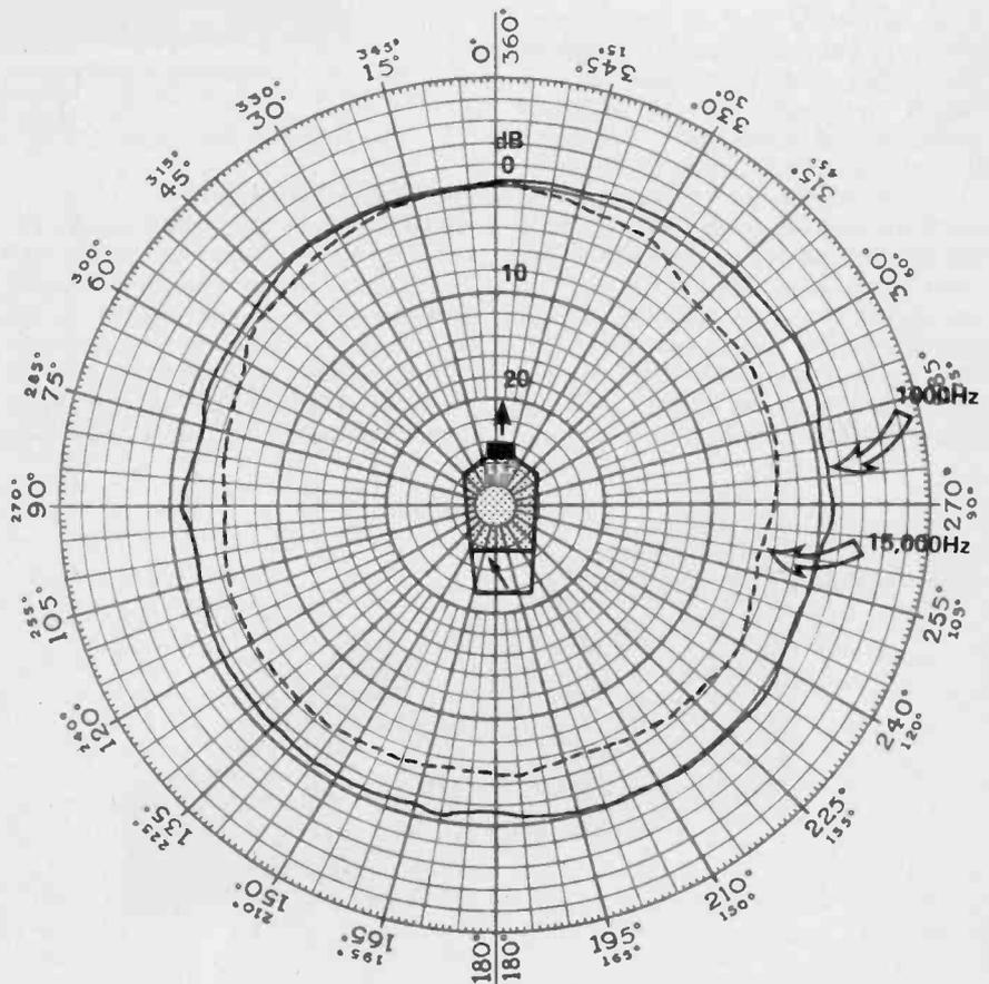
Fig. 1. Polar response of Realistic Sound Level Meter at 1000 and 15,000Hz.
