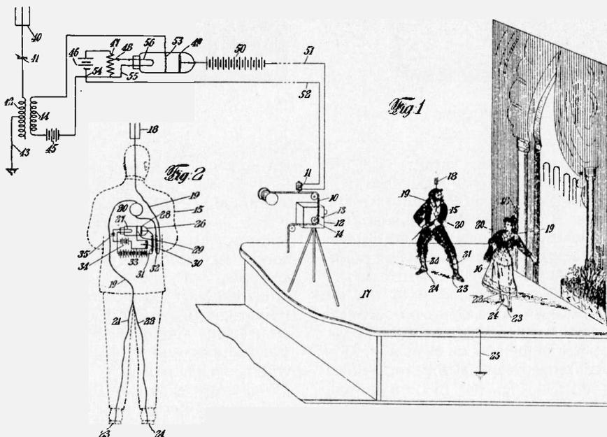
British Patent No. 107167 (1917). Magnetic recording techniques used in cinematography. Each actor has a microphone and portable transmitter. The transmitters have rather prominent aerials and are earthed via connections on the actors feet and a conductive stage.
