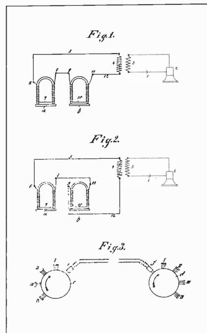
British Patent No. 888 of 1900. Pedersen's use of a magnetic recording system to transmit several telephone messages simultaneously over the same wire.
