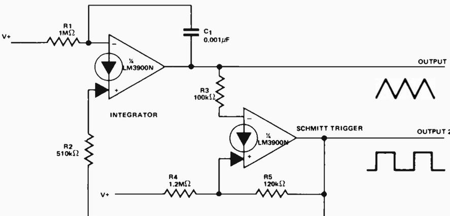
Fig. 10. A circuit for generating triangular and square-wave.
