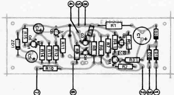
Fig. 6. Component overlay for the phase-proportional controller.
