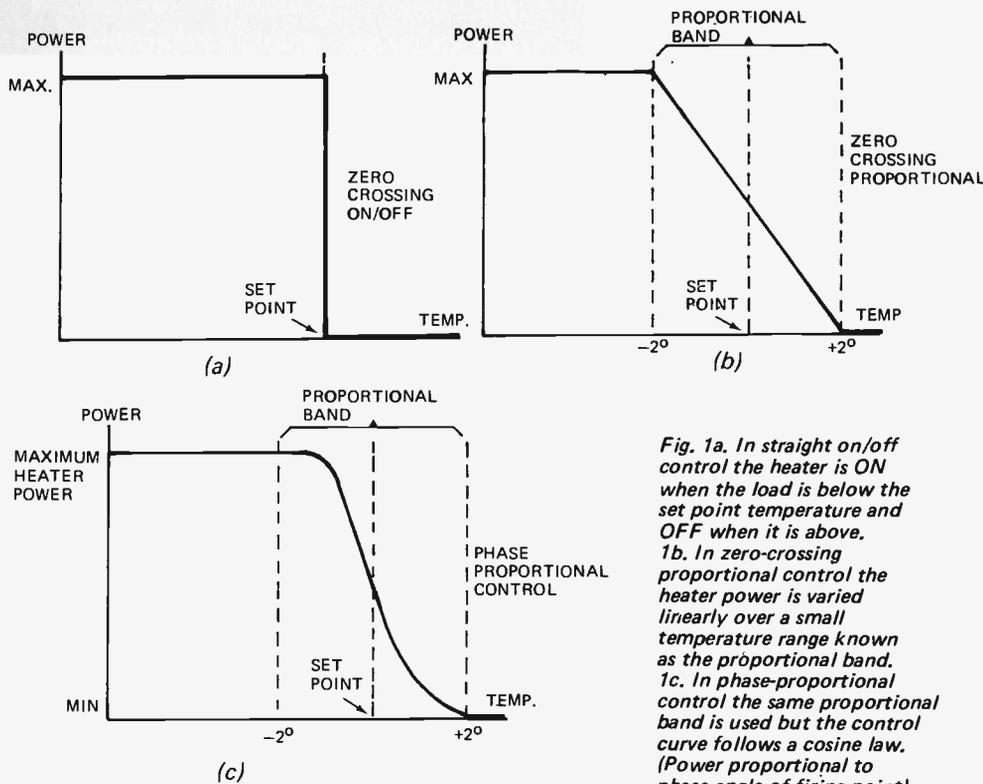
Fig. 1a. In straight on/off control the heater is ON when the load is below the set point temperature and OFF when it is above. 1b. In zero-crossing proportional control the heater power is varied linearly over a small temperature range known as the proportional band. 1c. In phase-proportional control the same proportional band is used but the control curve follows a cosine law. (Power proportional to phase angle of firing point).
