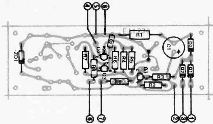
Fig. 5. Component overlay for the zero-crossing controllers. Note that for ON/OFF control some components are not fitted (refer Fig. 4).
