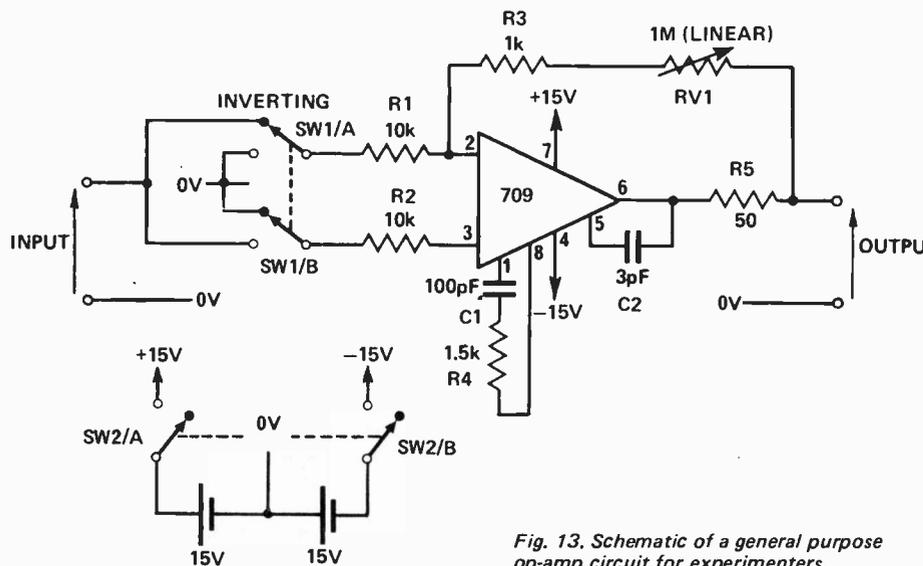
Fig. 13. Schematic of a general purpose op-amp circuit for experimenters.
