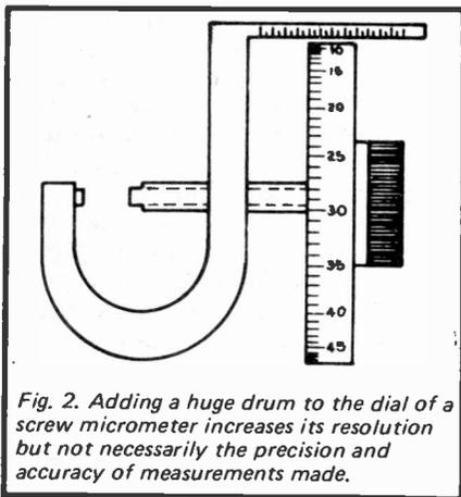
Fig. 2. Adding a huge drum to the dial of a screw micrometer increases its resolution but not necessarily the precision and accuracy of measurements made.
