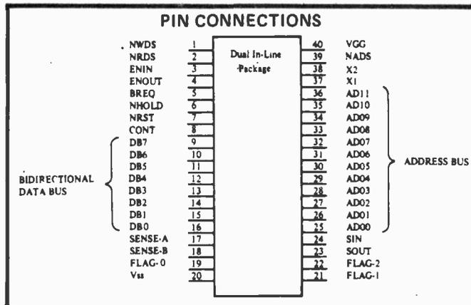
NWDS is an output to indicate to peripherals that CPU data is now valid, ie WRITE.
