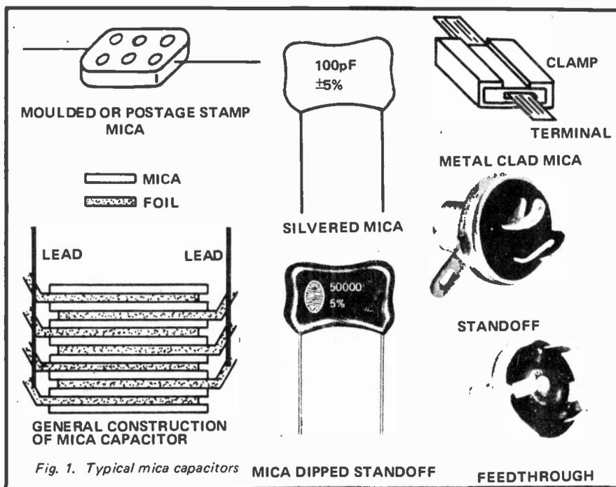
Fig. 1. Typical mica capacitors
