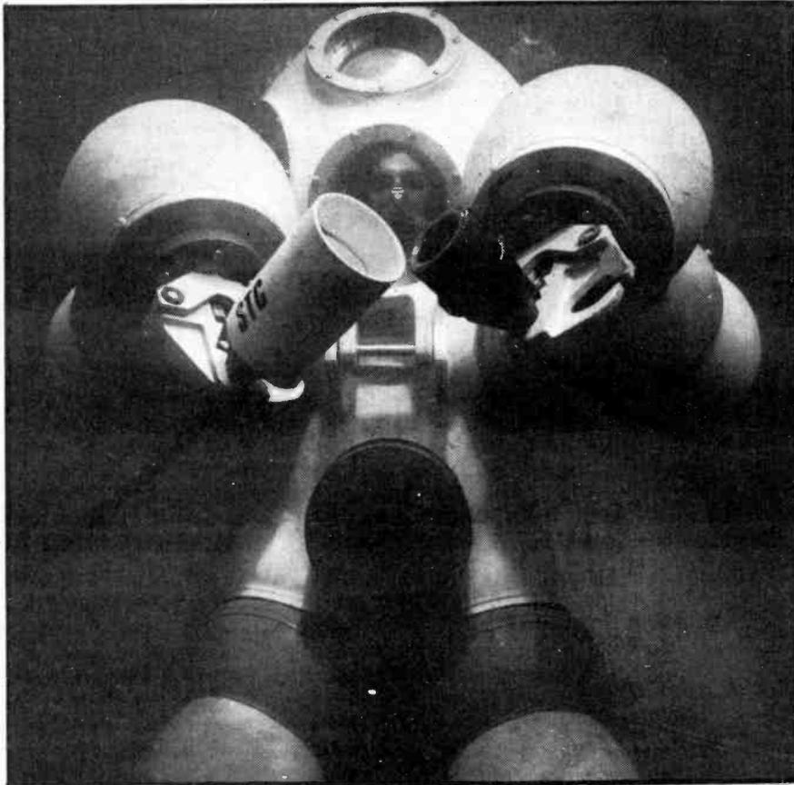
The picture shows the testing of a new STC underwater cable, which is unpluggable whilst live. It can operate at depths where the pressure is in excess of 700 p.s.i. Hence the 'Flash Gordon' repairman suit.
