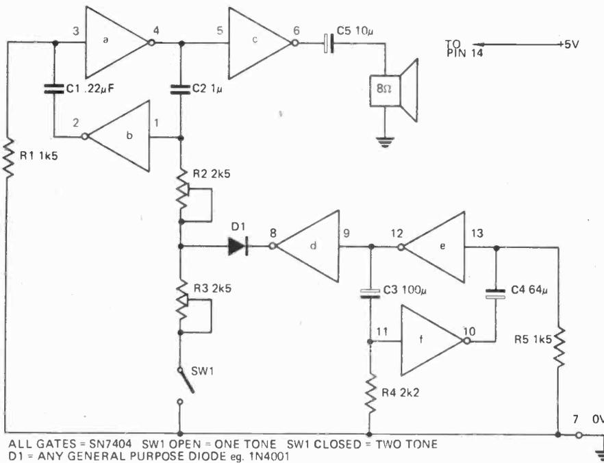
This simple circuit uses only 1 SN7404 IC and can either generate an altering two tone signal or a pulsed single tone, either of the two tones can be varied and the circuit will drive a loudspeaker or a crystal earpiece.
