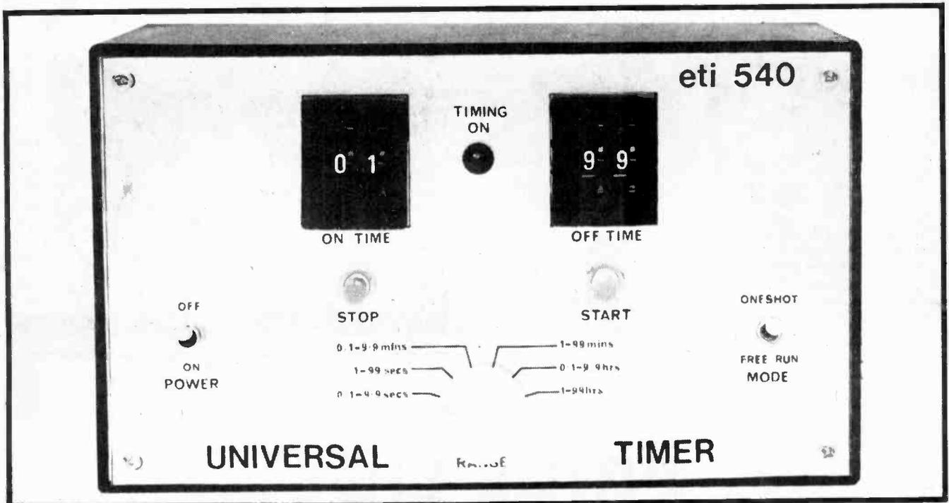
One tenth of a second to 99 hours. Both on and off times programmable. Manual or automatic operation, resettable at any time.
