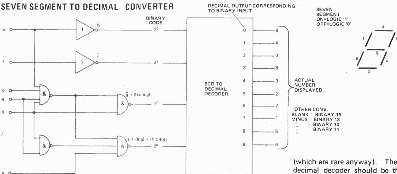
Note that the output from the gates is not 'straight' BCD so the outputs from the BCD to decimal decoder are
