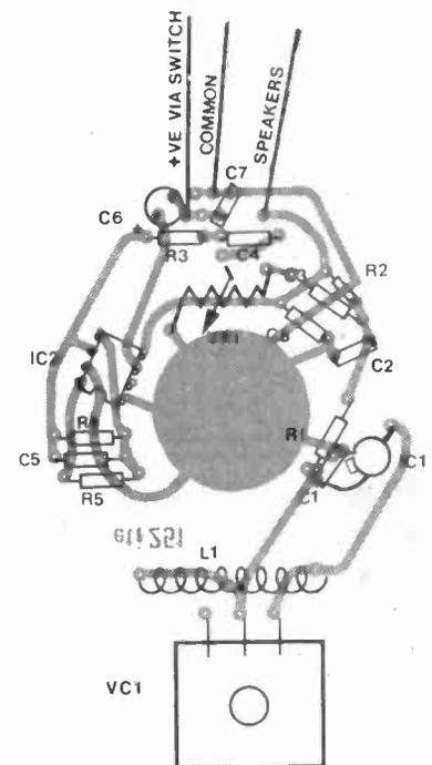
Fig. 3. Component overlay.
