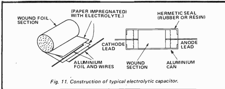
Fig. 11. Construction of typical electrolytic capacitor.
