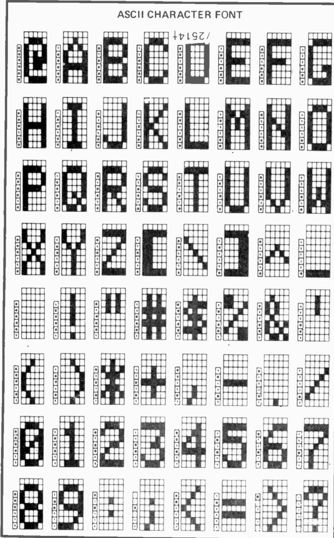
The Signetics 2513 is a high speed 2560-bit Static ROM available in 64x7x5, 64x8x5, and 512x5 versions. The product uses +5V, -5V and -12V power supplies, 5V TTL level input signals and Tri-State-Outputs for direct, low cost interfacing with TTL, DTL and MOS.
