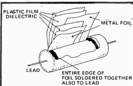
Fig 4 How polystyrene capacitors are made
