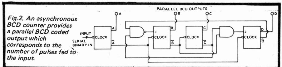
Fig. 2. An asynchronous BCD counter provides a parallel BCD coded output which corresponds to the number of pulses fed to the input.
