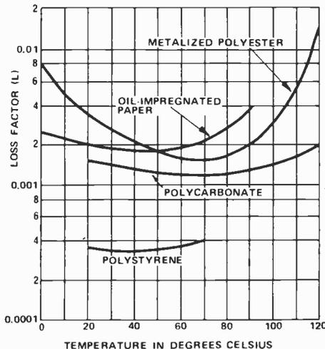
Fig. 8. Temperature versus loss factor.
