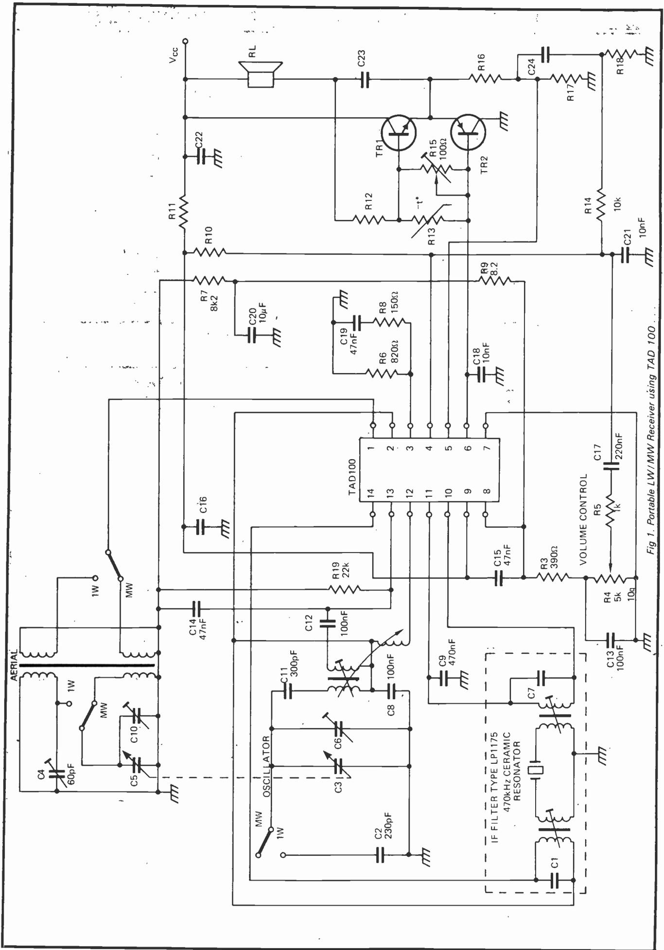
Fig 1. Portable LW/MW Receiver using TAD 100 . . .
