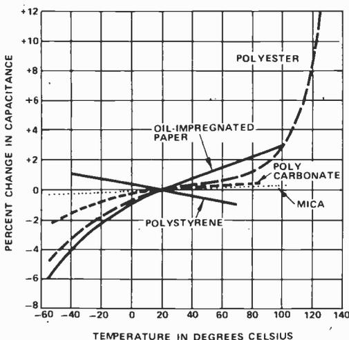
Fig. 7. Temperature versus change in capacitance.
