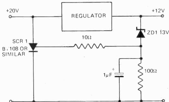
When using a regulated PSU to reduce a supply voltage there is always the
