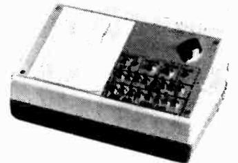
Full constructional details will be given next month for this low-cost video display unit. Primarily intended for microcomputer input/output, it can also be used for paging systems or to display scores for electronic games. Use your imagination; the ETI 560 makes it possible!
