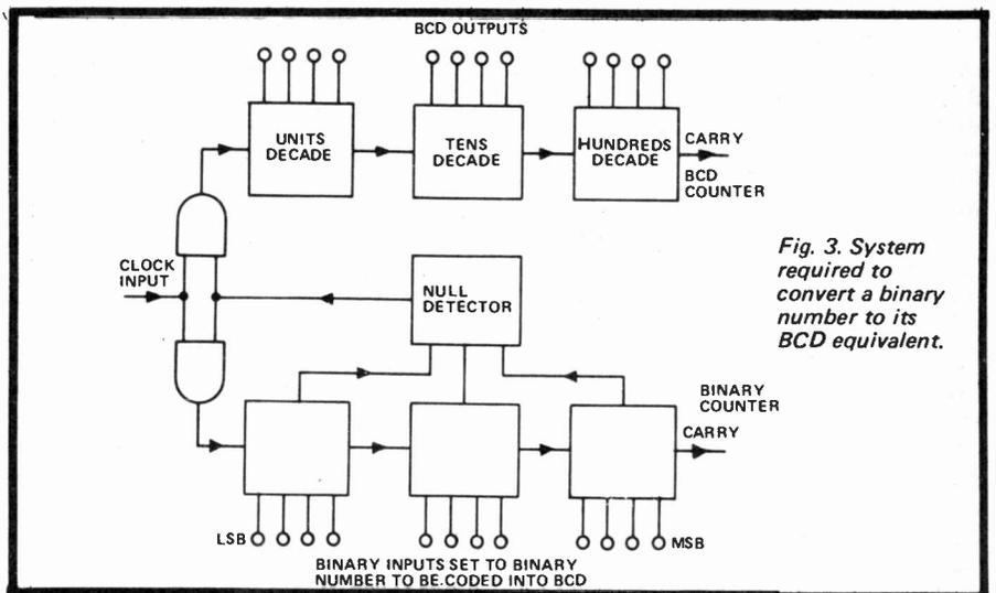
Fig. 3. System required to convert a binary number to its BCD equivalent.
