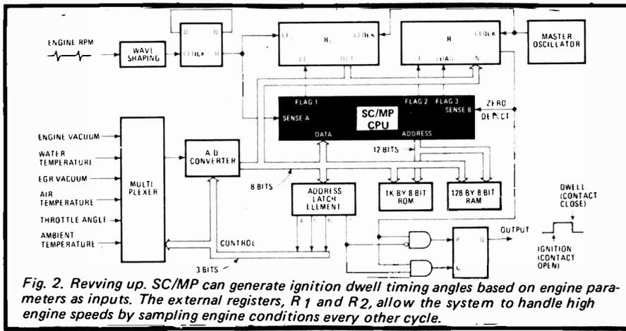
Fig. 2. Revving up. SC/MP can generate ignition dwell timing angles based on engine parameters as inputs. The external registers, R1 and R2, allow the system to handle high engine speeds by sampling engine conditions every other cycle.
