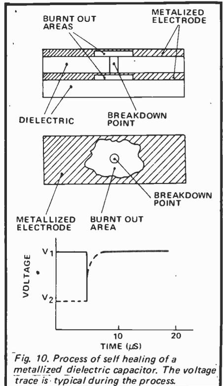
Fig. 10. Process of self healing of a metallized dielectric capacitor. The voltage trace is typical during the process.
