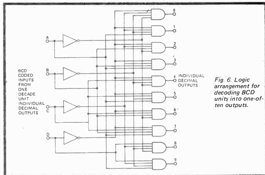
Fig. 6. Logic arrangement for decoding BCD units into one-of-ten outputs.
