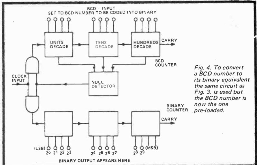
Fig. 4. To convert a BCD number to its binary equivalent the same circuit as Fig. 3. is used but the BCD number is now the one pre-loaded.
