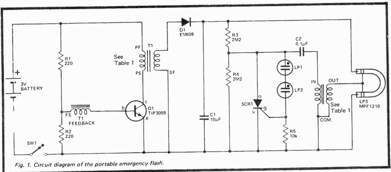
Fig. 1. Circuit diagram of the portable emergency flash.
