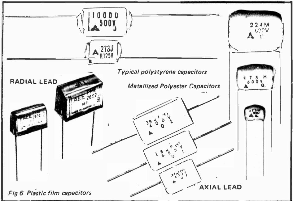
Fig 6 Plastic film capacitors
