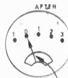
ONLY ADJUST METER IF IT IS OF THE MOVING IRON TYPE DO NOT ADJUST IF IT IS A MOVING COIL TYPE
