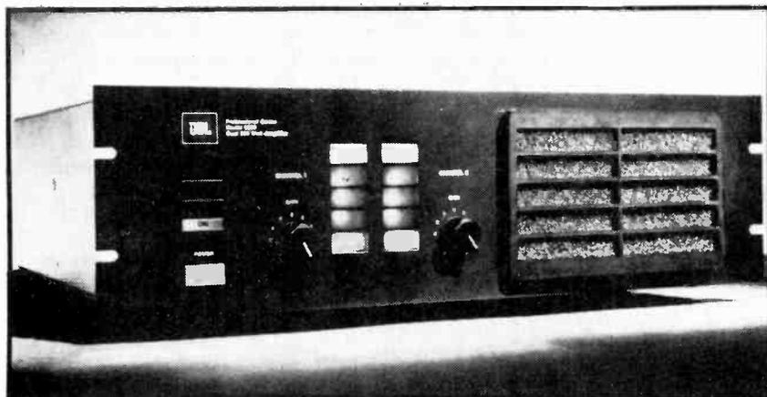
The 6233 a new ultra high power  $\approx 200W$  per channel ( $8\Omega$  : FCC) professional amp from JBL. It boasts power metering, fan cooling and a fully complementary output stage consisting of 12 150W transistors per channel. The power supply is novel — a 2000W inverter is employed rather than a transformer and rectifier — to keep down size and weight. If you feel you need this piece of monumental suicide engineering — JBL will relieve you of £1100 for the pleasure of its company.
