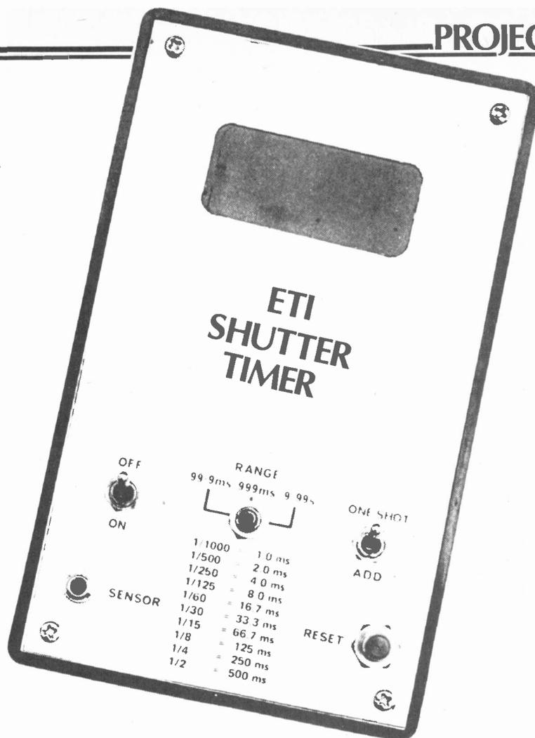
It is suitable for checking cameras with a hinged or removable back so that the sensor can be placed in the film plane. For cameras where the film fits into a slot this unit cannot be used.
