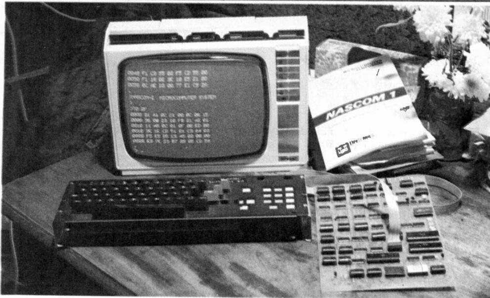
The photograph on the left shows the NASCOM 1 single board computer. The user requires only a standard TV receiver and a cassette recorder to complete a powerful and versatile home computer system.
