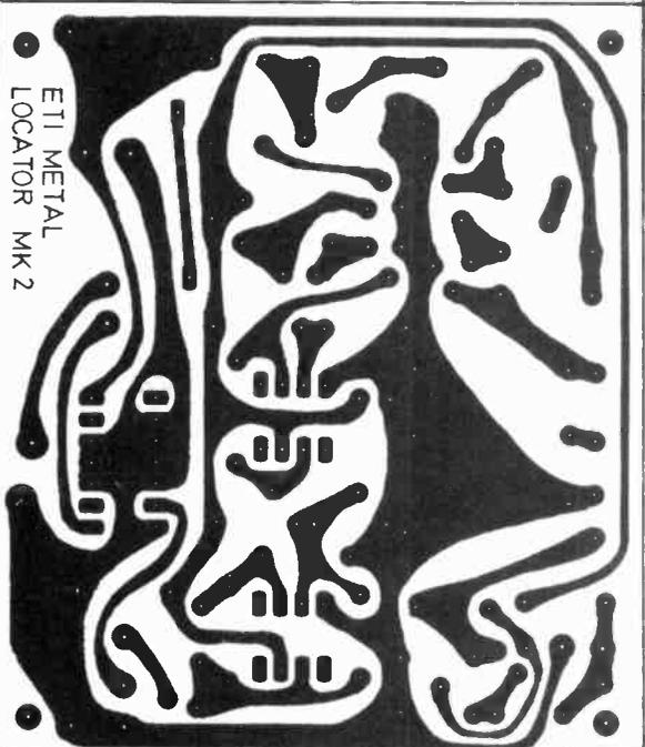
Fig 4. The PCB for the IB Mk 2. Full size is 89 x 77 mm.
