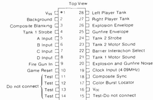
Fig 3. 8710 pinout.
