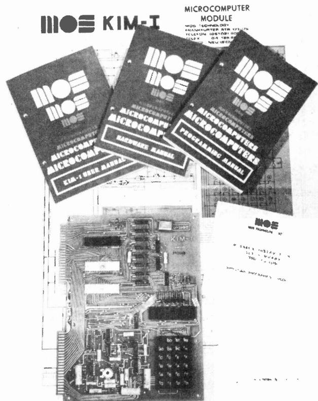
**KIM1 together with the three excellent manuals supplied with the kit, the "wall chart" circuit diagram and the MPU reference guide.**
