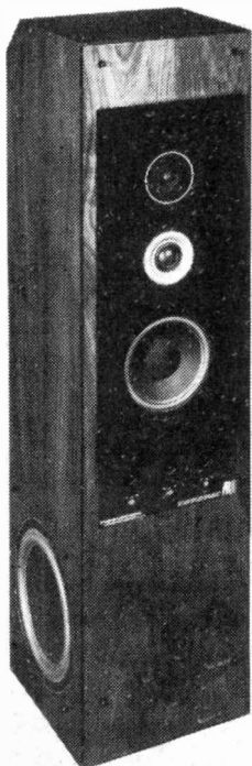
The AR9. Coming from one of the 'founder' manufacturers it represents Acoustic Researches state of the art. The cabinet is treated around the baffle with absorption material to prevent diffraction and re-radiation effects that lesser enclosures suffer from. It also stands an endearing 53in high!
