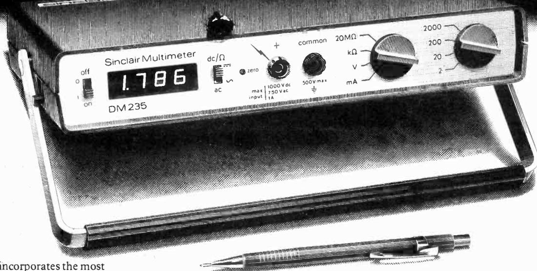
The DM235 incorporates the most important features of a bench-top meter into a rugged yet lightweight instrument for true portability. High accuracy, resolution and input impedance mean superior performance to analogue meters – but at a price significantly lower than many. The DM235's design and specification makes it ideal for all but the most demanding applications.
