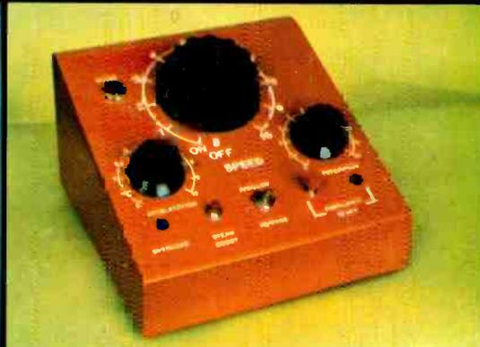
A pulse width train controller for smooth slow running plus inrush braking and acceleration. Full construction details in our catalogue.
