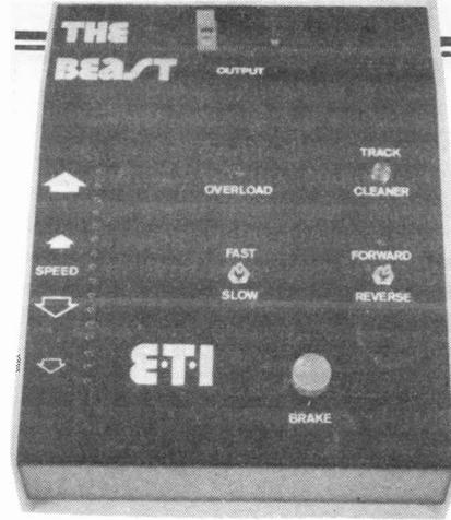
ensuring that the power signals are unimpaired by oxides and gunge on the track, pick-ups, and motor brushes. The track cleaner system can not be used with 2-wire controllers.
